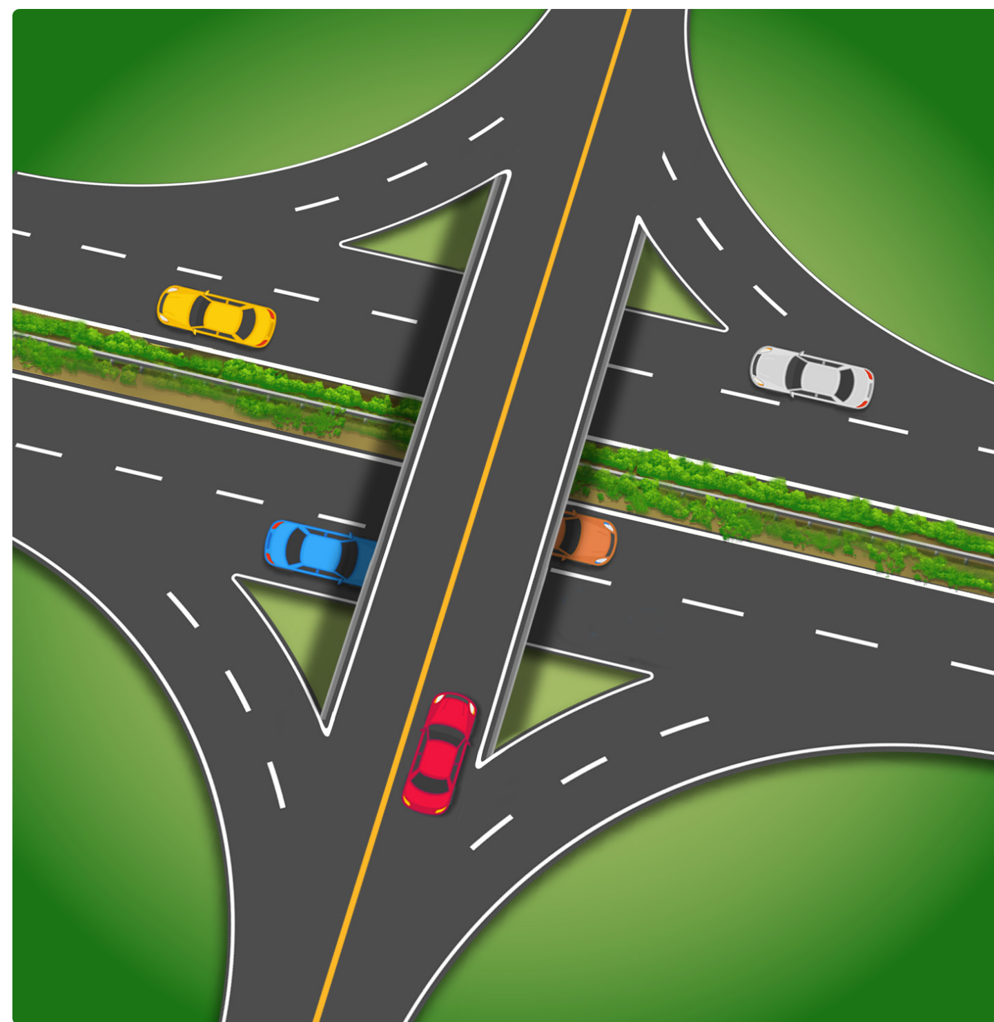
Interchange SR 316 traverses over or under the side road with entrance and exit ramps.
