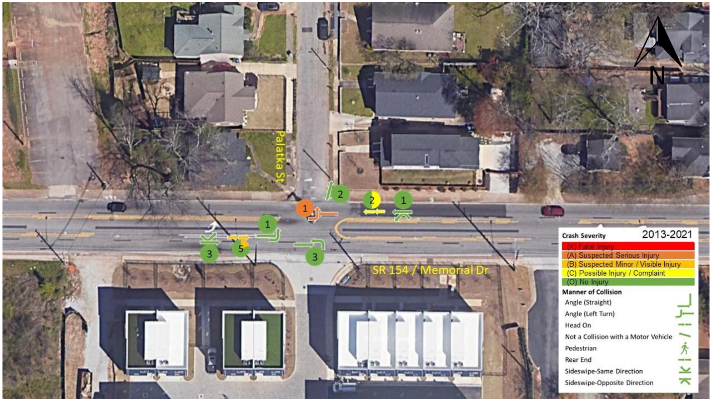
Figure 17 - Crash Diagram for SR 154 at Palatka St
