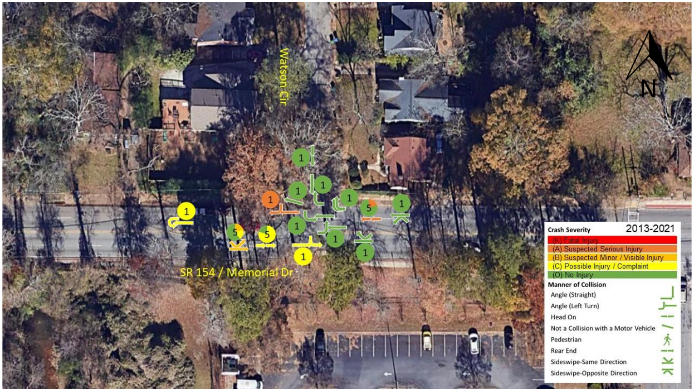
Figure 18 - Crash Diagram for SR 154 at Watson Cir
