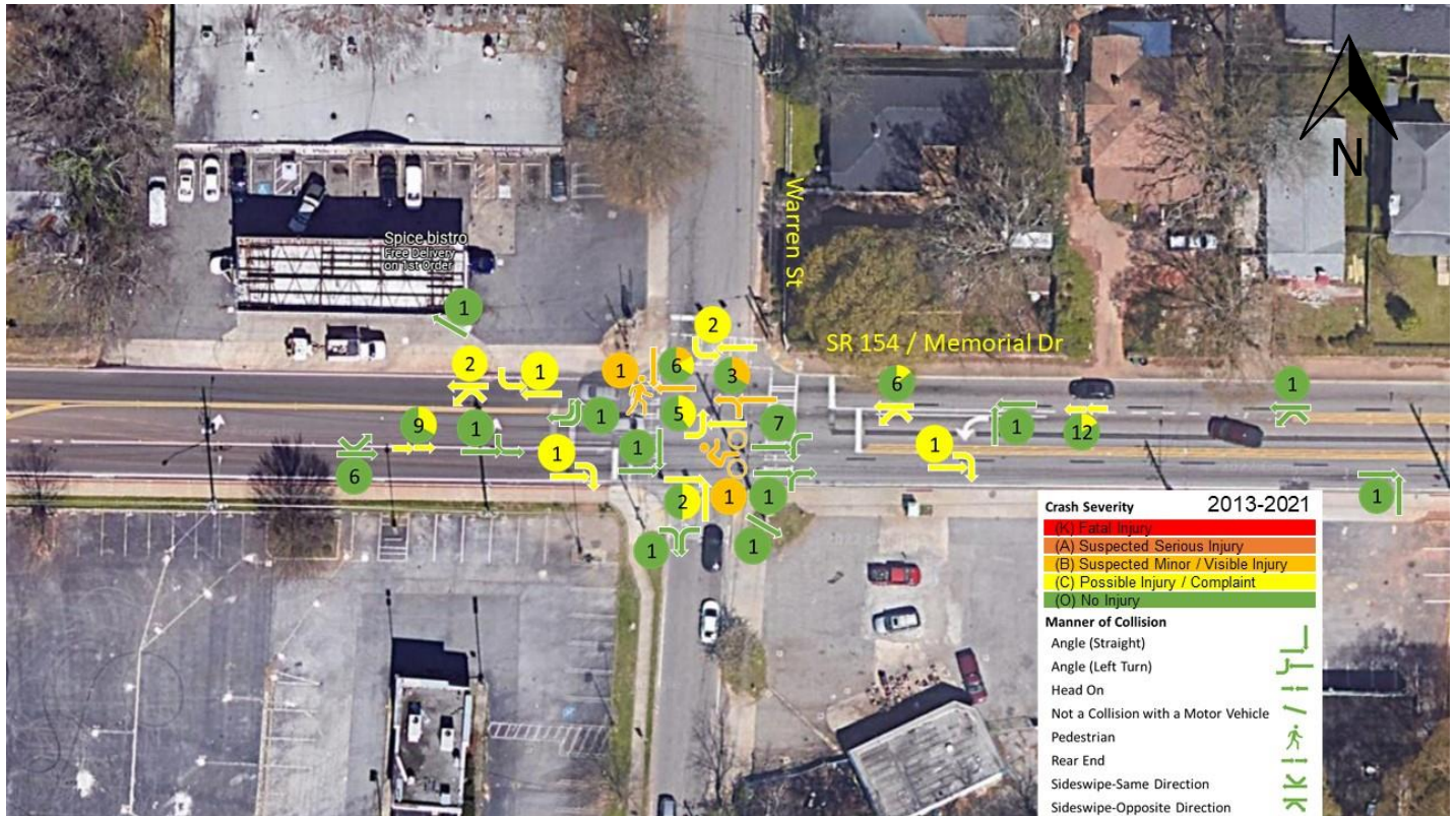
Figure 13 - Crash Diagram for SR 154 at Warren St
