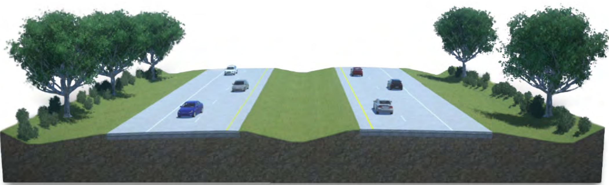
TYPICAL SECTION 1: FOUR-LANE RURAL FREEWAY WITH DEPRESSED MEDIAN SR 316
