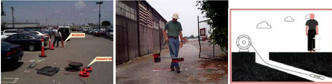
Metallic Pipe - Direct Connection and Surface Induction
