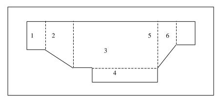
Each of the end areas of the area of excavation has different dimensions and are shown in the following table:
