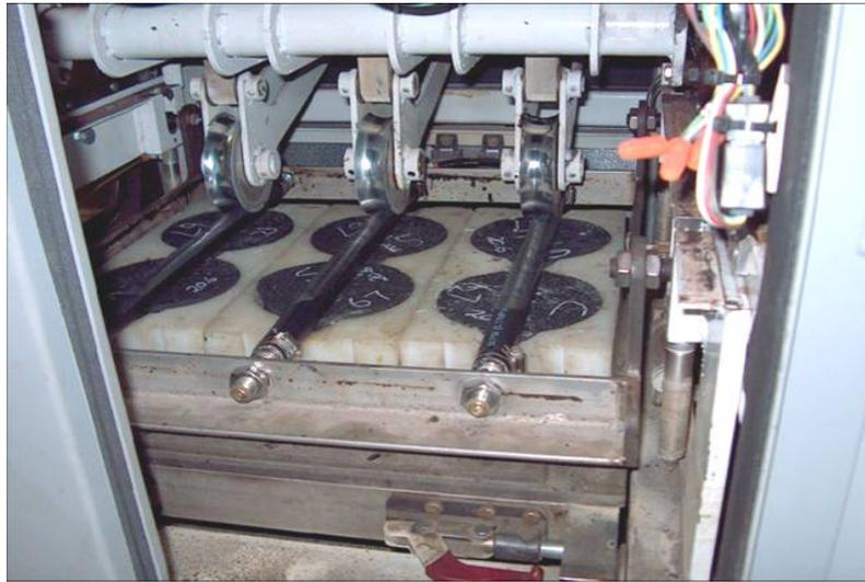
**The Asphalt Pavement Analyzer measures a mix design's resistance to rutting**
