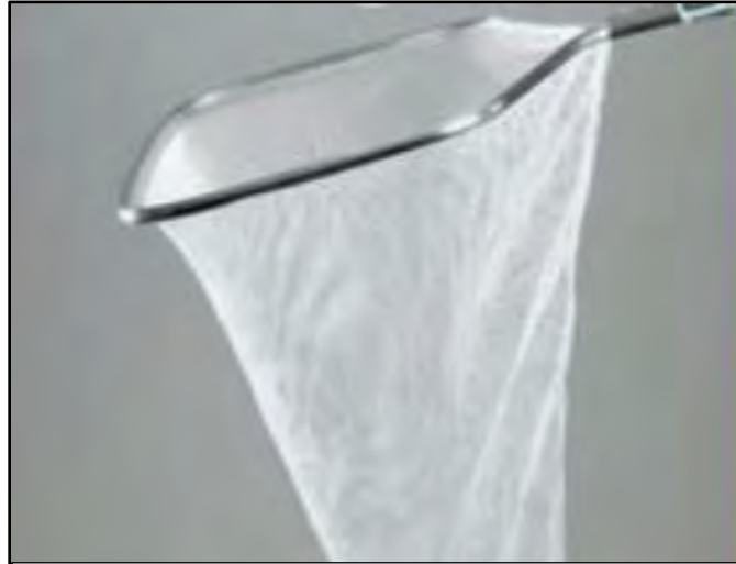
Image 6. Suggested dipnet product. Manufactured by Loki Nets—Stock # SH-2D: 16"x18" Monorail bow, D-shape (38cm width, interior dimension of frame), 48" aluminum handle, ace (nylon) netting, knotless; mesh size: 1/8" (4 mm); mesh depth: 18" or 24". (Thomas Floyd, GADNR Biologist)
