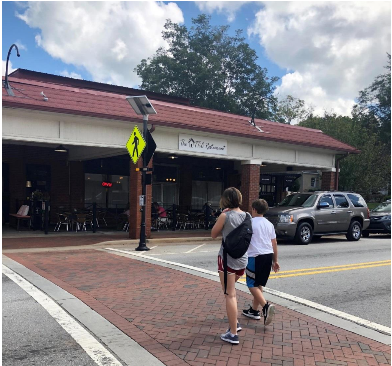
Figure 5.1. Rectangular Rapid Flashing Beacon
