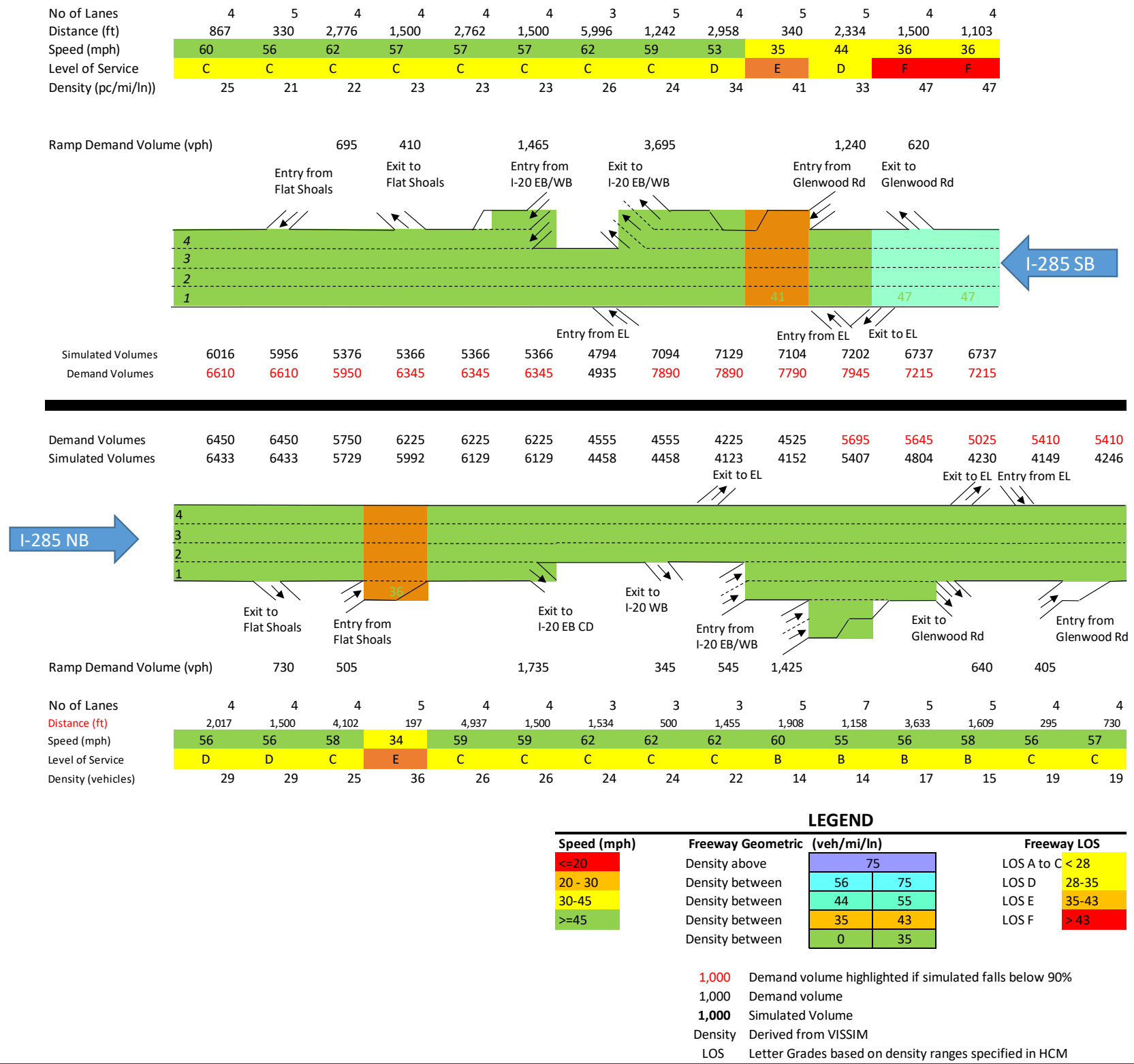
Figure 6-6. Freeway Segment Analysis Schematic Results (VISSIM) – 2045 Build AM Peak (I-285 SB & NB)
