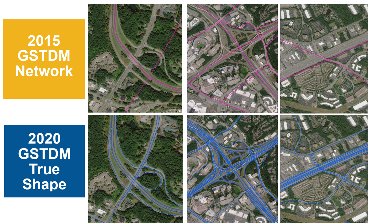
Figure 4 True Shape versus Previous Network Representation
