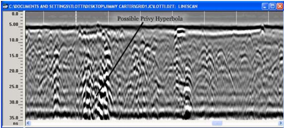
Figure 4. GPR linescan for Grid 1.
