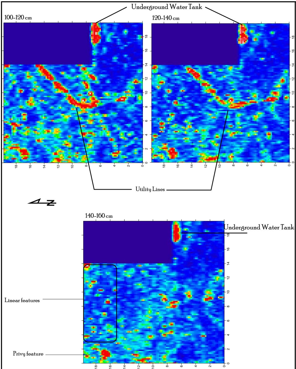
Figure 9. Super 3D composite radar image of Grids 1 and 2.
