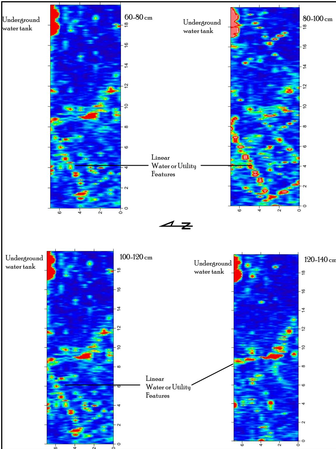
Figure 7. Composite radar image of Grid 2.
