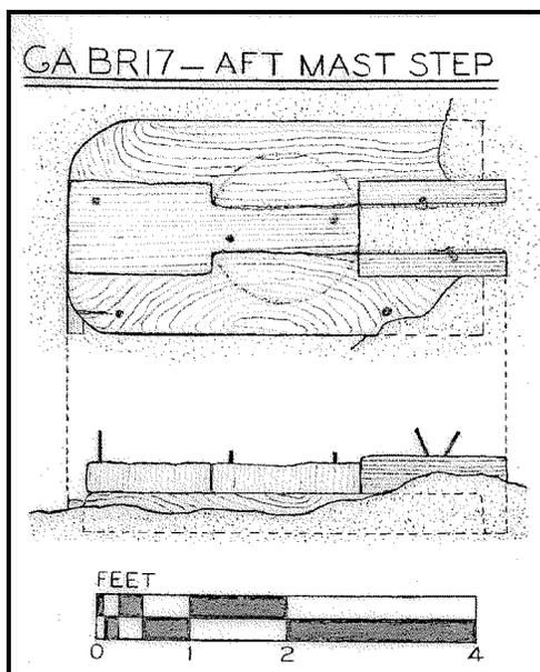
Figure 35. Drawing of the Mainmast step (USACE, Savannah 1994:164).
