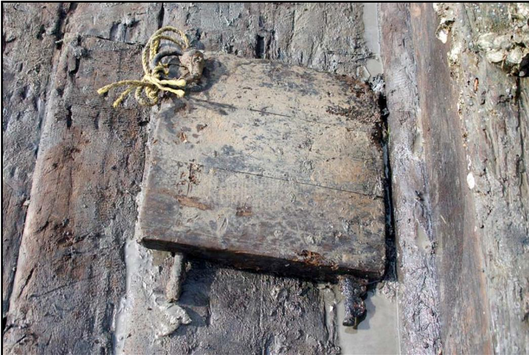
**Figure 66. Hatch for lumber port.**
