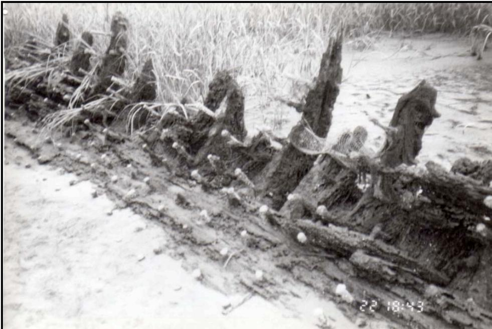
**Figure 37. Starboard side of the hull illustrating the futtock and fastener pattern (USACE, Savannah).**
