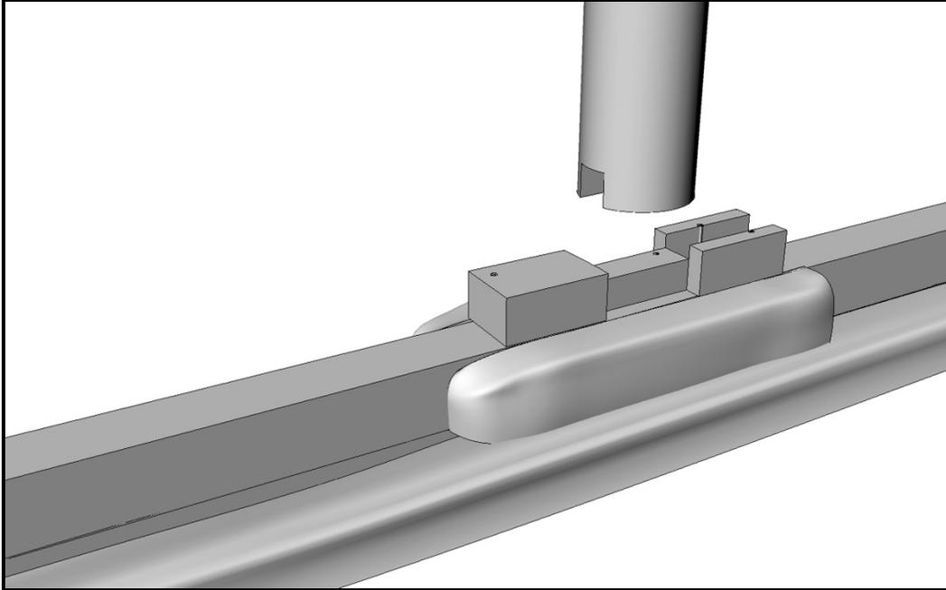
**Figure 65. Configuration of the mainmast step and heel of the mast.**
