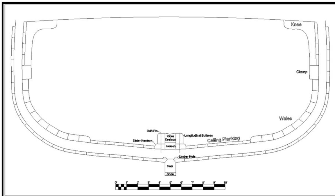
Figure 101. Hull section reconstruction at the mainmast step.
