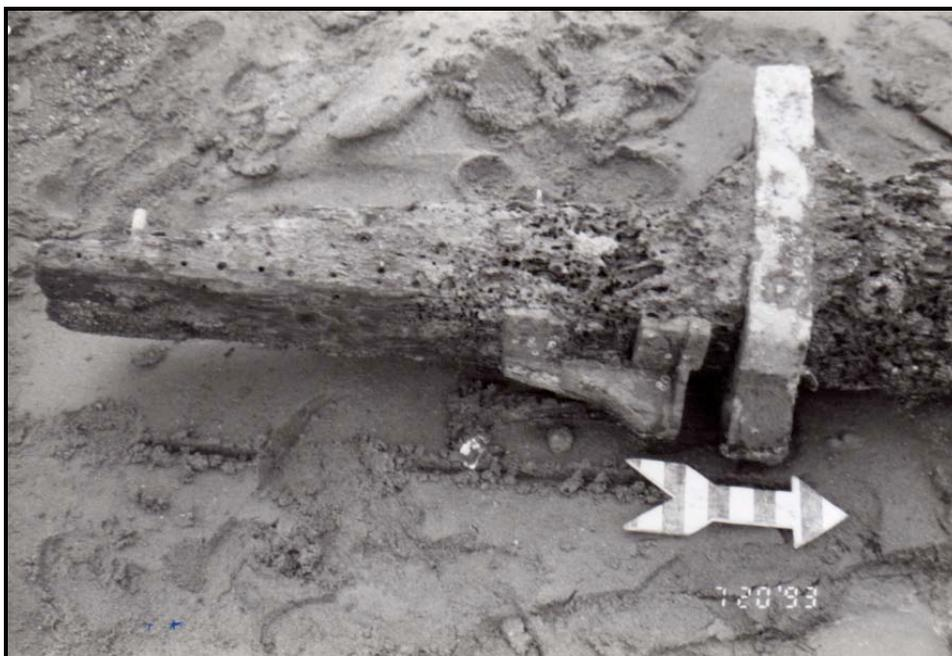
**Figure 39. Lower section of sternpost with gudgeon and pintle stop (USACE, Savannah).**
