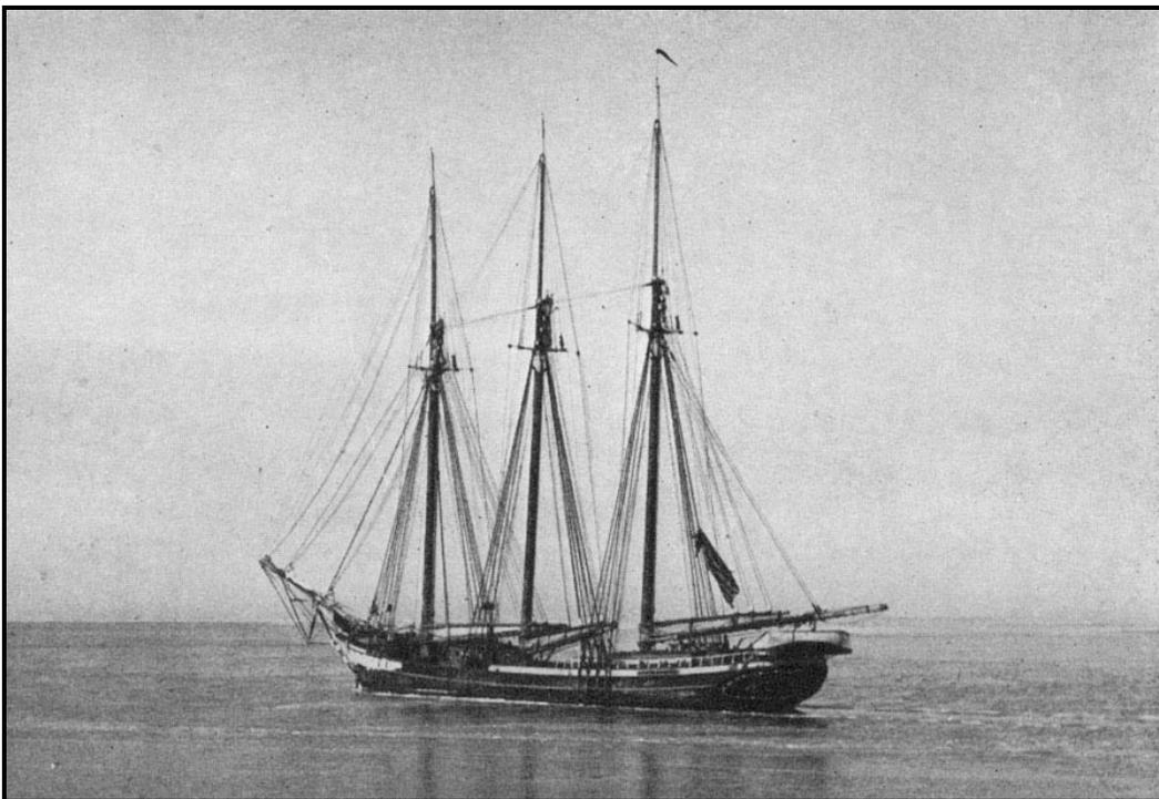
**Figure 105. Mast placement on the tern schooner Peter H. Crowell built at East Boston in 1873 (Robinson and Dow 1924:473).**
