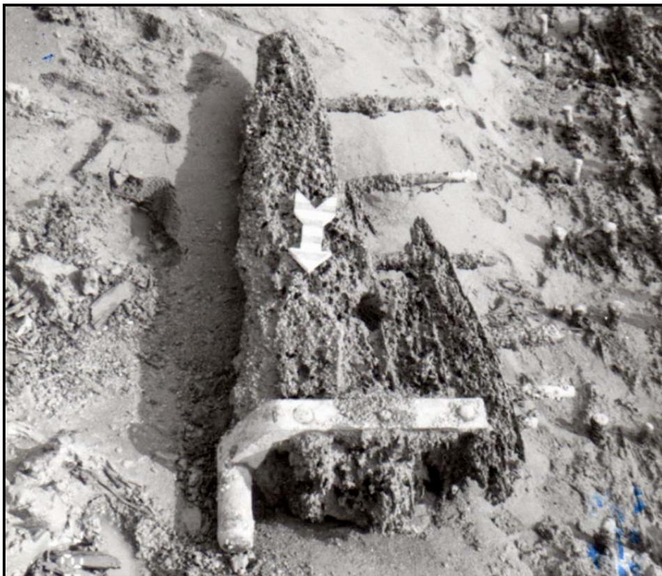
**Figure 40. Section of the rudder with pintle attached (USACE, Savannah).**
