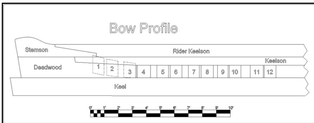
**Figure 57. Profile drawing of the surviving bow structure.**
