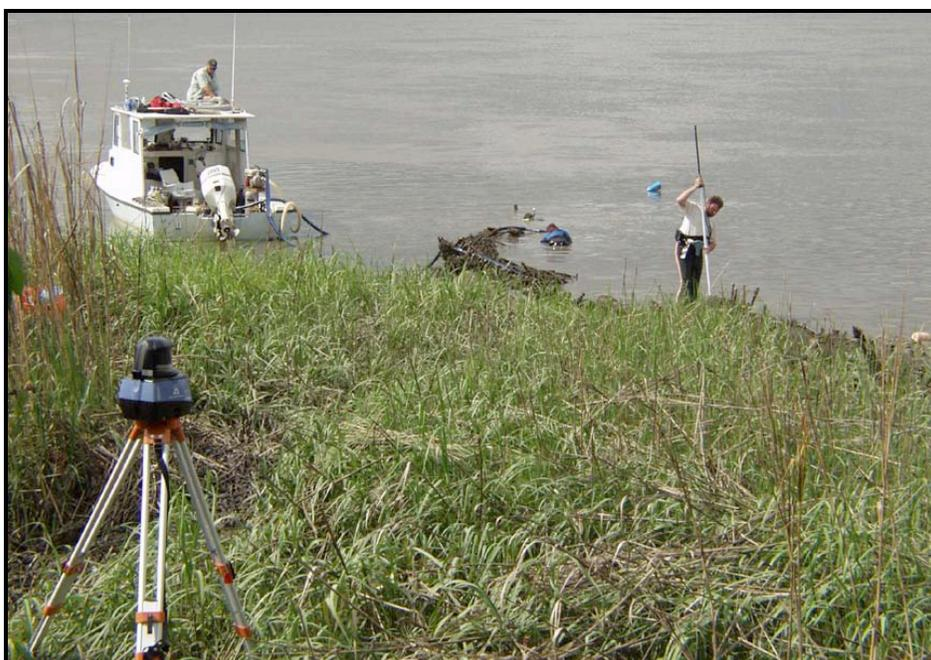
**Figure 44. One of two laser transmitters mounted on tripods in the marsh.**
