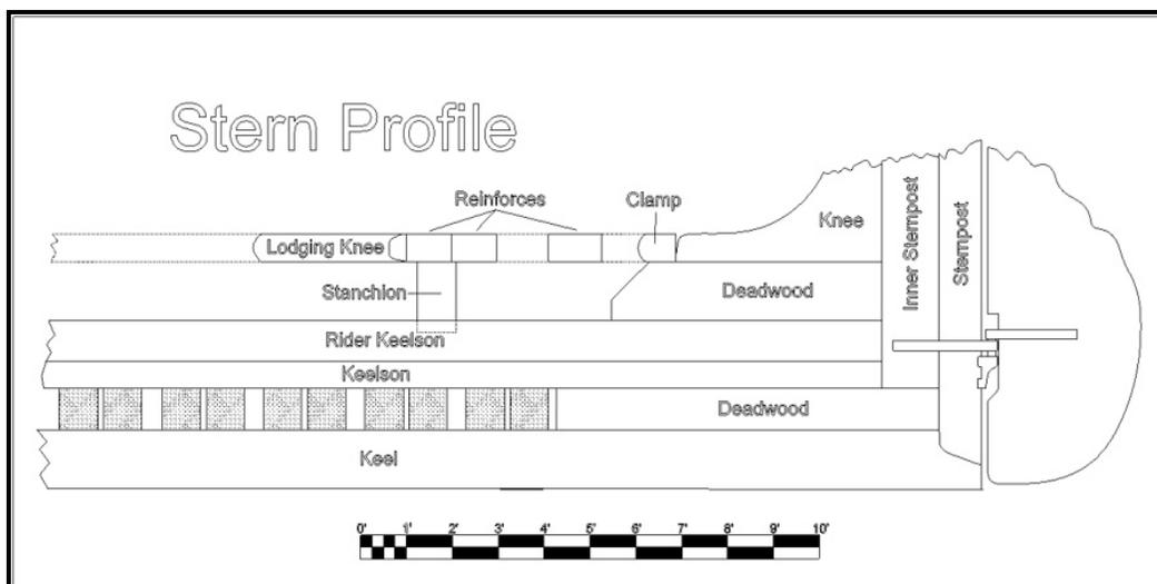
**Figure 59. Profile drawing of the surviving stern structure.**
