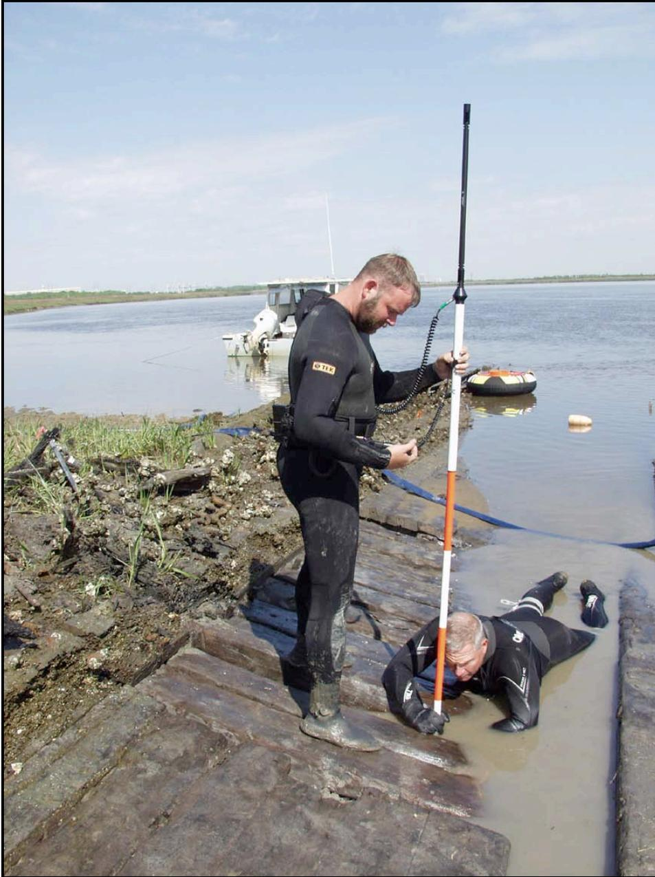
**Figure 49. Mapping molded dimensions and plank seams.**
