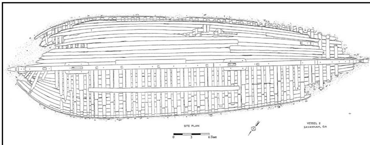
Figure 109. Plan of derelict vessel No. 2 excavated by Tidewater Atlantic Research, Inc., in 1993.
