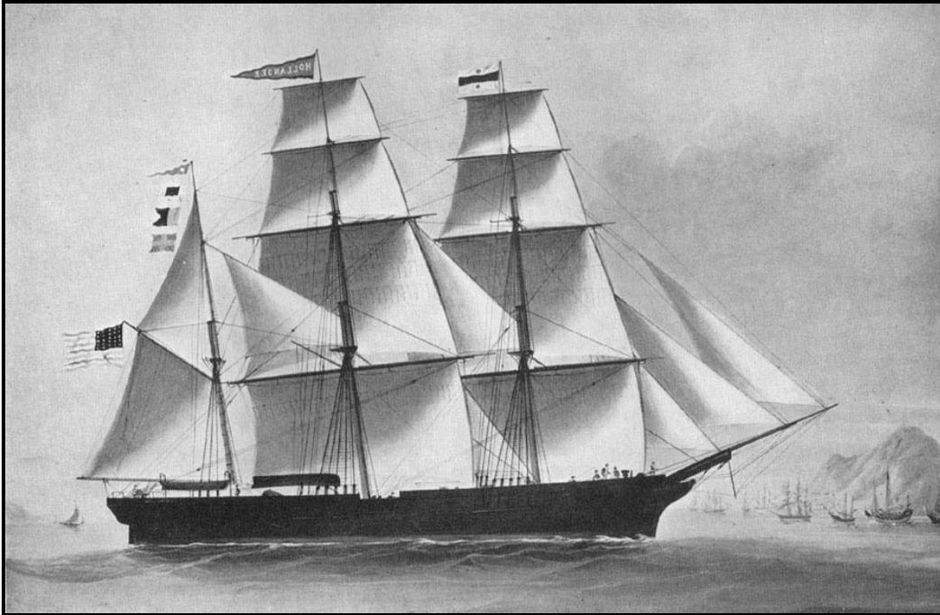
**Figure 103.** Mast placement on the bark *Hollander* built at Newburyport, Massachusetts in 1849 (Robinson and Dow 1924:405)
