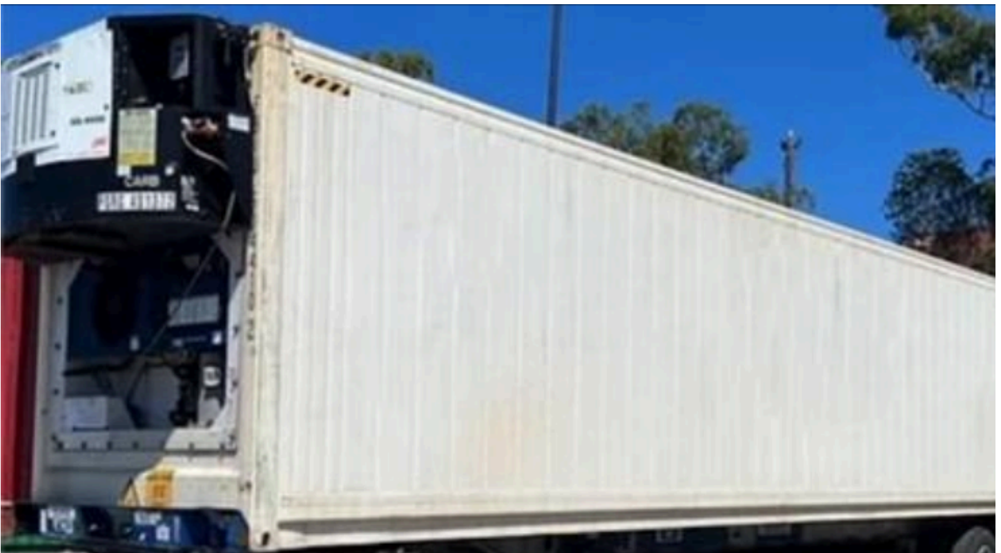
Type 111 Intermodal Freight Container secured to trailer chassis with genset (Photo courtesy of UL FSRI via the NIOSH report)
