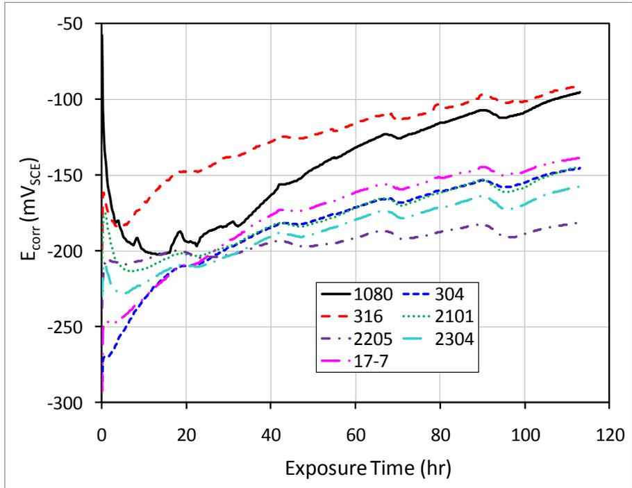
Figure 6.2  $E_{\text{corr}}$  vs. time in carbonated solutions
