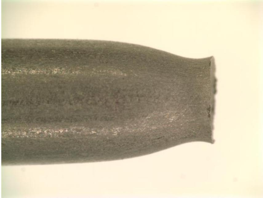
Figure C.13 Fracture surface of 17-7 HSSS
