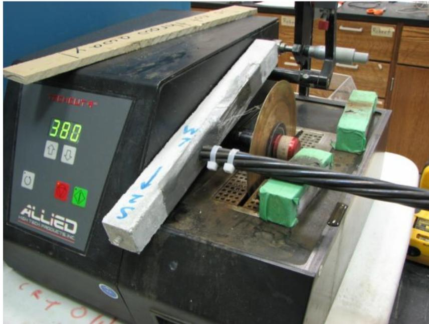
Figure E.1 Strand segments cut using slow-speed water-cooled diamond saw. Two plastic wire ties are secured around the seven-wire strand to prevent relative movement of the wires from their as-received geometry.
