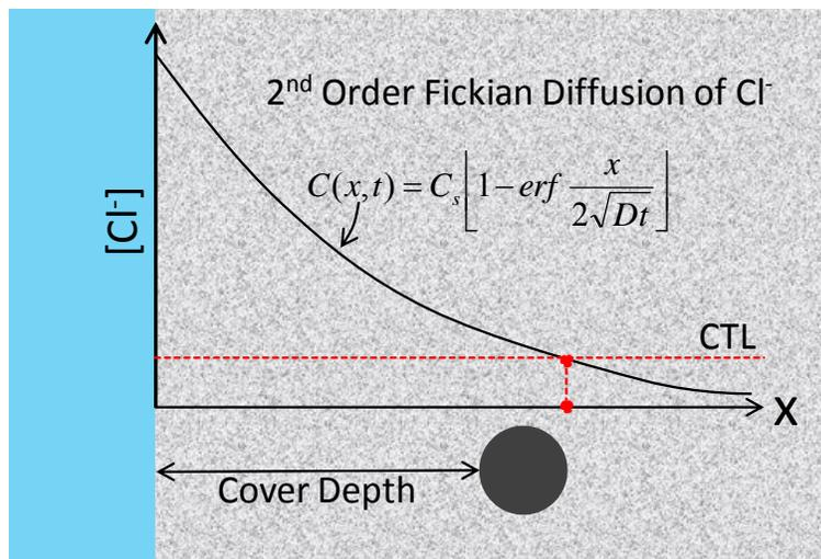
Figure 2.11 Colleparidi model for  $\text{Cl}^-$  ingress into concrete
