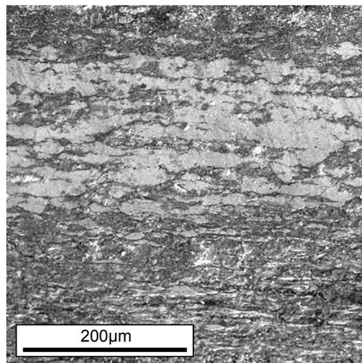
Figure 3.2 As-received  $ZnPO_4$  surface coating on prestressing steel
