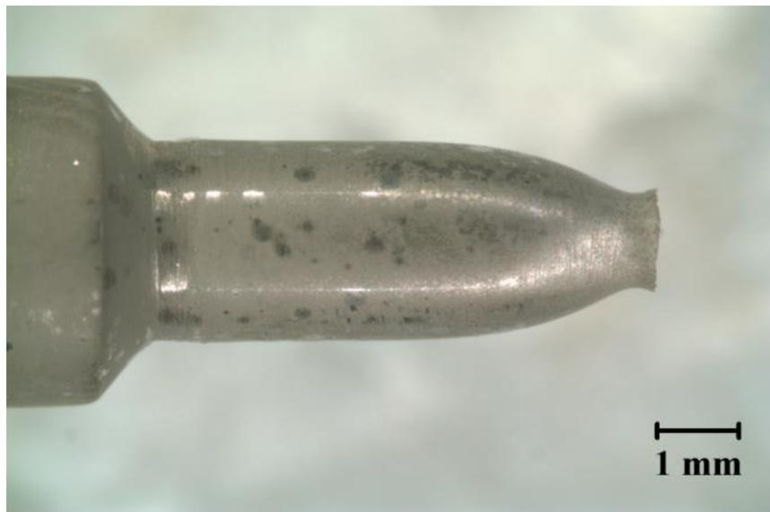
Figure I.2 2205 SSRT specimen tested in an alkaline solution with 0.5 M Cl<sup>-</sup>
