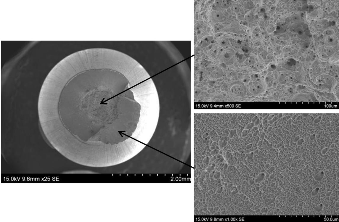
(b) Typical HSS fracture surface (2205 shown)
