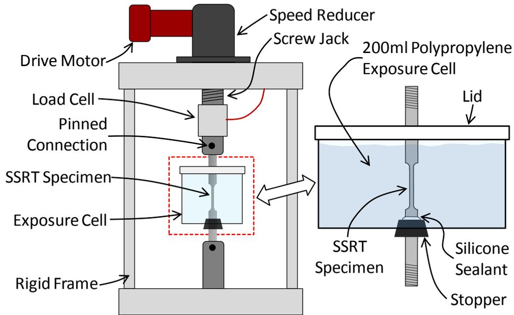
Figure 6.39 Apparatus and exposure cell used for SSRTs
