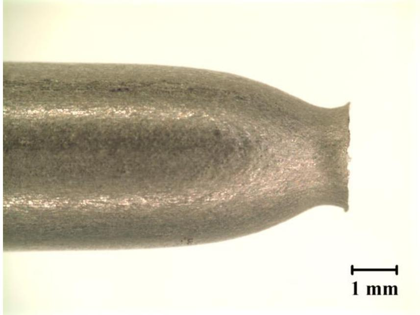
Figure C.3 Fracture surface of 304 HSSS
