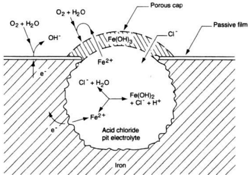
Figure 2.9 Typical corrosion pit morphology (Jones, 1996)
