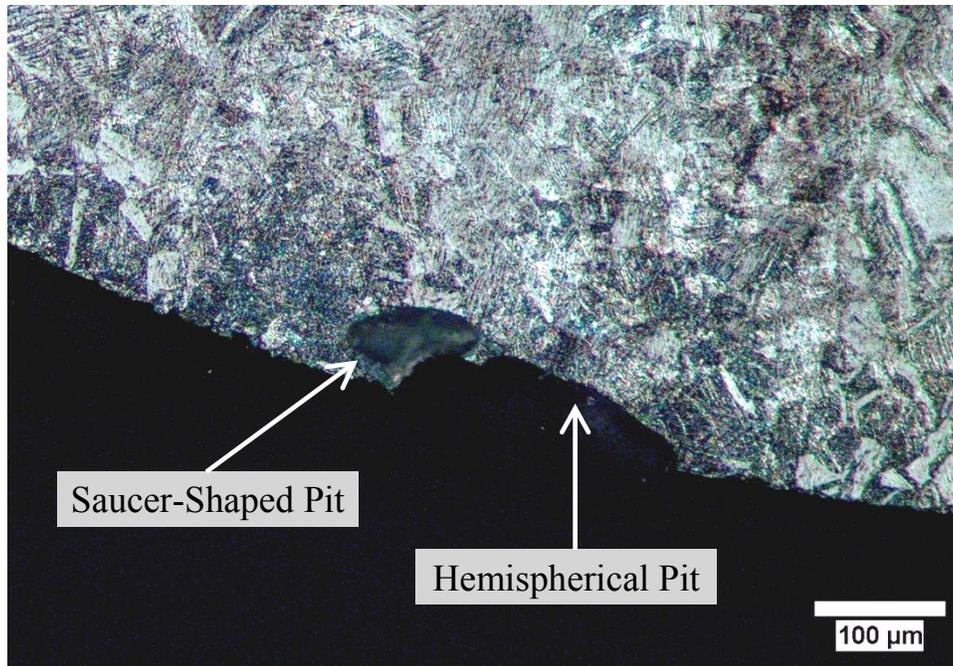
Figure 6.19 Hemispherical and saucer-shaped pitting of 304 HSSS
