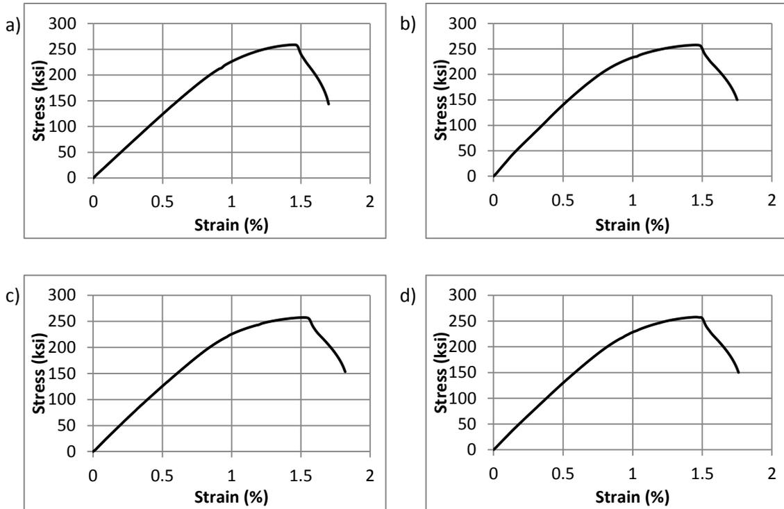
Figure J.7 2205 #7 HW wire stress-strain curves for a) test 1, b) test 2, c) test 3, and d) average
