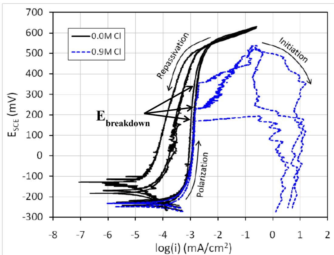
Figure 3.7 Cyclic polarization behavior of triplicate wire specimens under 0.0M and 0.9M Cl<sup>-</sup> exposure
