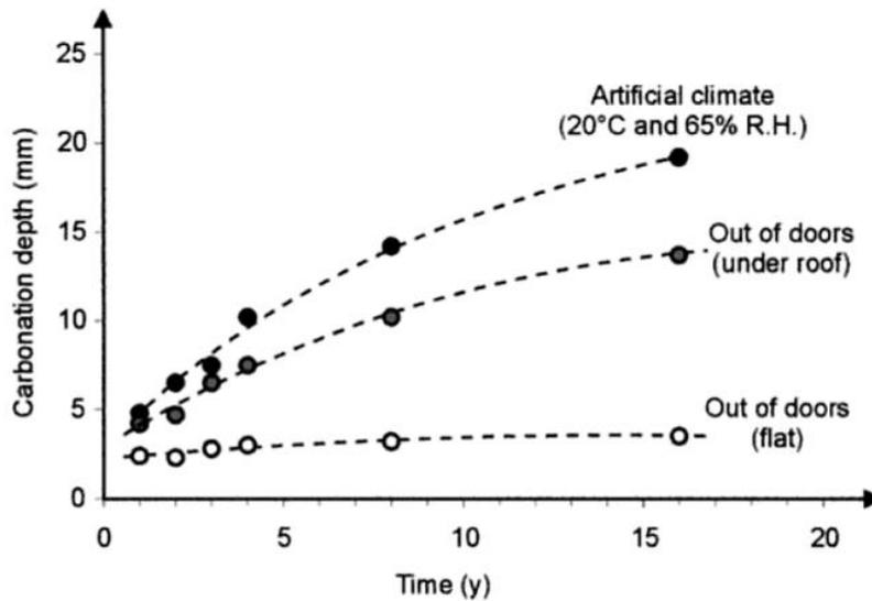
Figure 2.7 Carbonation depth vs. time (Wierig, 1984)
