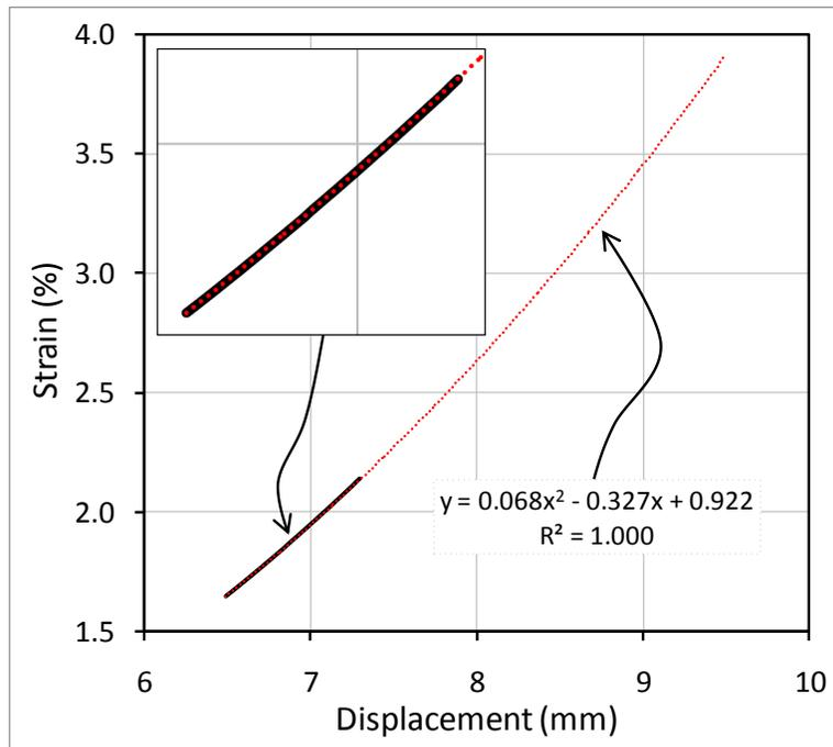
Figure 5.2 Crosshead displacement vs. strain calibration of 304 HSSS
