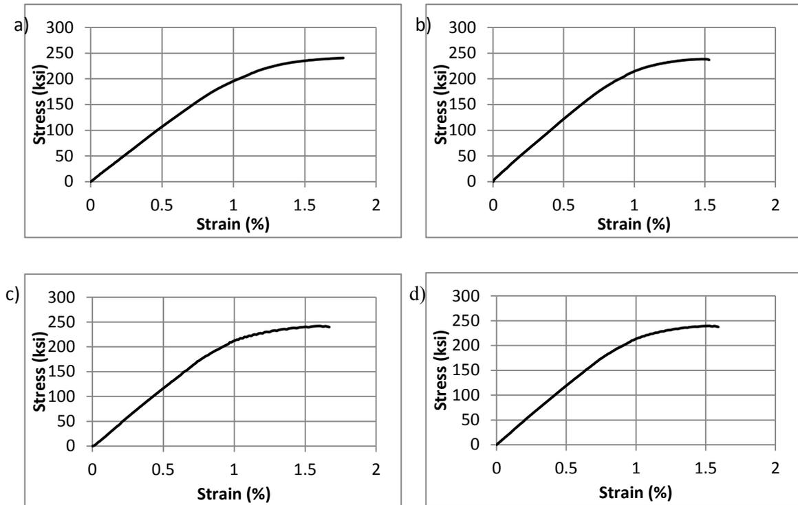
Figure J.1 2205 strand stress-strain curves for a) test 1, b) test 2, c) test 3, and d) average
