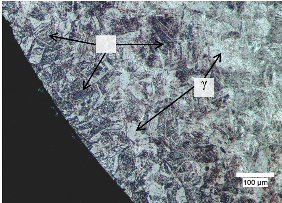
Figure 4. Increased density of  $\gamma$ -martensite at surface of 304 HSSS
