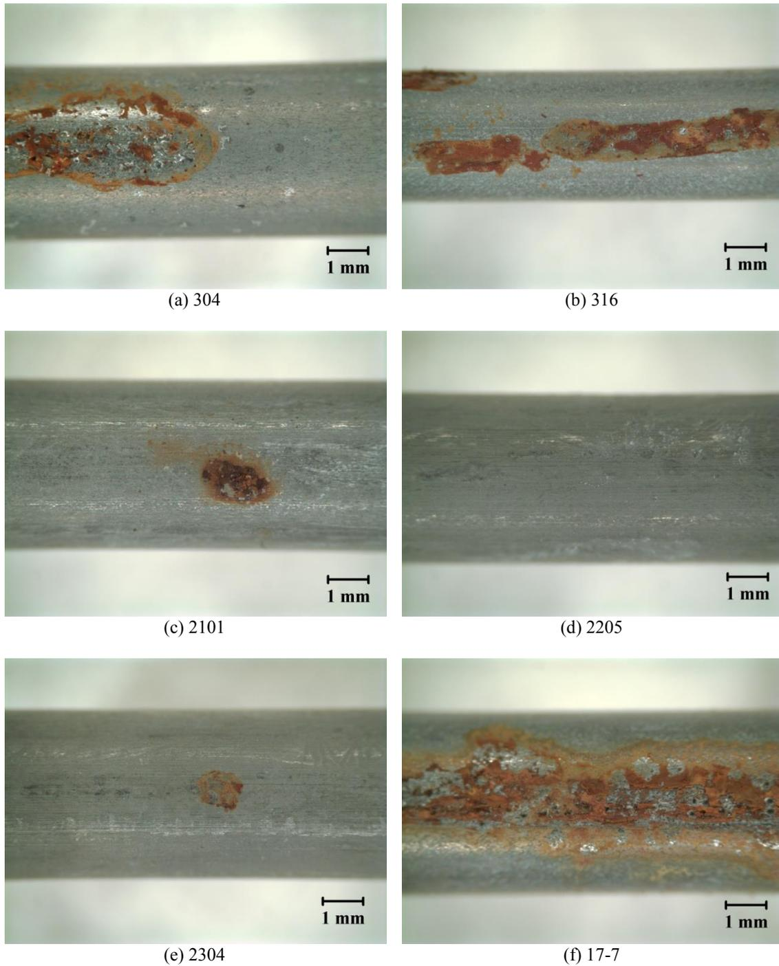
Figure 6.7 Corrosion damage in alkaline solutions with 1.00 M  $\text{Cl}^-$
