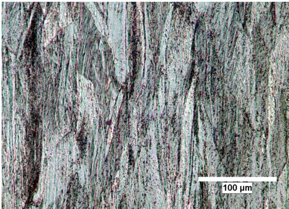
Figure B.6 Longitudinal microstructure of 304 HSS
