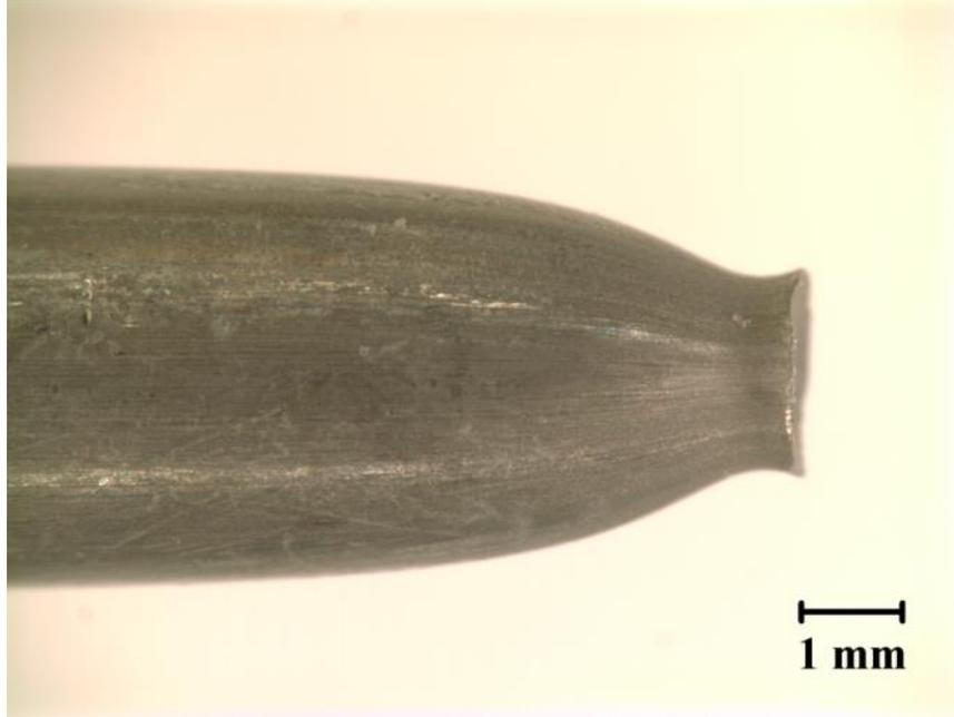
Figure C.11 Fracture surface of 2304 HSSS
