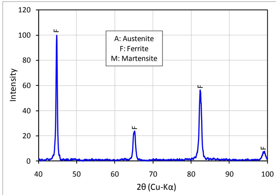
Figure 4.5 Diffraction pattern of High-C 1080 steel
