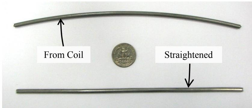
Figure 7.11 Stainless steel wire before and after straightening
