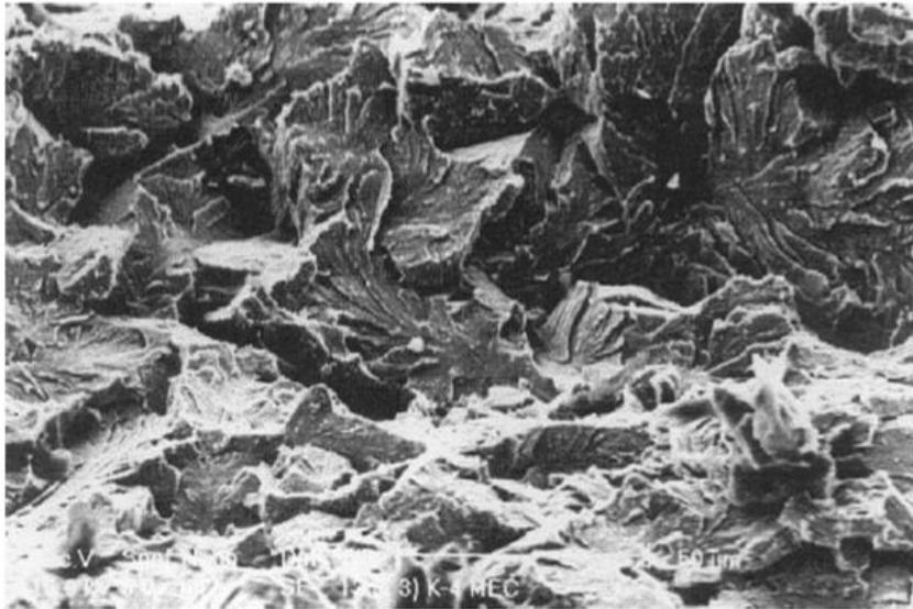
Figure 2.25 Transgranular HE of prestressing steel (from (Schroeder and Müller, 2003))
