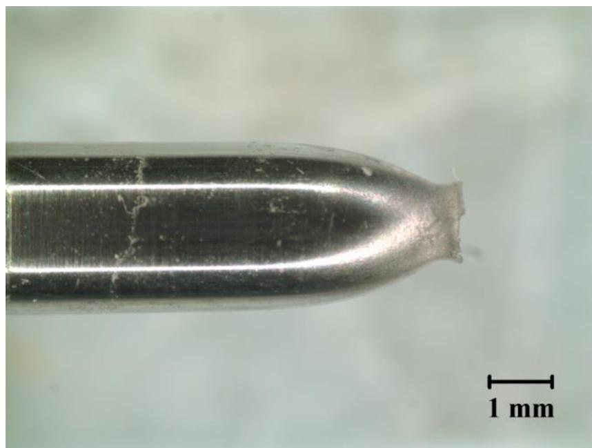
Figure I.3 2205 SSRT specimen tested in a carbonated solution with 0.5 M Cl<sup>-</sup>
