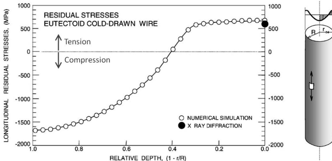
Figure 5.4 Residual stresses in 1080 prestressing steel (from (Elices, 2004))
