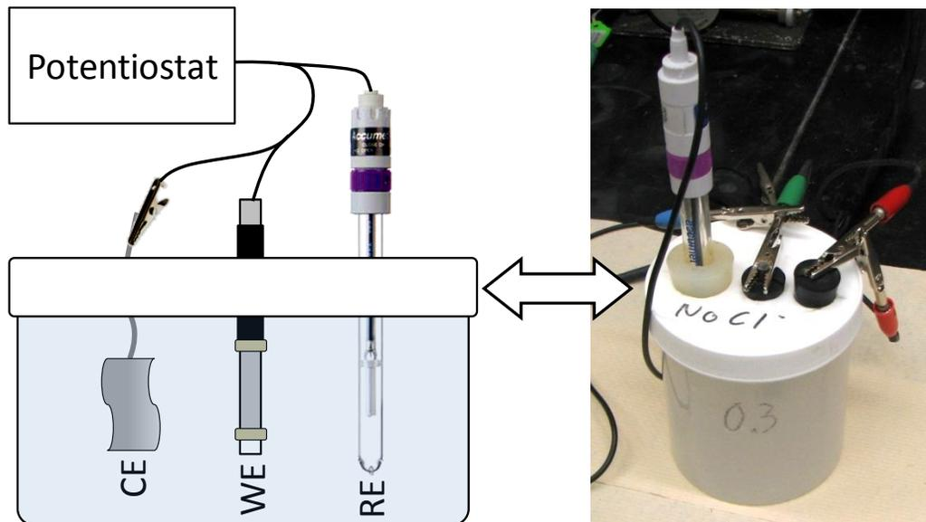
Figure 3.5 Three electrode electrochemical cell used for CPP experiments where CE is the cathode electrode, WE is the working (test wire) electrode, and RE is the reference electrode
