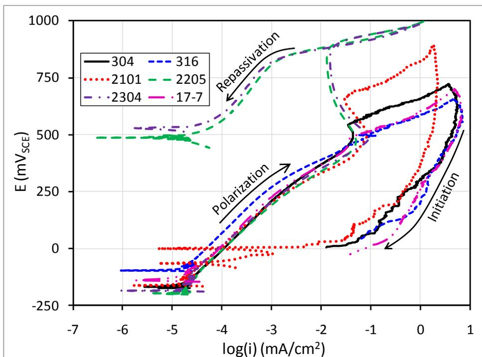
Figure 6.10 Polarization curves in carbonated solutions with 0.50 M Cl<sup>-</sup>
