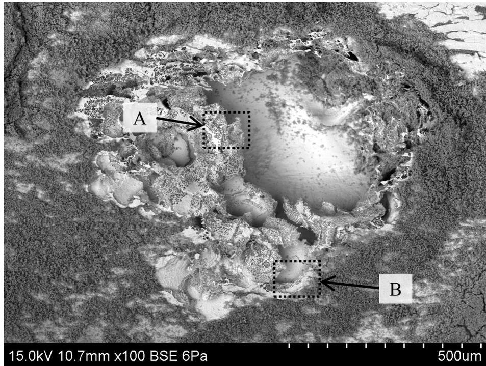
Figure 6.15 Large pit in 304 HSS tested in a carbonated solution with 1 M Cl<sup>-</sup>
