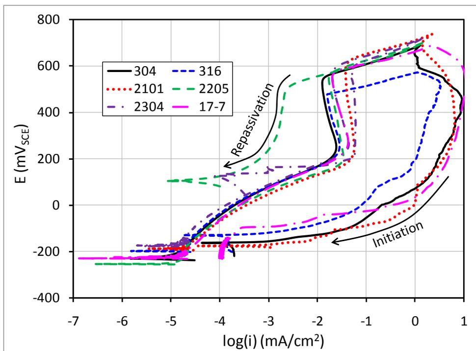
Figure 6.6 Polarization curves in alkaline solutions with 1.00 M Cl<sup>-</sup>
