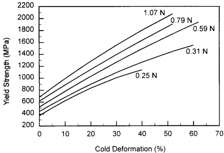
Figure 2.33 Influence of N addition and cold deformation on yield strength (from (Stein and Witulski, 1990))
