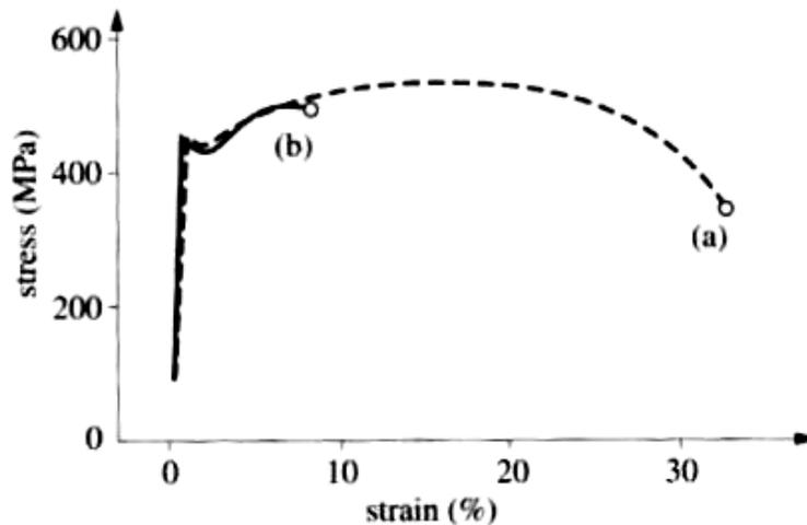
Figure 2.19 Slow strain rate test of steel in (a) air and (b) seawater (from (Landolt, 2007))
