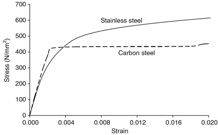
Figure 2.35 Comparison between the stress vs. strain behavior of stainless steel and carbon steel (from (Gardner, 2005))
