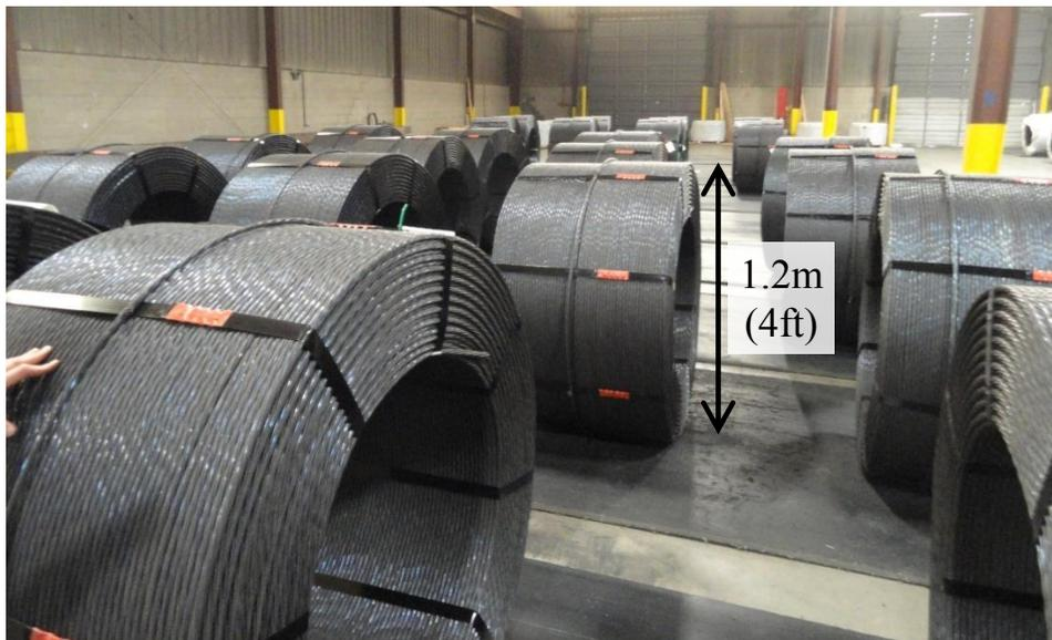
Figure 7.6 Packs of prestressing strand ready for shipment at RettCo Steel
