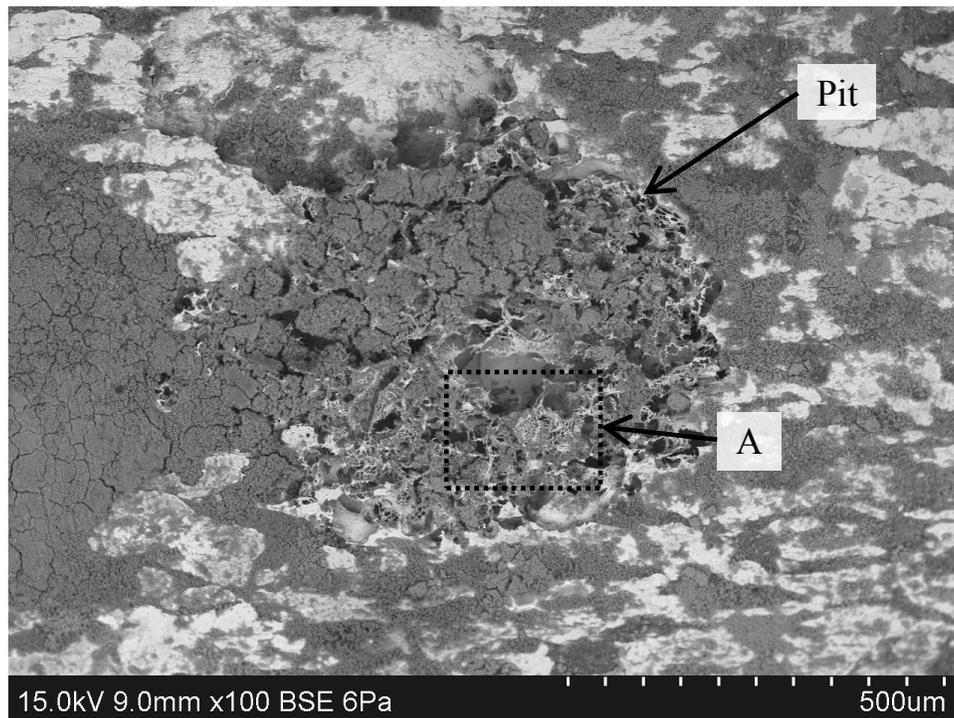
Figure 6.28 Corrosion pit in 17-7 HSSS tested in carbonated solution with 1 M Cl<sup>-</sup>
