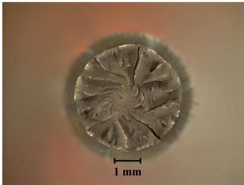
Figure C.2 Fracture surface of 1080 prestressing steel
