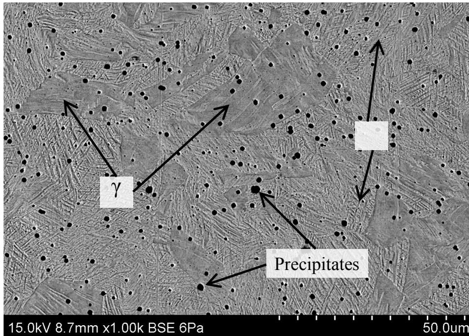
Figure 4.8 SEM micrograph of etched 316 showing distributed precipitates
