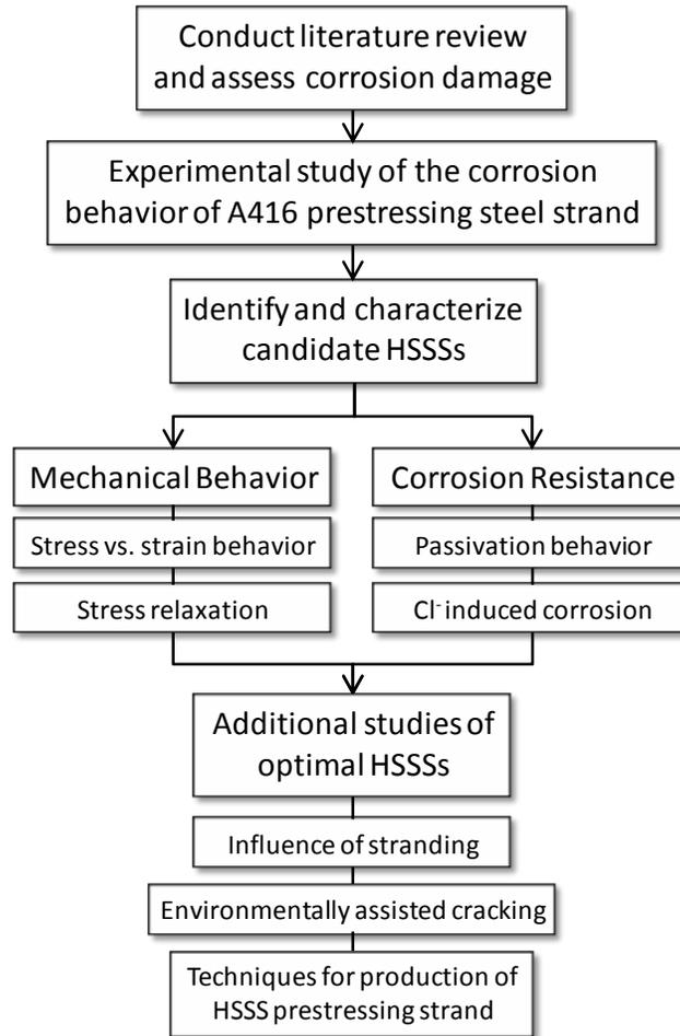
Figure 1.1 Scope of experimental program
