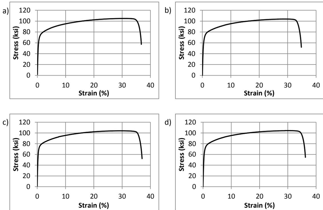
Figure J.8 2304 rod stress-strain curves for a) test 1, b) test 2, c) test 3, and d) average
