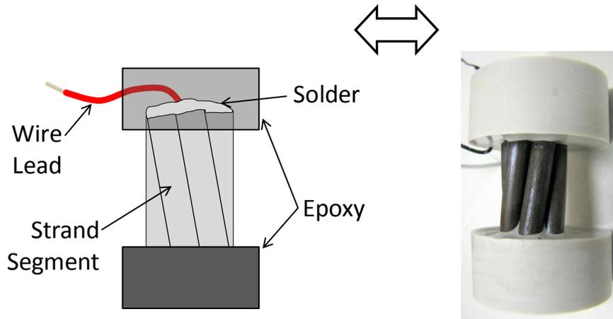
Figure 3.4 Overview of prestressing strand specimen configuration
