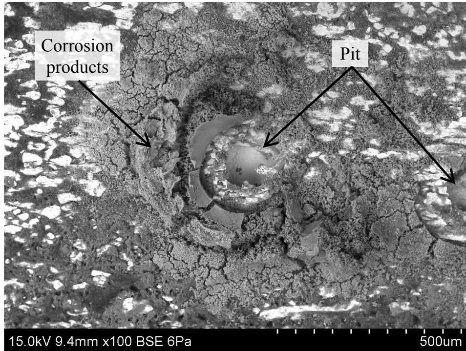
Figure 6.14 Large corrosion pit in 316 HSS tested in an alkaline solution with 0.5M Cl<sup>-</sup>
