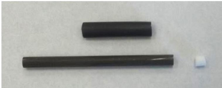
Figure D.2 Cut wire specimen along with heat-shrink tubing and PTFE plug to be epoxied to the end of the wire segment
