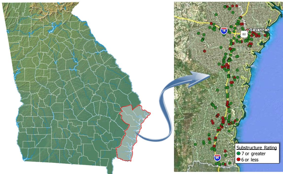
Figure 1.3 Bridge substructure deterioration in Georgia's coastal counties
