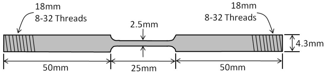
Figure 6.38 Dogbone specimen used for all SSRTs
