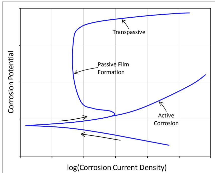
Figure 2.3 Polarization curve for active and passive metal
