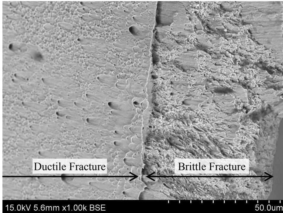
Figure 6.48 Fracture surface of 2205 HE SSRT specimen in carbonated solution corresponding to region A in Figure 6.47
