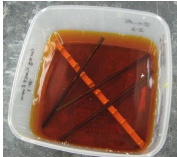
(b) Wire segments with  $\text{FeCl}_3$  solution added to exposure cell
