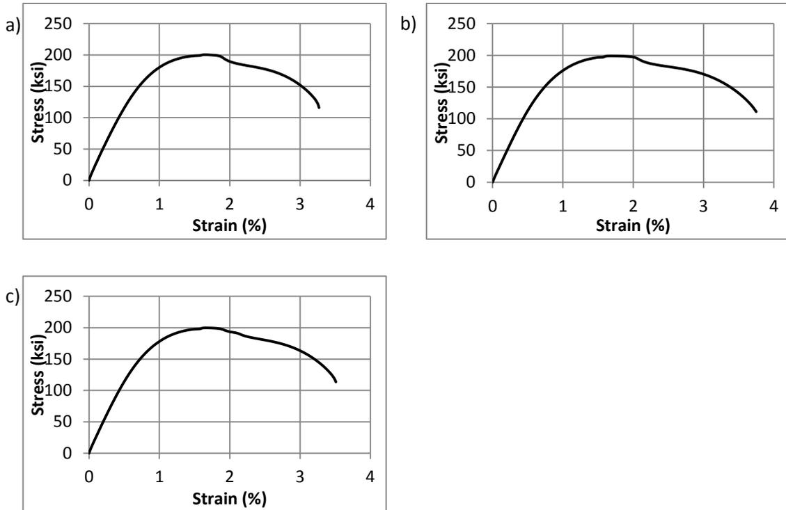
Figure J.9 2304 #3 wire stress-strain curves for a) test 1, b) test 2, c) test 3, and d) average
