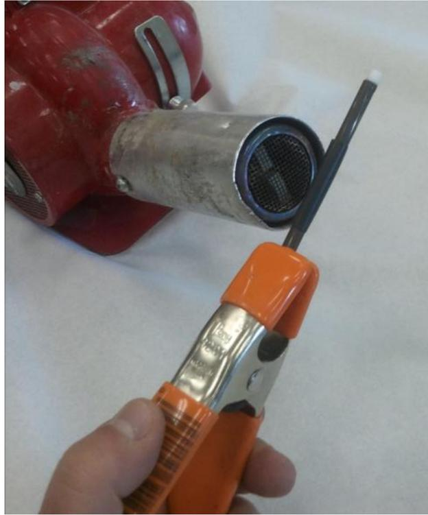
Figure D.3 Securing heat shrink tubing to wire segment with heat gun
