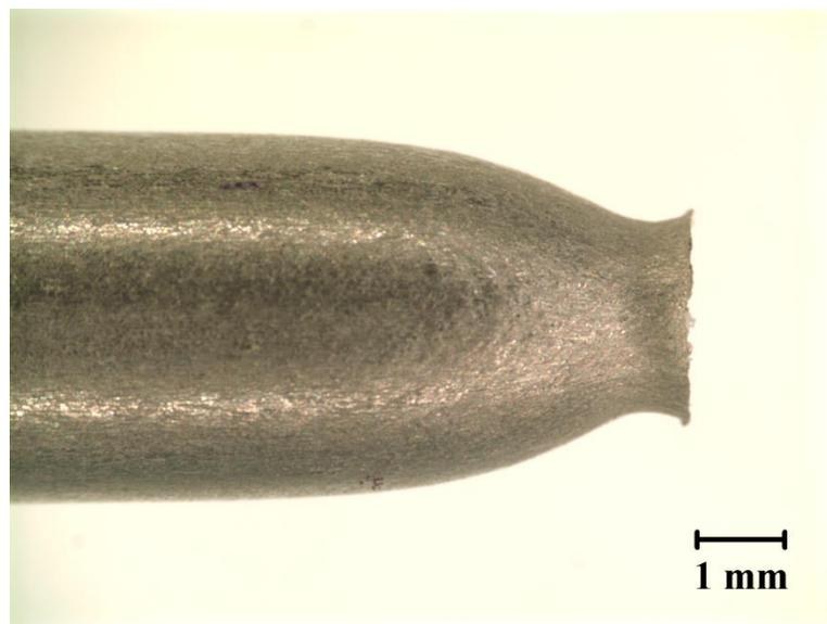
(b) Typical HSS fracture surface (304 shown)
