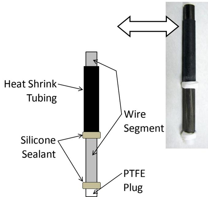
Figure 3.3 Overview of prestressing wire specimen configuration
