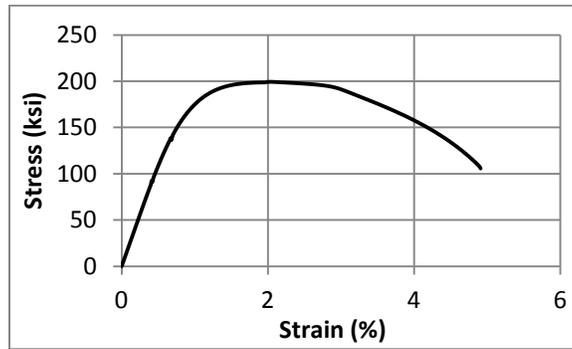
Figure J.5 2205 #5 wire stress-strain curve
