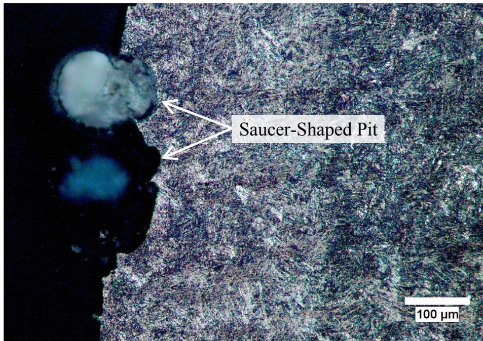
Figure 6.30 Cross section of pit in 17-7 HSS tested in alkaline solution with 0.5 M  $\text{Cl}^-$
