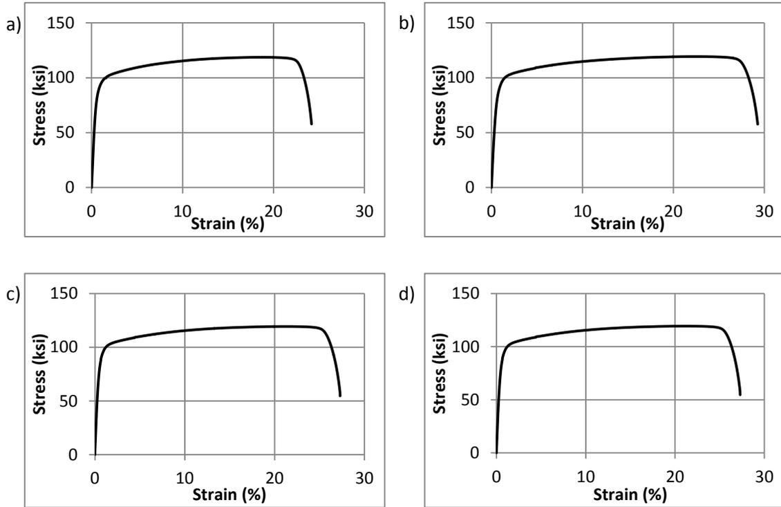
Figure J.3 2205 rod stress-strain curves for a) test 1, b) test 2, c) test 3, and d) average
