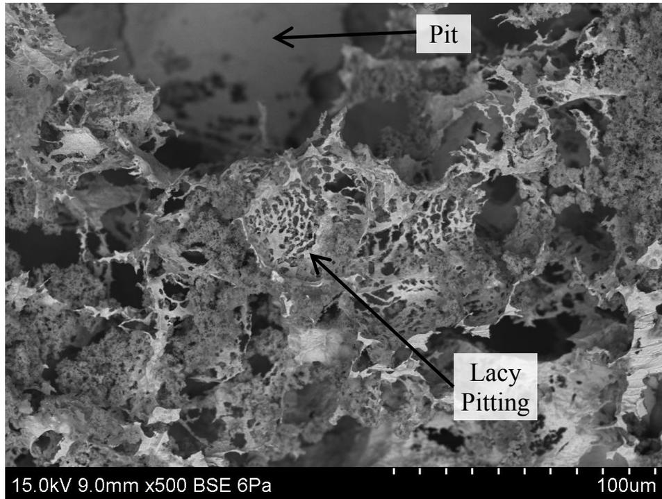
Figure 6.29 Lacy pitting in region A of the corrosion pit shown in Figure 6.28
