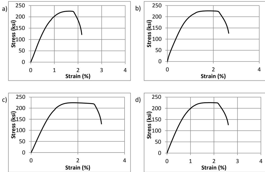
Figure J.6 2205 #7 UW wire stress-strain curves for a) test 1, b) test 2, c) test 3, and d) average
