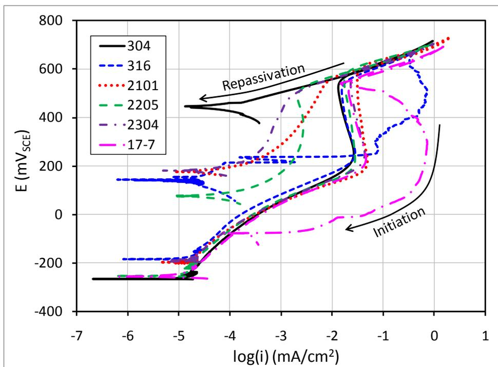
Figure 6.4 Polarization curves in alkaline solutions with 0.25 M Cl<sup>-</sup>
