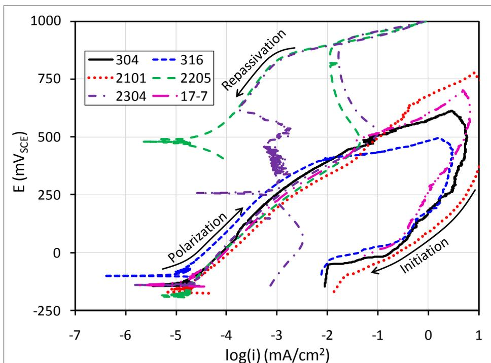
Figure 6.11 Polarization curves in carbonated solutions with 1.00 M Cl<sup>-</sup>
