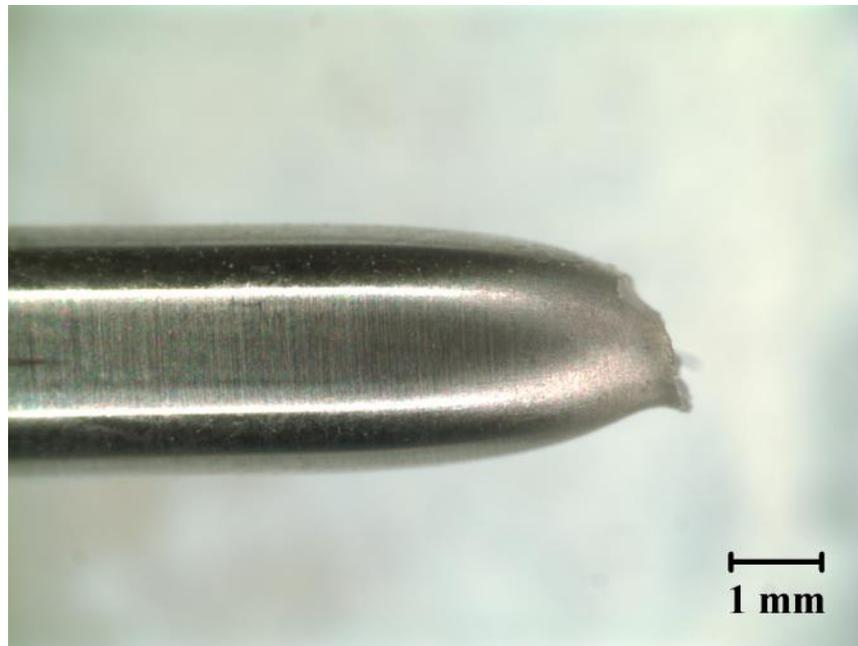
Figure I.6 2304 SSRT specimen tested in air
