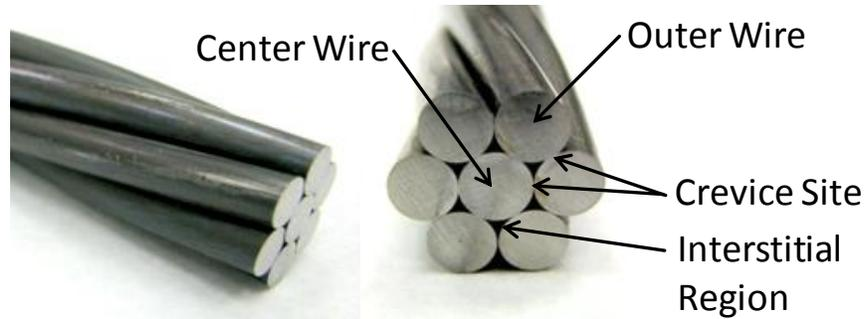
Figure 2.10 Seven-wire prestressing strand geometry including crevice sites
