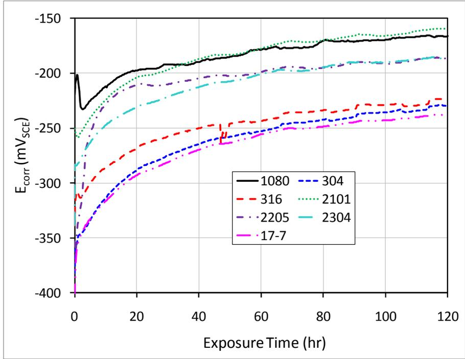
Figure 6.1  $E_{\text{corr}}$  vs. time in alkaline solutions
