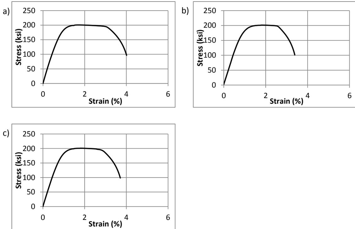
Figure J.4 2205 #3 wire stress-strain curves for a) test 1, b) test 2, and c) average
