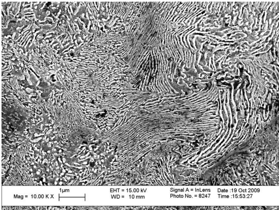
Figure B.4 Transverse microstructure of 1080 prestressing steel
