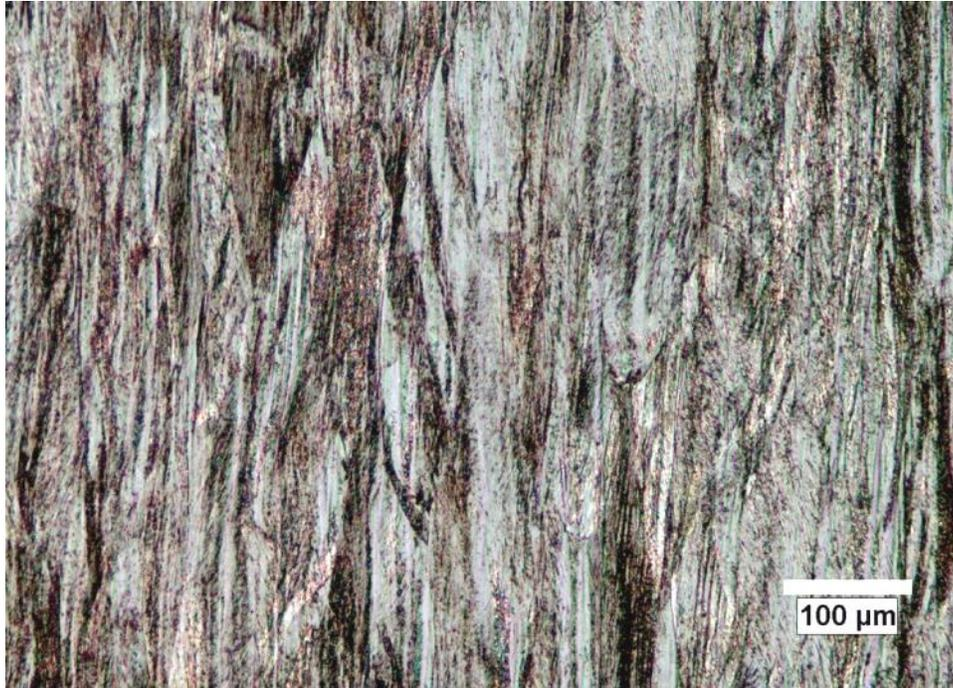
Figure B.5 Longitudinal microstructure of 304 HSS
