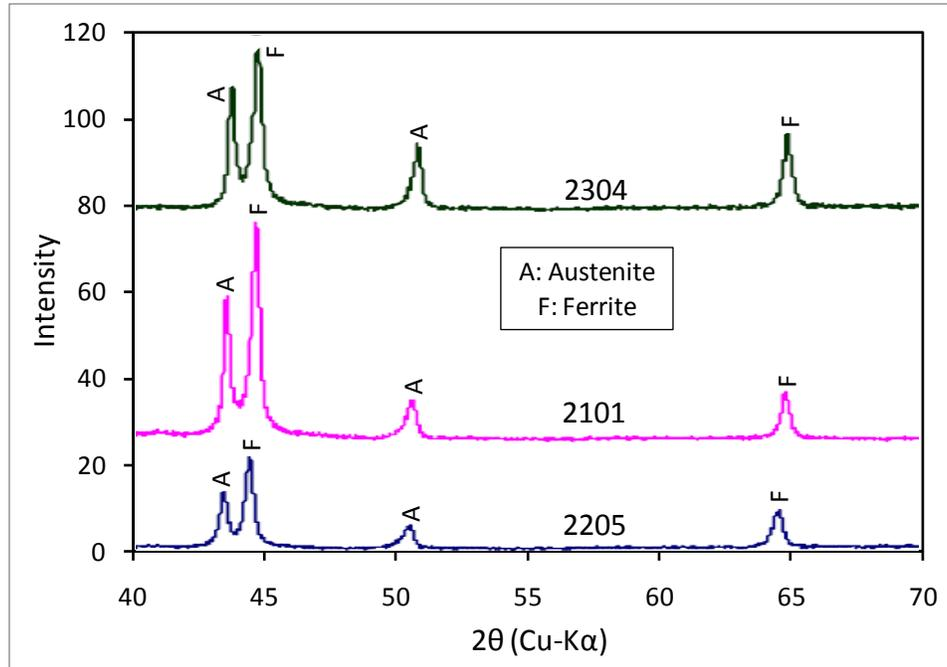
Figure 4.12 XRD patterns of annealed 2101, 2205, and 2304 (from (Bhattacharya, 2008))
