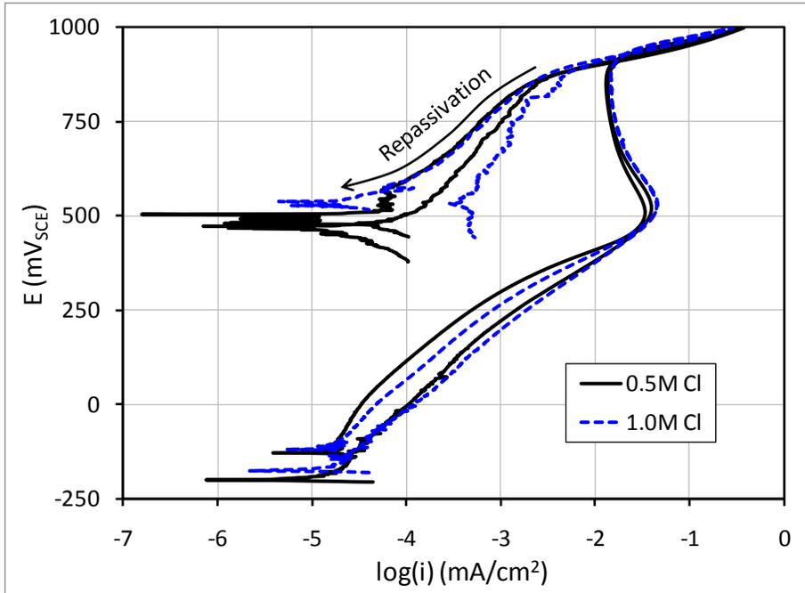
Figure 6.35 Polarization curves of 2205 strand tested in carbonated solutions
