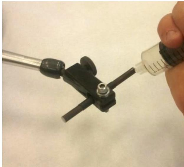
Figure D.4 Application of silicone sealant circumferentially at crevice site located at heat-shrink tubing and PTFE plug interface with wire segment
