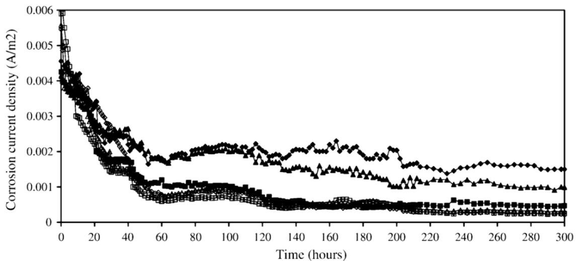
Figure 2.6 Corrosion current density vs. time indicating the formation of a passive film on the surface of steel embedded in mortar (from (Poursaeed and Hansson, 2007))
