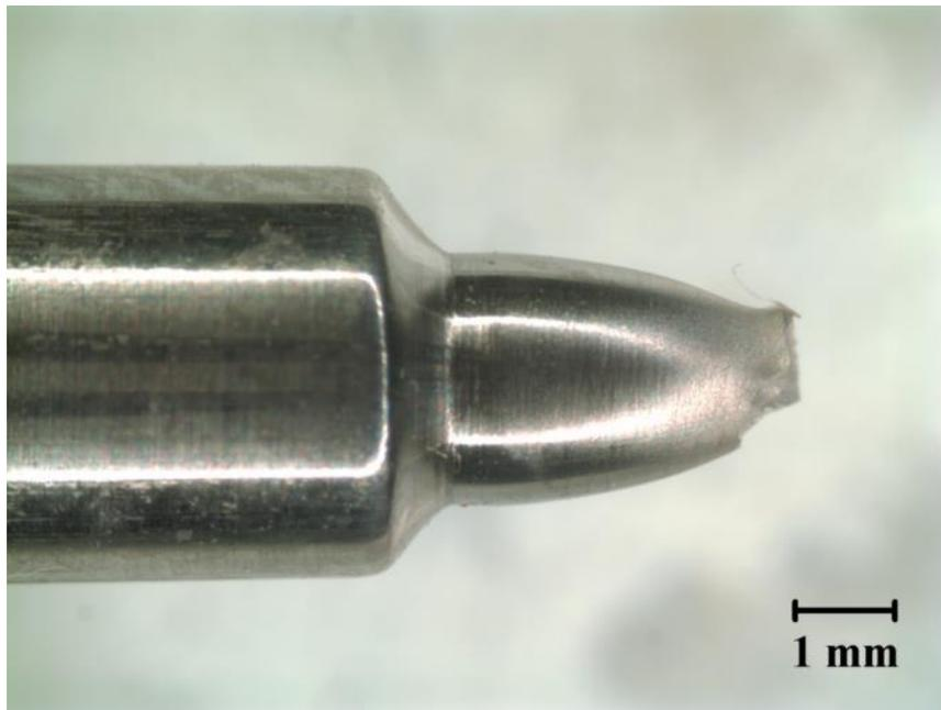
Figure I.8 2304 SSRT specimen tested in a carbonated solution with 0.5 M Cl<sup>-</sup>
