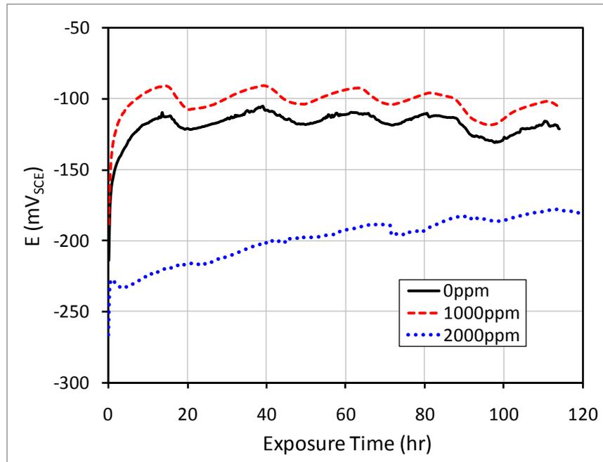
Figure H.6 2205 HSSS exposed to carbonated solutions with 0, 1000, and 2000ppm  $SO_4^{2-}$
