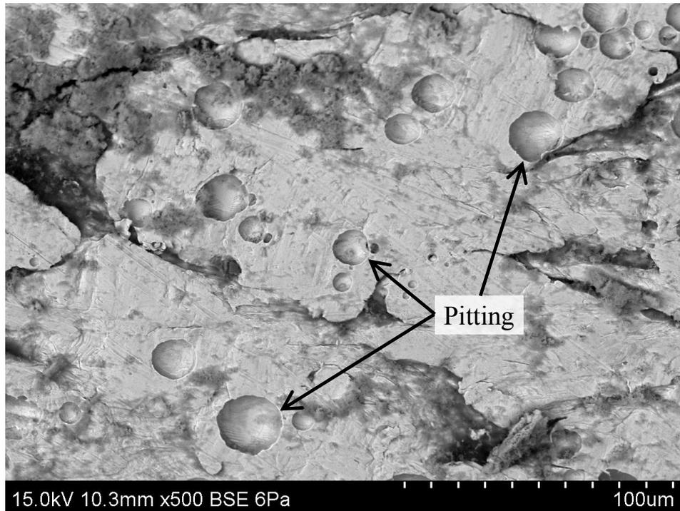
Figure 6.13 Pitting of 304 HSS tested in a carbonated solution with 0.5 M  $\text{Cl}^-$
