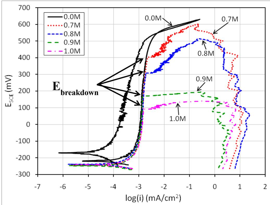
Figure 3.8 Cyclic polarization curves for prestressing wire specimens
