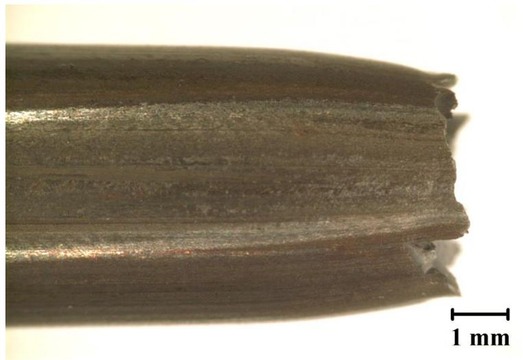
(a) Typical 1080 steel fracture surface
