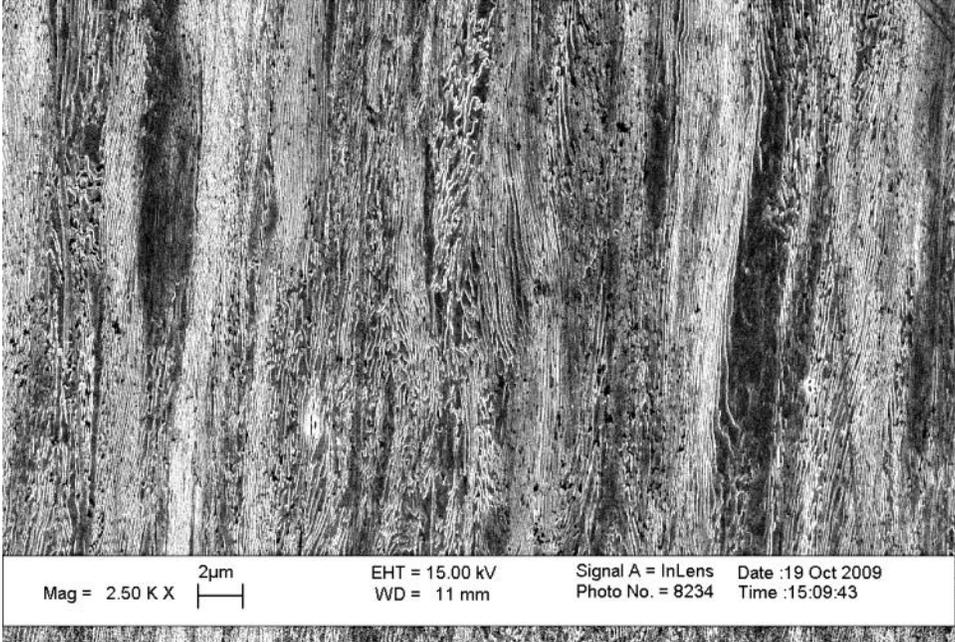
Figure B.1 Longitudinal microstructure of 1080 prestressing steel
