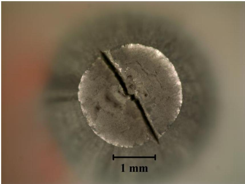
Figure C.8 Fracture surface of 2101 HSS
