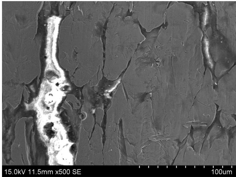
(a) SEM micrograph of surface of 304 HSSS produced by Sumiden
