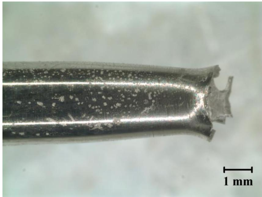
Figure I.10 2304 SSRT specimen tested in a carbonated solution with an applied cathodic potential of  $-820 \text{ mV}_{\text{SCE}}$
