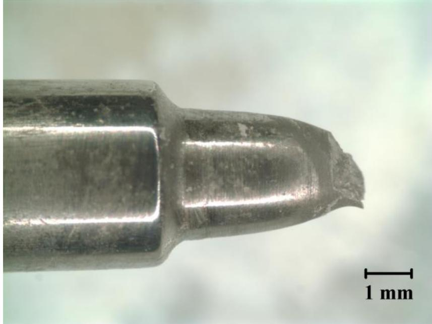
Figure I.7 2304 SSRT specimen tested in an alkaline solution with 0.5 M Cl<sup>-</sup>
