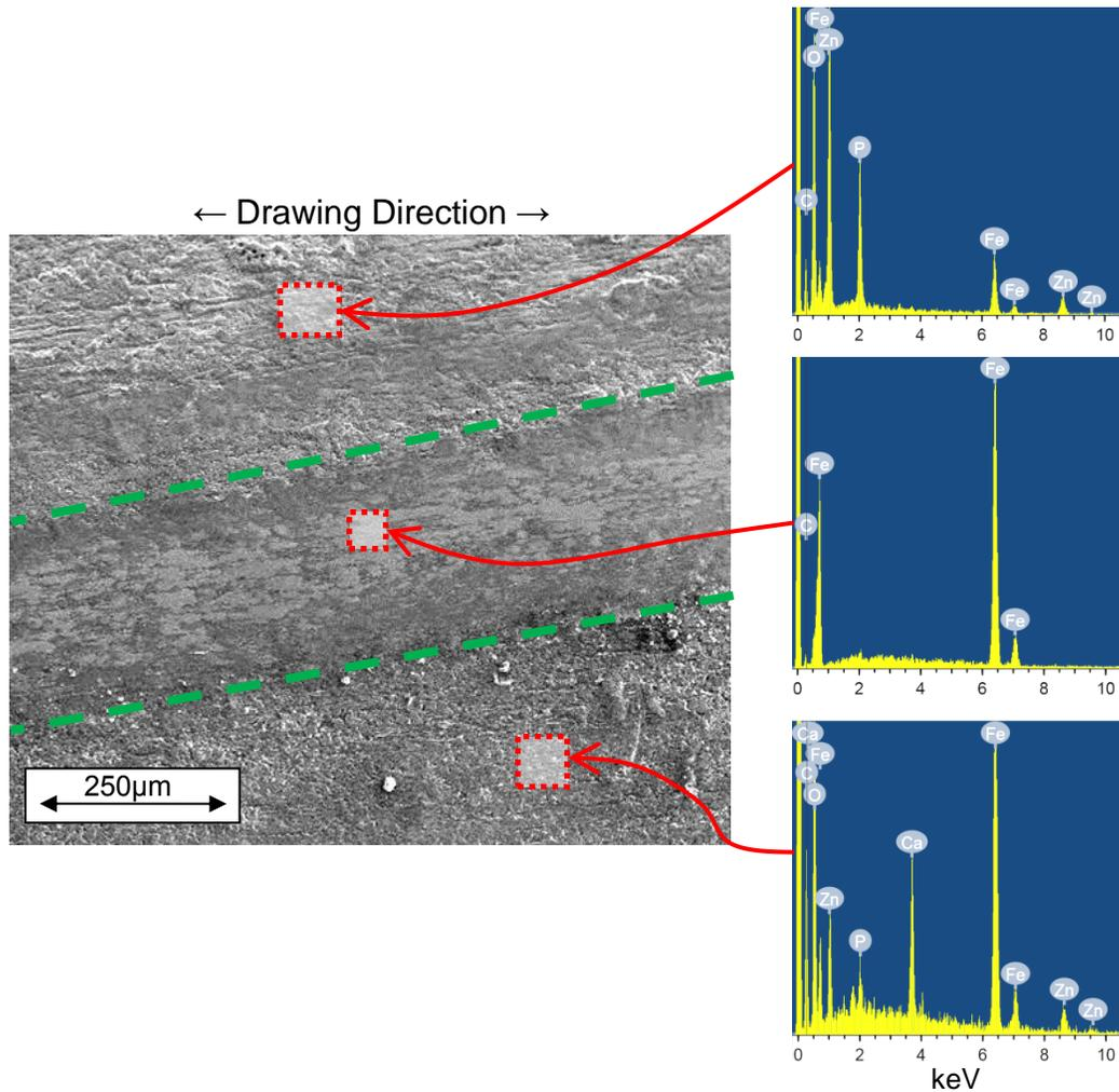
Figure 3.17 Typical Type 2 imperfection in  $ZnPO_4$  surface coating of prestressing steel
