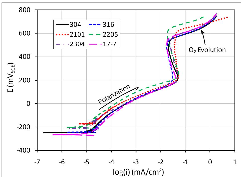
Figure 6.3 Polarization curves in alkaline solutions with 0.00 M Cl<sup>-</sup>
