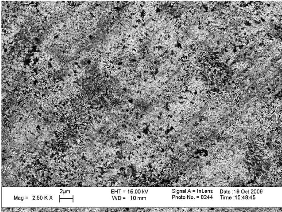
Figure B.3 Transverse microstructure of 1080 prestressing steel
