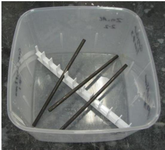
(a) Triplicate wire segments placed in  $\text{FeCl}_3$  exposure cell
