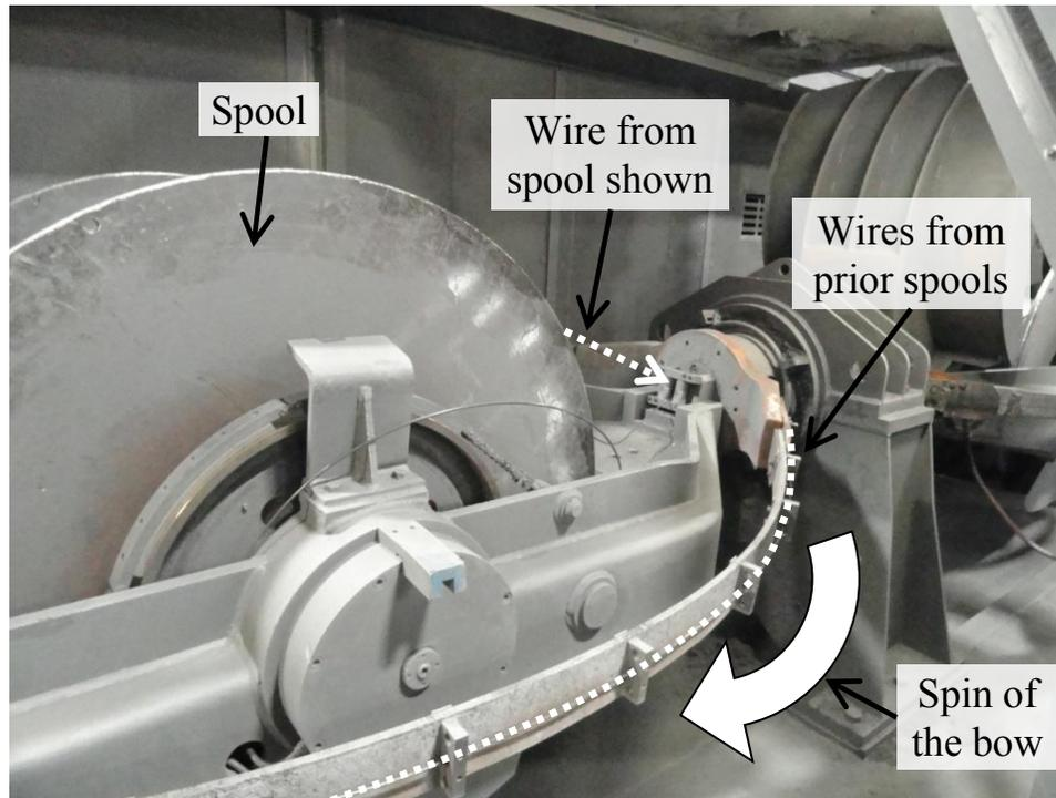
Figure 7.4 Typical configuration of bow strander at SWPC
