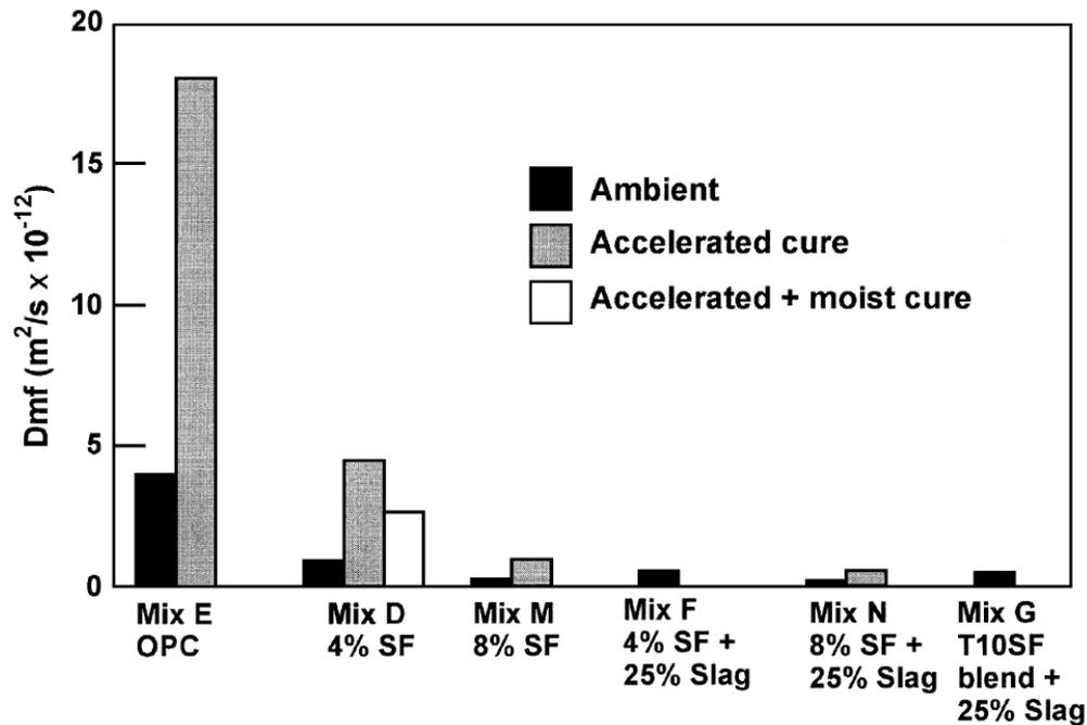
Figure 2.26 Reduction of  $\text{Cl}^-$  diffusion coefficient ( $D_{mf}$ ) with use of SCMs at a w/cm of 0.30 (from (Hooton and Titherington, 2004))
