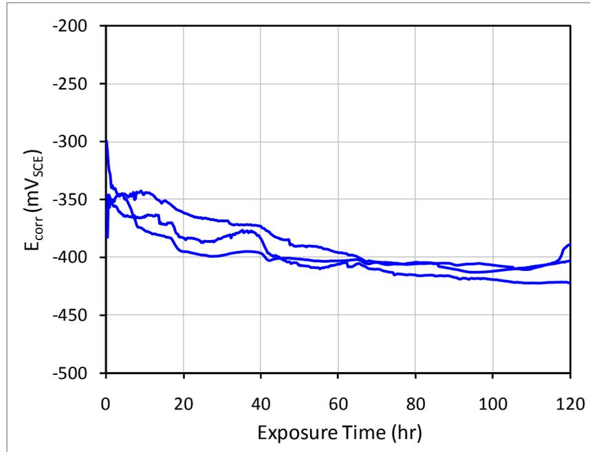
Figure G.3  $E_{corr}$  vs. time of triplicate 2304 strand specimens in alkaline solutions
