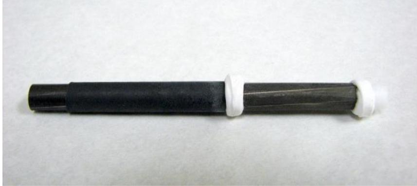
Figure D.5 Completed wire corrosion test specimen
