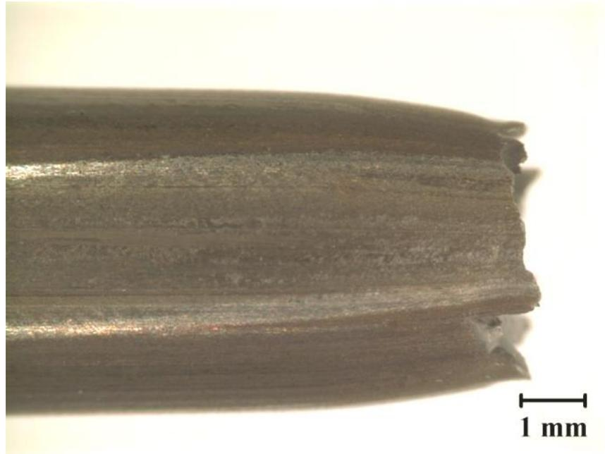
Figure C.1 Fracture surface of 1080 prestressing steel
