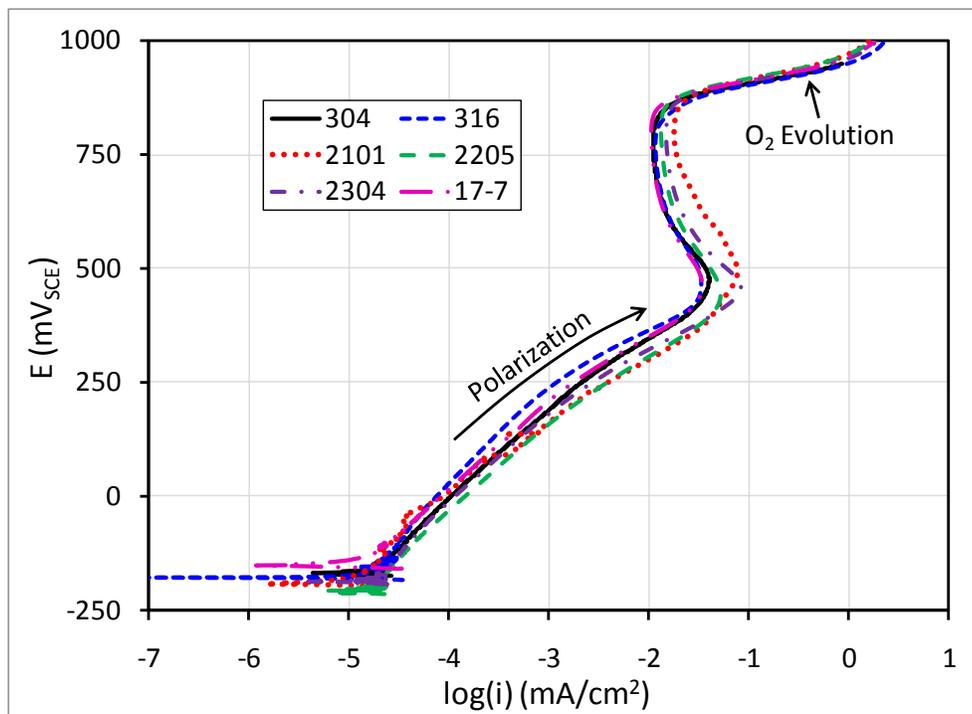
Figure 6.8 Polarization curves in carbonated solutions with 0.00 M Cl<sup>-</sup>
