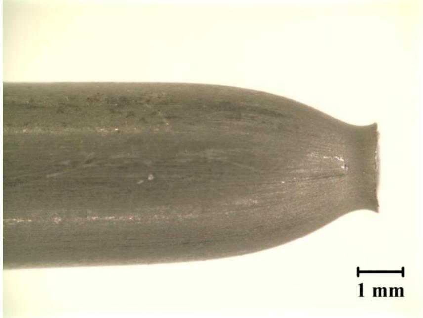
Figure C.9 Fracture surface of 2205 HSSS
