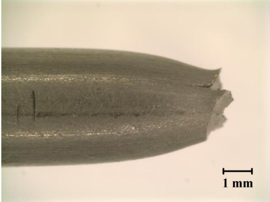
Figure C.7 Fracture surface of 2101 HSS
