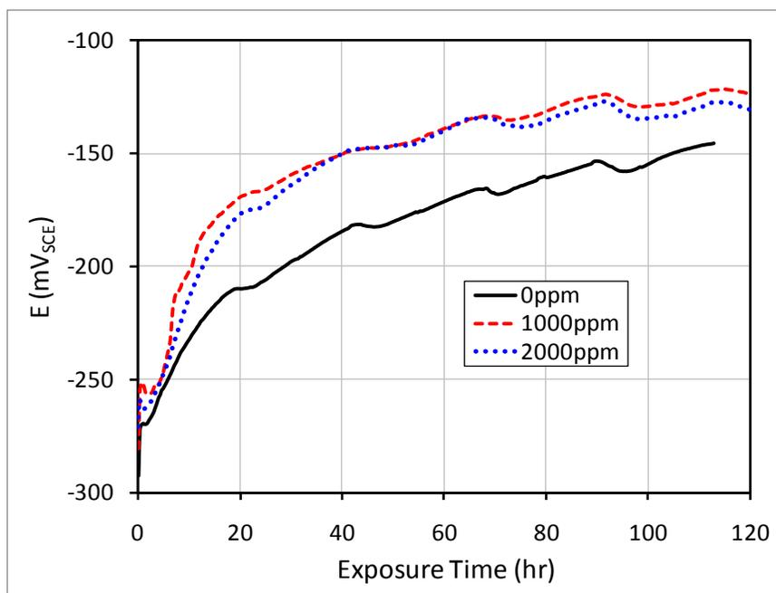
Figure H.4 304 HSS exposed to carbonated solutions with 0, 1000, and 2000ppm SO<sub>4</sub><sup>2-</sup>
