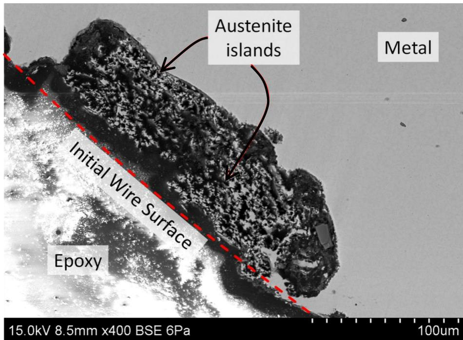
Figure 6.27 Selective dissolution of ferrite in large corrosion pit in 2101 HSS tested in carbonated solution with 1 M Cl<sup>-</sup>
