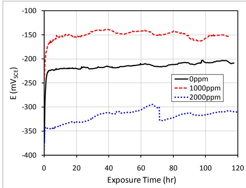
Figure H.5 2205 HSSS exposed to alkaline solutions with 0, 1000, and 2000ppm  $SO_4^{2-}$
