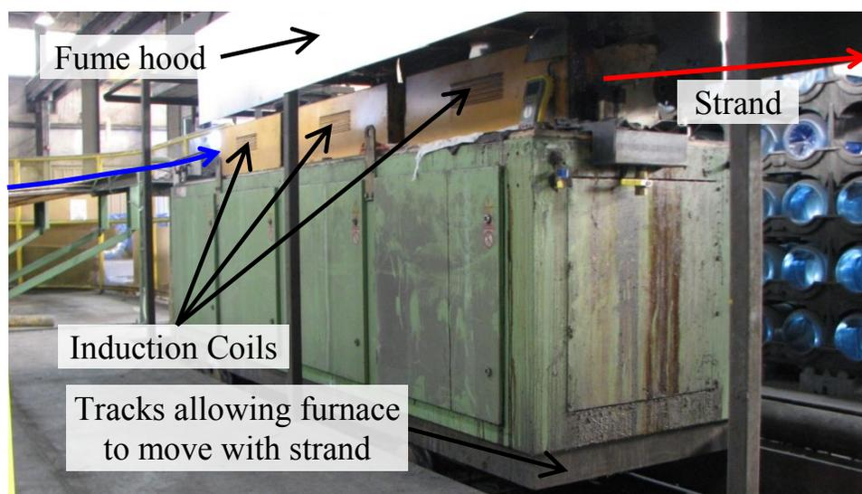
Figure 7.9 Three-coil induction furnace for low-relaxation heat treatment
