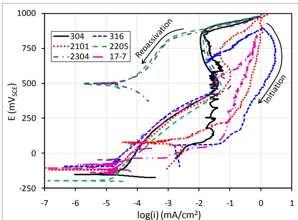
Figure 6.9 Polarization curves in carbonated solutions with 0.25 M Cl<sup>-</sup>
