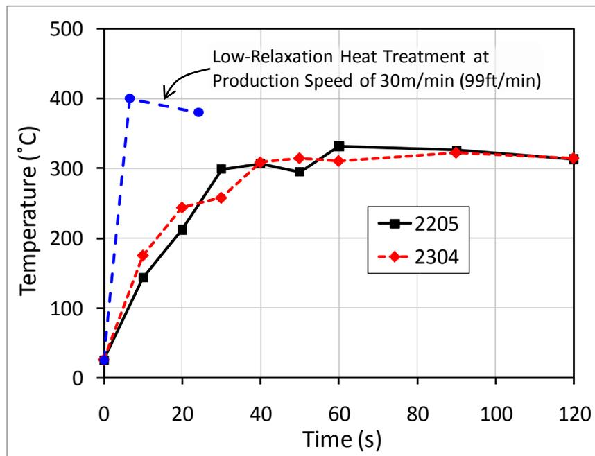
Figure 7.17 Temperature vs. time within 25 cm (10 in) nozzle
