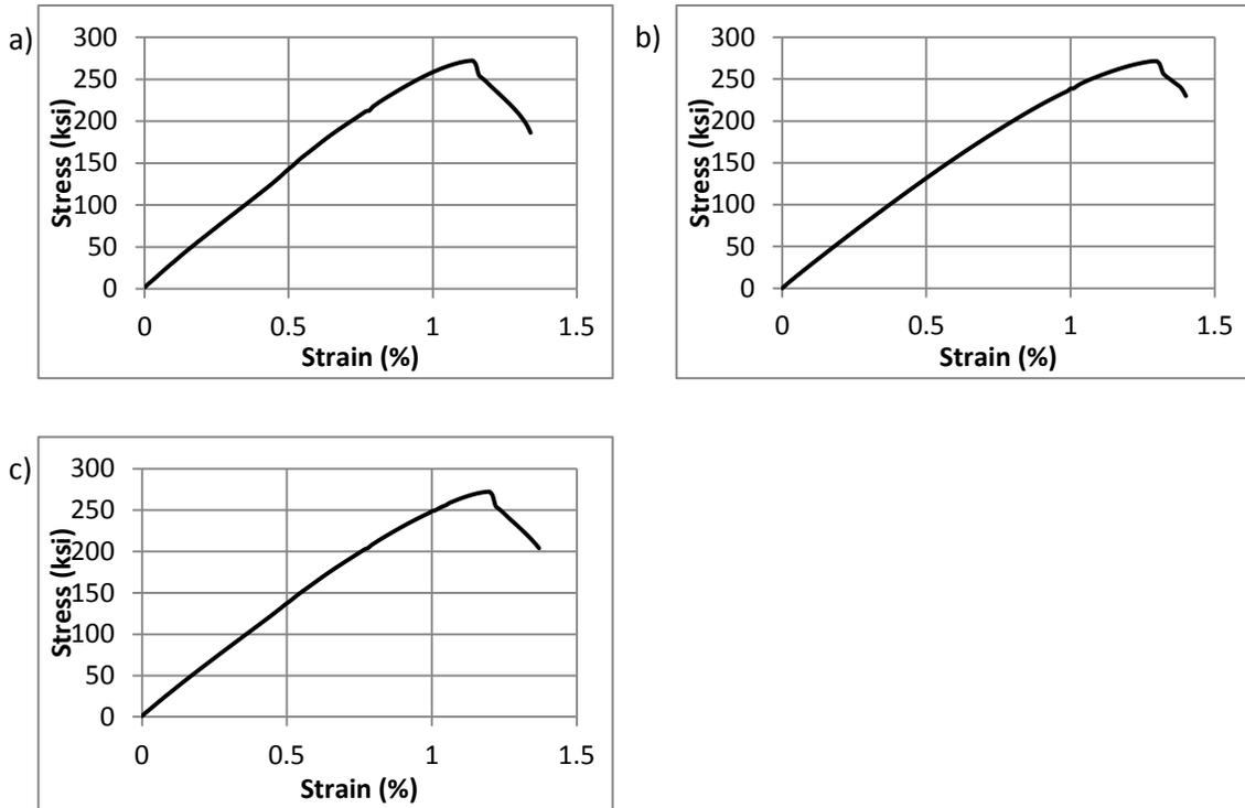
Figure J.12 2304 #7 HW wire stress-strain curves for a) test 1, b) test 2, and c) average
