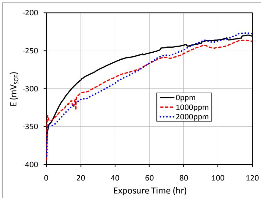
Figure H.3 304 HSS exposed to alkaline solutions with 0, 1000, and 2000ppm SO<sub>4</sub><sup>2-</sup>
