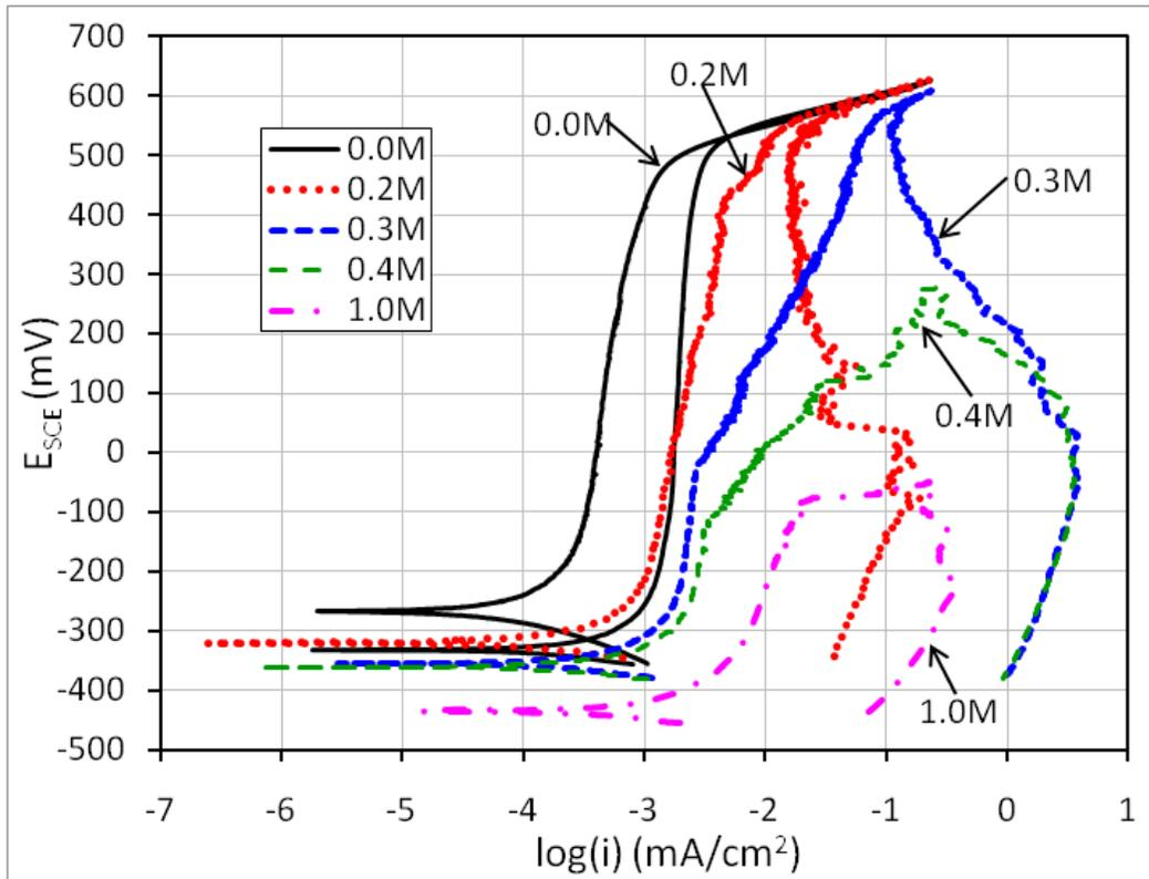
Figure 3.10 Cyclic polarization curves for prestressing strand specimens
