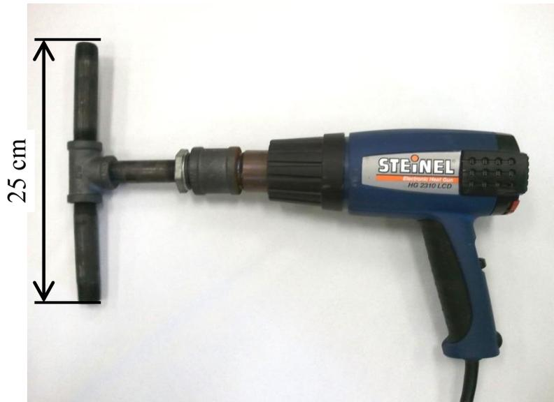
Figure 7.16 Heat gun with T-shaped nozzle attachment
