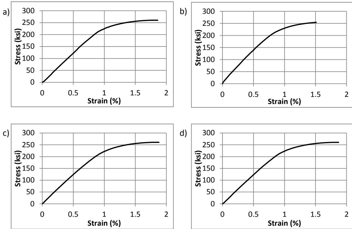
Figure J.2 2304 strand stress-strain curves for a) test 1, b) test 2, c) test 3, and d) average
