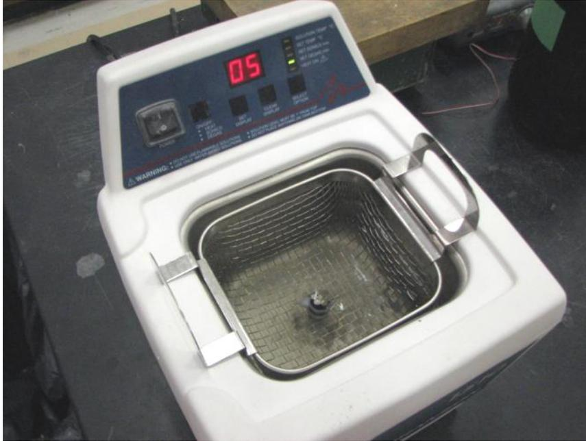
Figure E.2 Strand segments ultrasonicated in ethanol for 1 min following cutting to remove scale and debris from the interstices of the strand.
