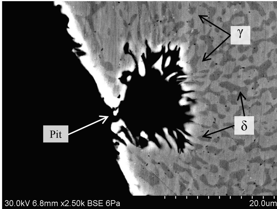
Figure 6.25 Dissolution of ferrite in 2101 HSSS tested in alkaline solution with 1M Cl<sup>-</sup>
