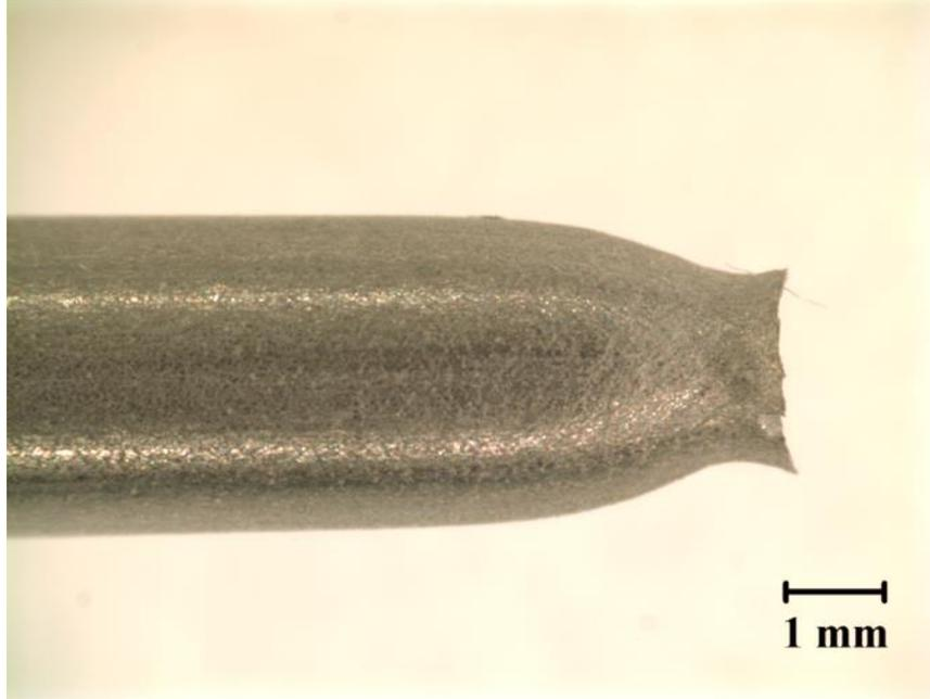
Figure C.5 Fracture surface of 316 HSSS
