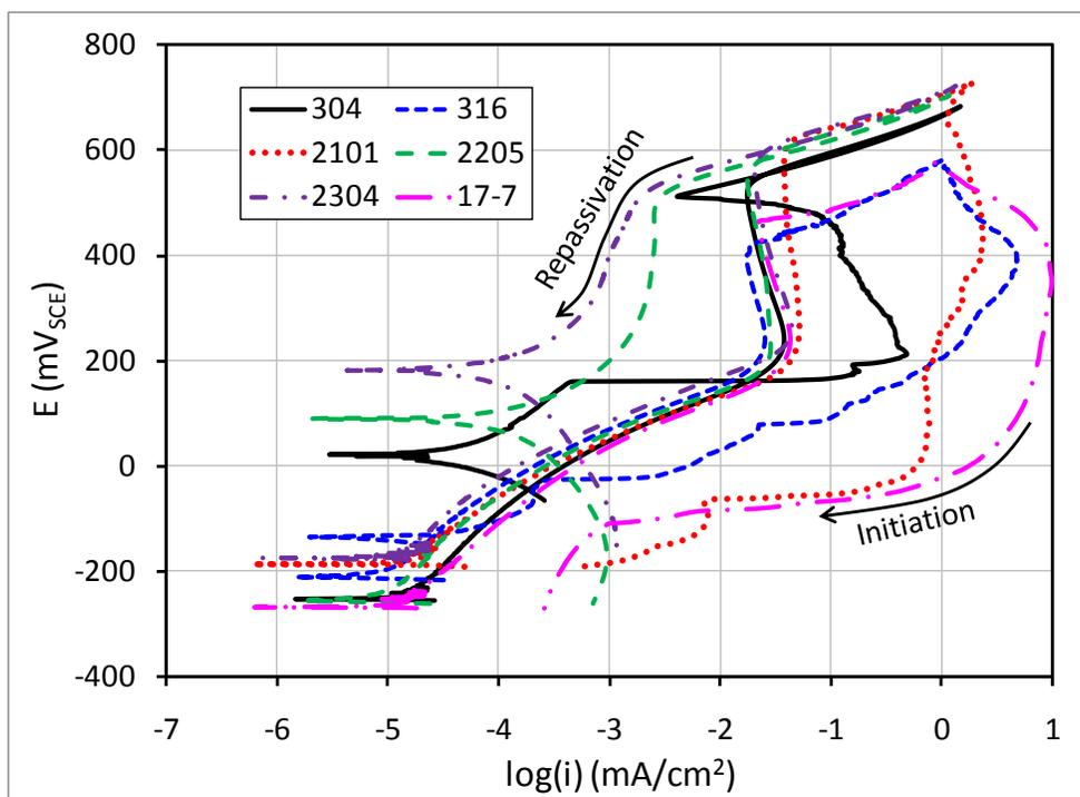
Figure 6.5 Polarization curves in alkaline solutions with 0.50 M Cl<sup>-</sup>
