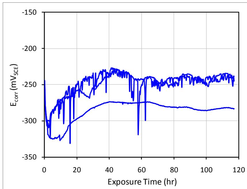
Figure G.4  $E_{corr}$  vs. time of triplicate 2304 strand specimens in carbonated solutions
