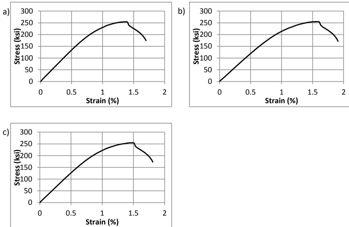
Figure J.11 2304 #7 UW wire stress-strain curves for a) test 1, b) test 2, and c) average
