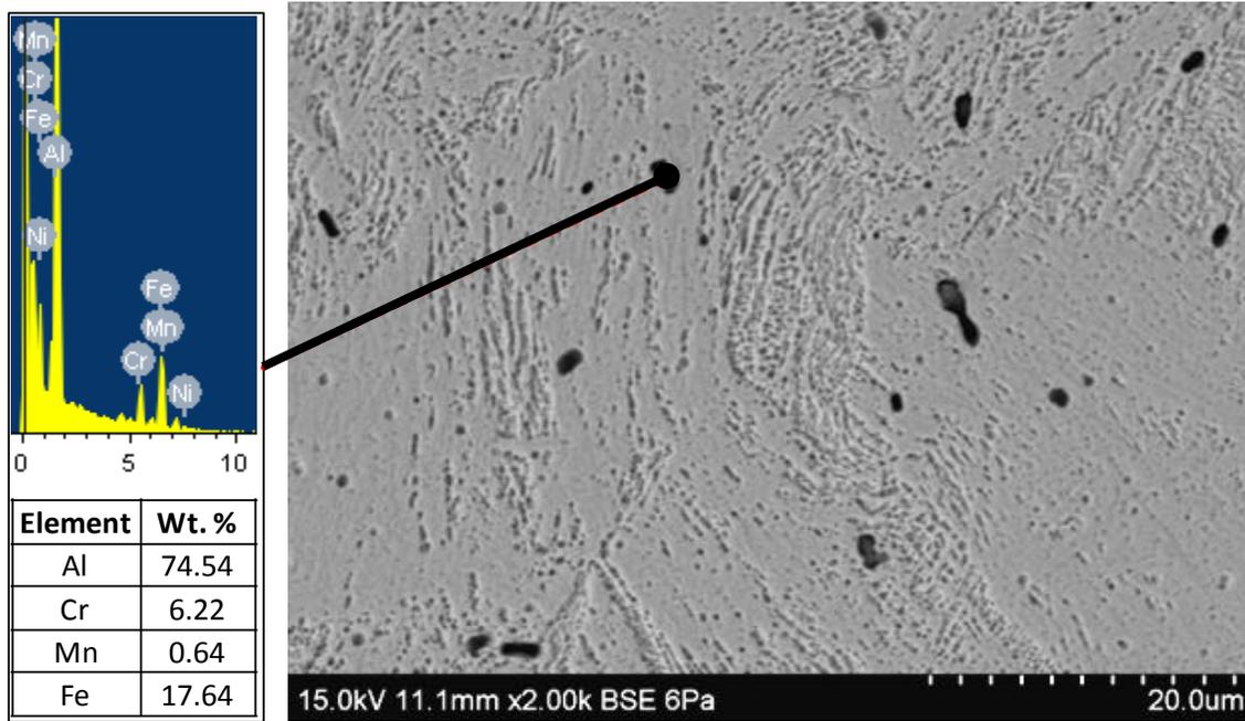
Figure 4.18 Distributed precipitates shown in etched 17-7 HSSS
