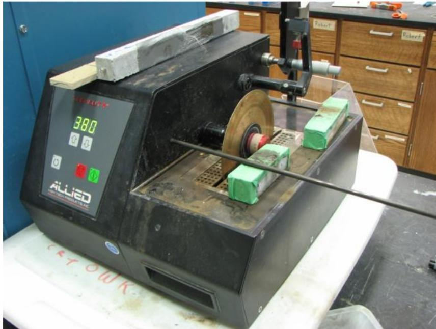
Figure D.1 Wire rod cut using slow-speed water-cooled diamond saw
