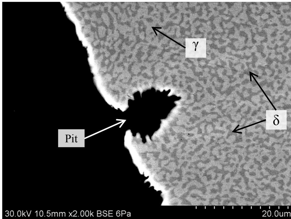
Figure 6.26 Dissolution of ferrite in 2304 HSSS tested in carbonated solution with 1M Cl<sup>-</sup>
