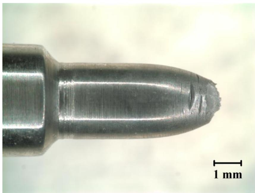
Figure I.4 2205 SSRT specimen tested in an alkaline solution with an applied cathodic potential of  $-1000 \text{ mV}_{\text{SCE}}$
