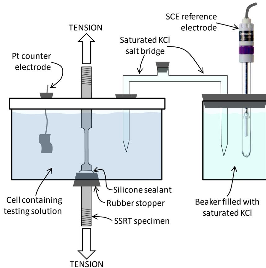
Figure 6.41 Experimental setup for HE SSRTs
