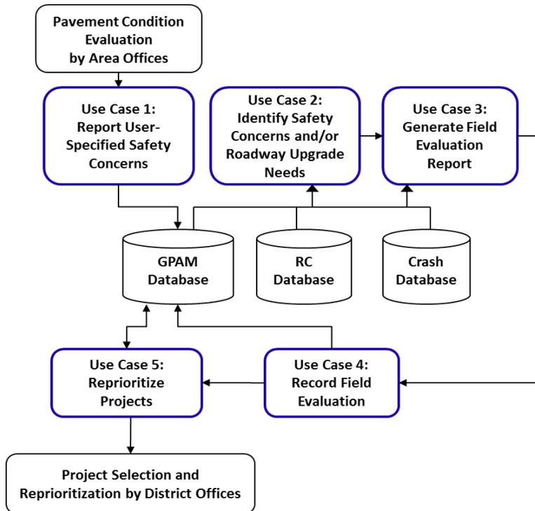
**Figure 7.2 Process and Data Flow of the Proposed Safety-Incorporated Resurfacing Program**
