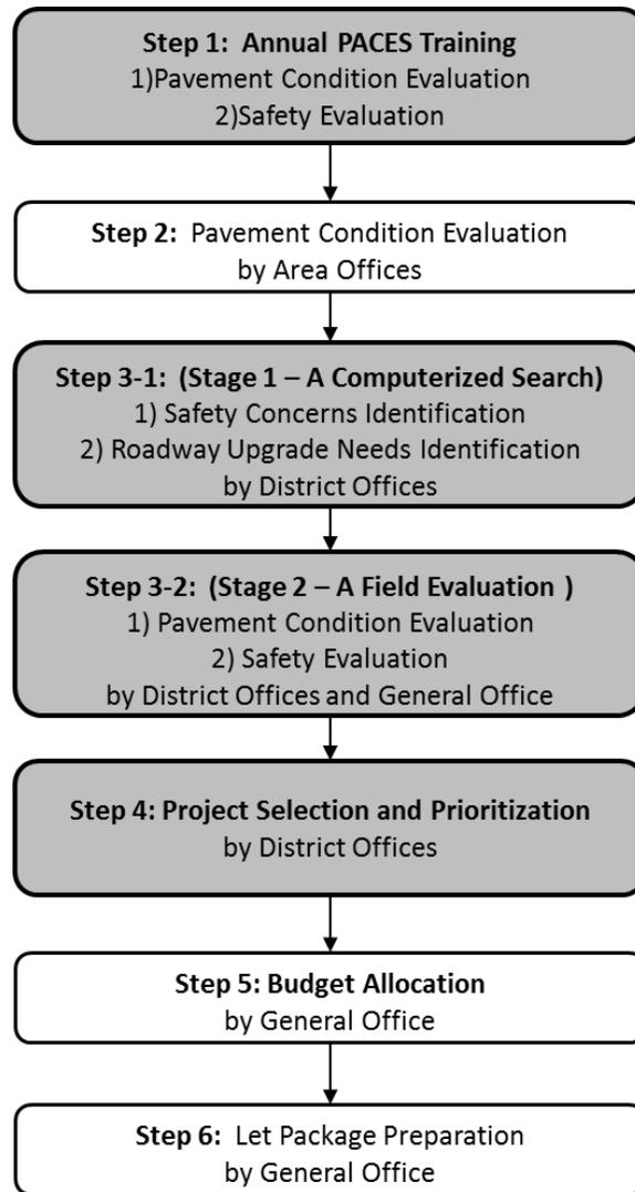
**Figure 5.6 Safety-Incorporated Resurfacing Program for GDOT**
