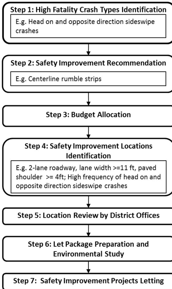
**Figure 4.2 Process for System-wide Improvement**
