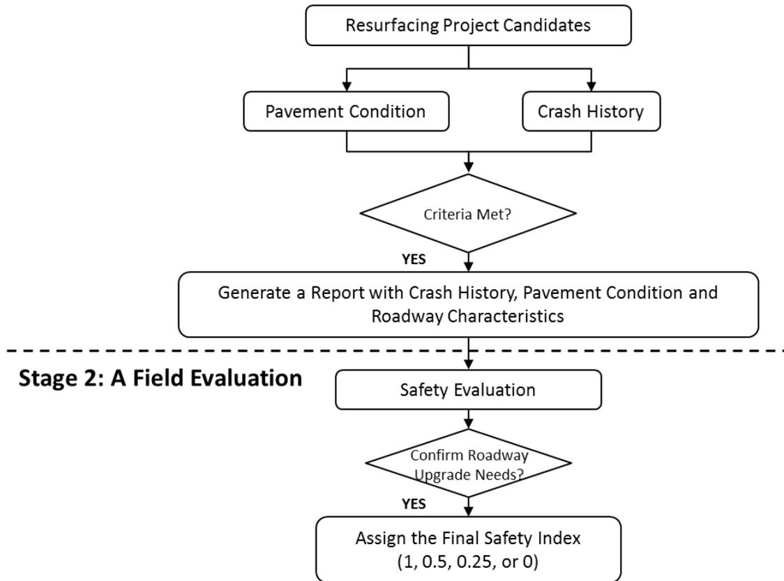
**Figure 5.4 Two-Stage Roadway Upgrade Needs Identification**
