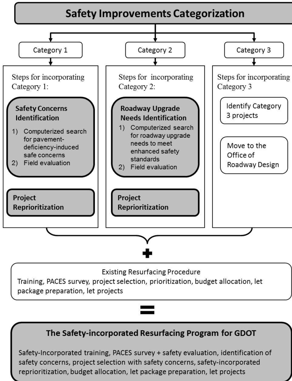
**Figure 5.1 Overview of the Proposed Safety-Incorporated Resurfacing Program**
