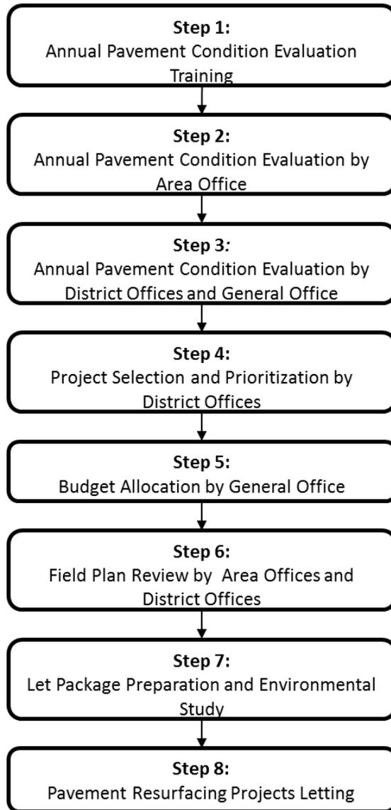
**Figure 3.1 Procedures for GDOT’s Resurfacing Program**
