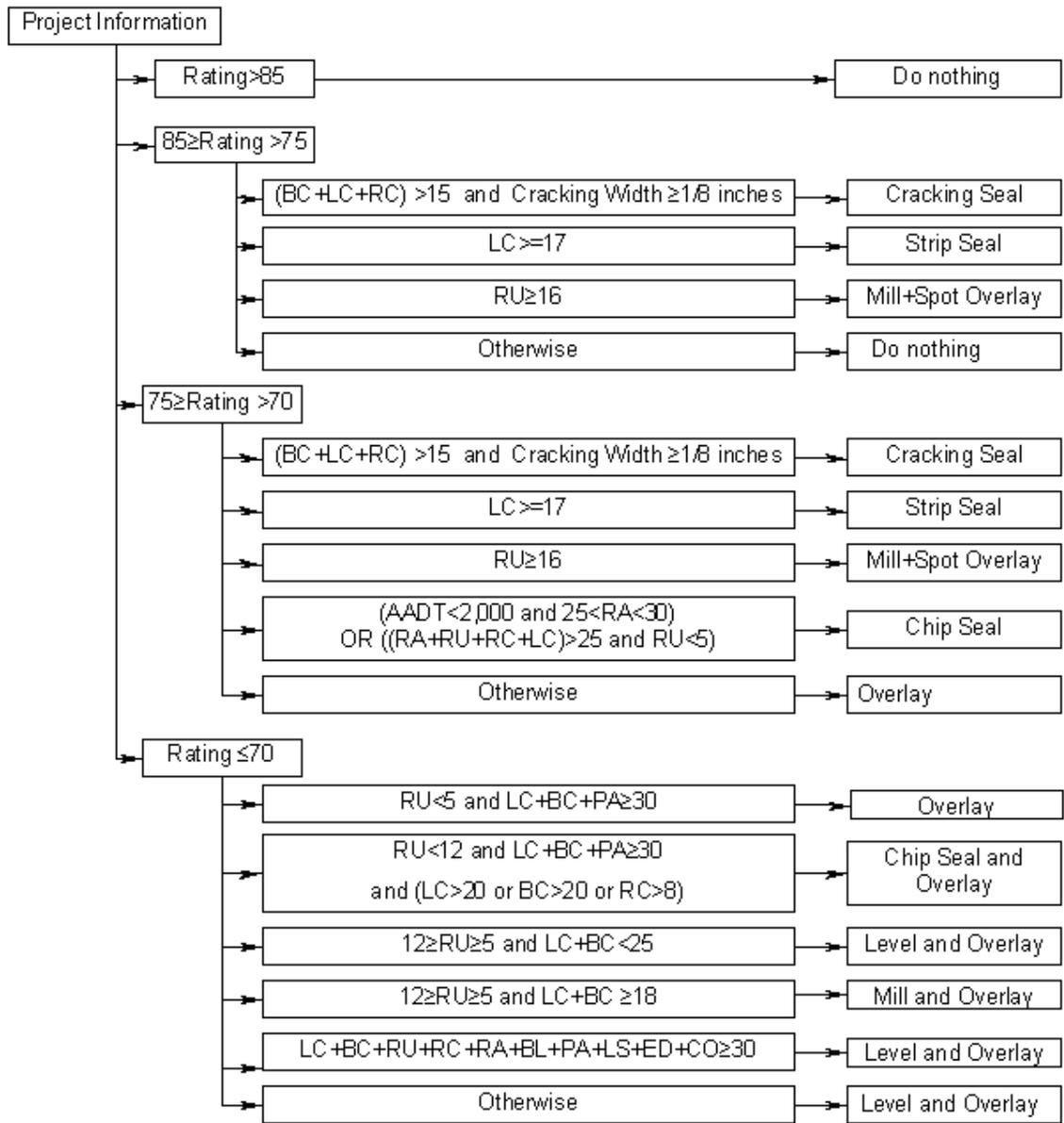
BC: Blocking cracking deduct value; LC: Load cracking deduct value;
