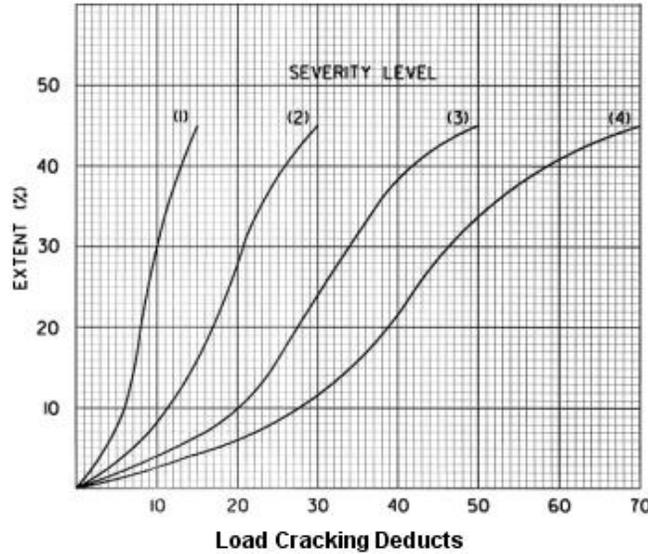
**Figure 3.2 Deduct Values for Load Cracking**
