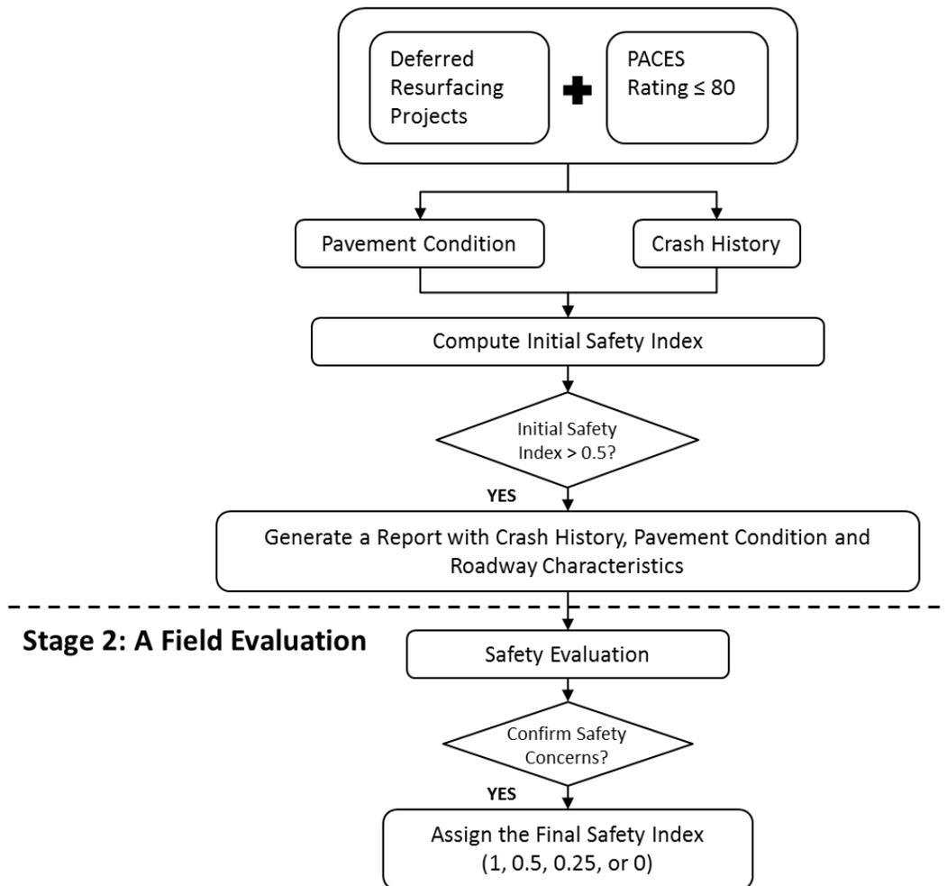
Figure 5.2 Two-Stage Safety Concerns Identification
