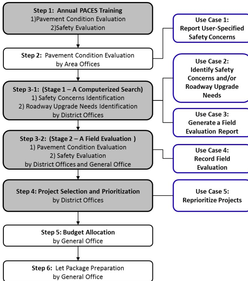
**Figure 7.1 Use Cases for the Proposed Procedure**
