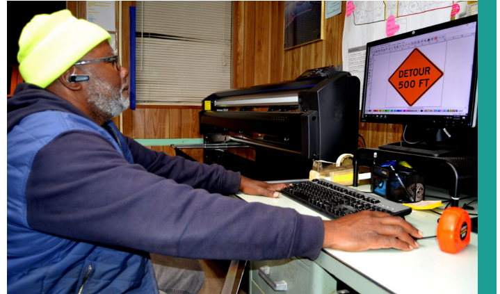
Equipment Operator Anthony Walker reviews a detour sign. Designs made from a library on the computer go to a plotter for printing on reflective vinyl sheeting.
