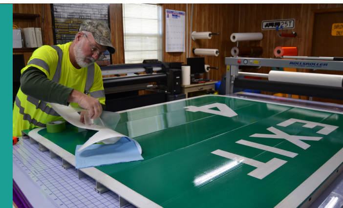
Highway Maintenance Foreman Tim Walker peels transfer paper off an arrow on a panel sign to replace a damaged Liberty Expressway exit sign in Albany.
