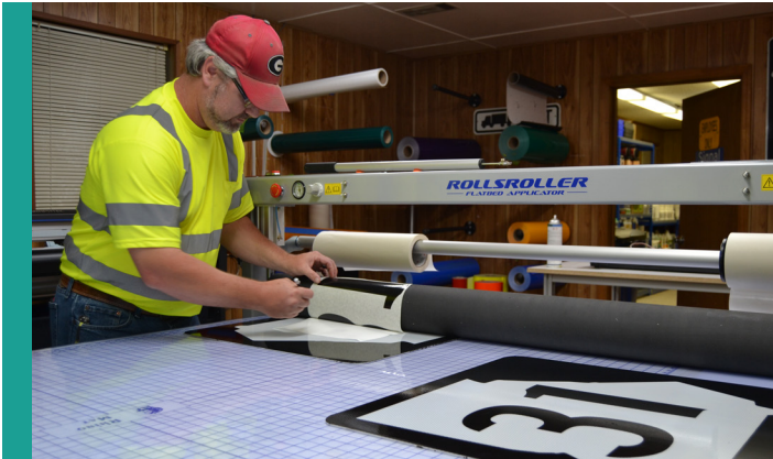
Highway Maintenance Foreman Dale Price uses the new cold press table to apply the numbers "31" to a blank state sign for a road detour.
