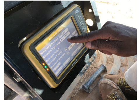
Many large construction equipment vehicles today are outfitted with GPS systems that help operators perform a variety of tasks, including excavating, grading and paving.
