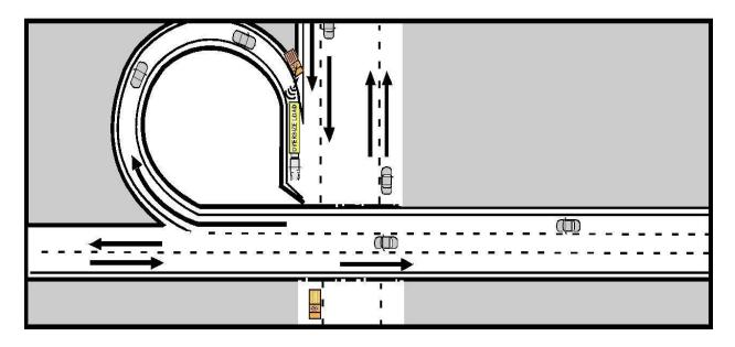
Fig. 14: Rear escort vehicle monitors clearances.
