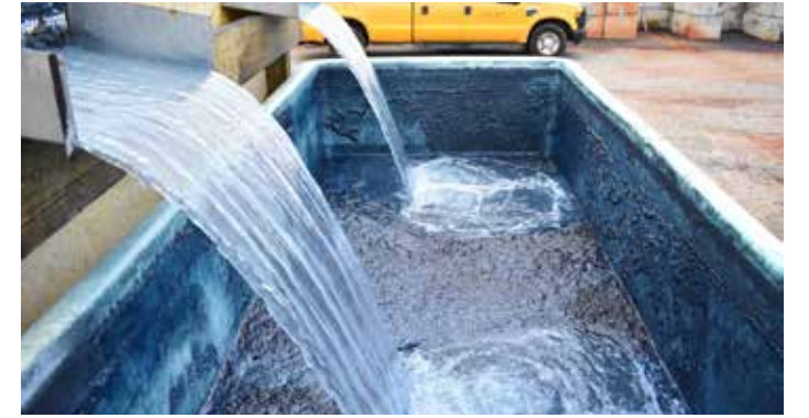
Making brine. Brine, a mixture of salt and water, is a preventative treatment that limits the bonding of ice to the pavement. Georgia DOT spread about 600,000 gallons of brine on the interstates for Helena. Photo: Kyle Collins, GDOT
