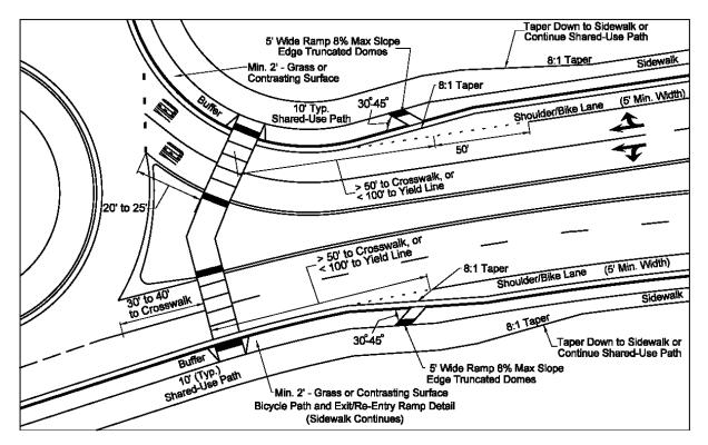
Figure 4-4. Bicycle Path Exit and Entry with Extended Sidewalk
