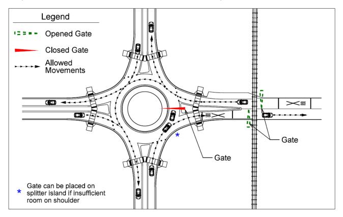
Figure 6-2A. Track clearance stage with gated closure for circulating flow
