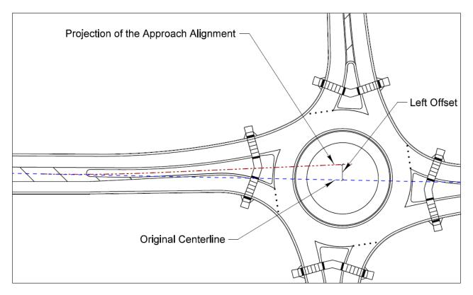
Figure 3-8. Left Offset Design for Entry Deflection
