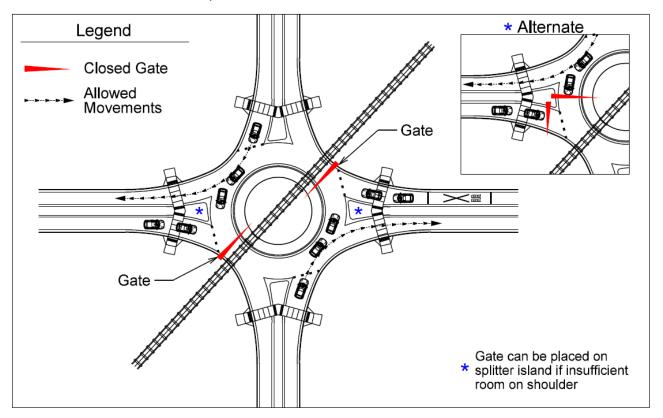
Figure 6-4. Railroad through the roundabout
