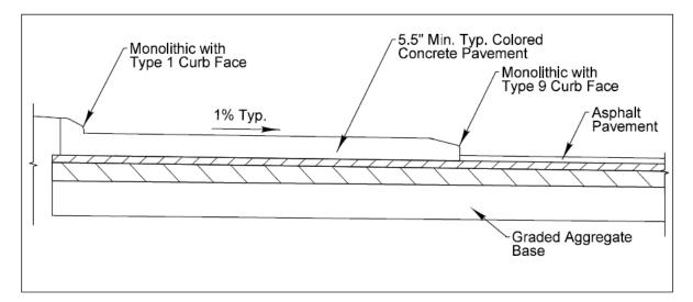
Figure 3-40A. Outside Truck Apron (Monolithic) Typical Section
