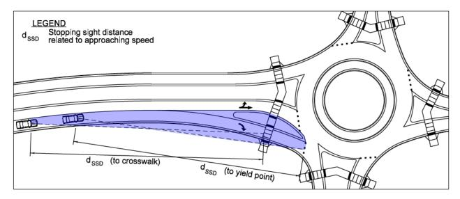
Figure 3-20. Approach SSD (with Bypass Lane)
