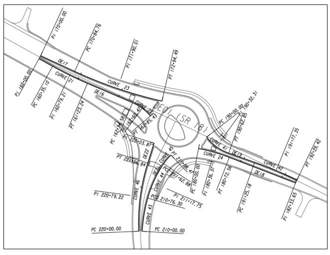
Figure F-1. Splitter Island Alignments
