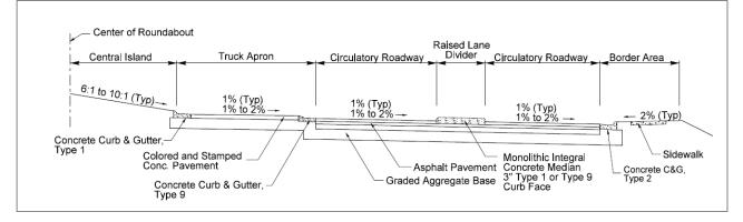
Figure 3-44. Case 3 Multilane Roundabout Circulatory Roadway Typical Section
