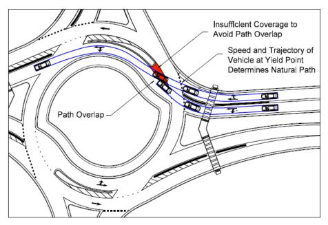
Figure 3-32. Case 3 Multilane Roundabout with Path Overlap (Avoid)
