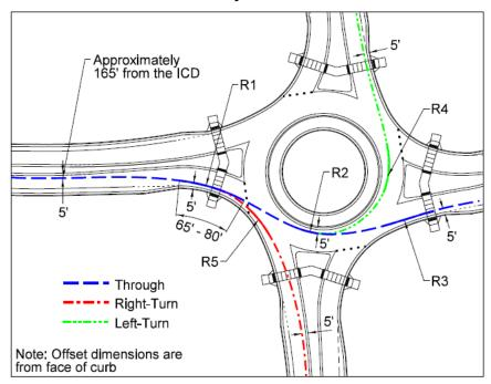
Figure 3 13. Determination of Entry Path Curvature – Single Lane Roundabouts
