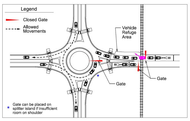
Figure 6-2B. Track clearance stage with gated closure for circulating flow and at track crossing
