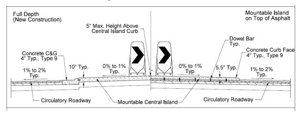
Figure 3-45. Mountable Apron at Mini-Roundabouts, shown with Bollards
