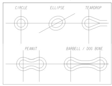
Figure 3-7. Roundabout Shapes
