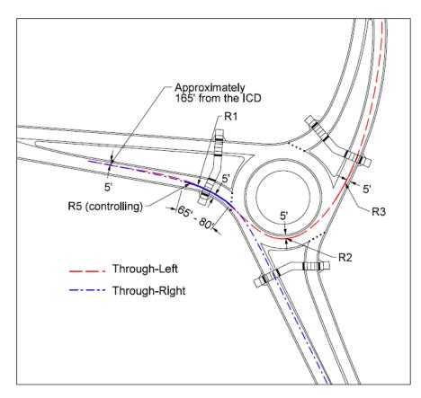
Figure 3-14. Determination of Entry Path Curvature – Y Roundabouts
