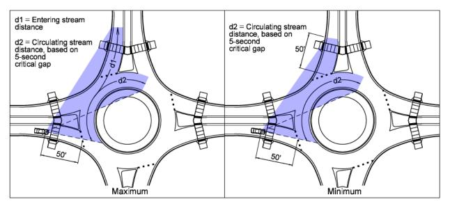
Figure 3-24. Maximum and Minimum Intersection Sight Distance
