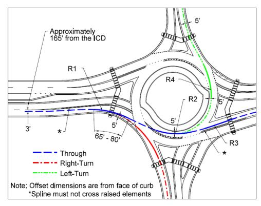
Figure 3-16. Determination of Entry Path Curvature – Multilane Roundabouts Case 2
