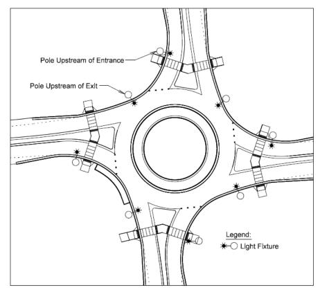
Figure 7-1. Perimeter Pole Placement
