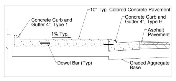
Figure 3-40B. Outside Truck Apron Typical Section
