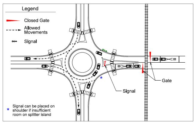
Figure 6-5. Signal at roundabout with gate at railroad crossing
