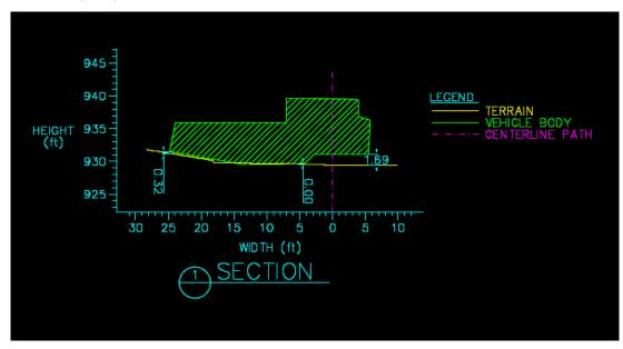
Figure D-12. Vertical Check Punch Through Example
