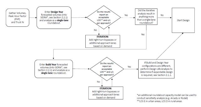
Typically, four operational performance measures are used to estimate the operational performance of a roundabout entry: volume-to-capacity ratio, control delay, LOS, and queue length. These measures are checked to be within the desirable ranges for each lane configuration throughout the iterative process.
