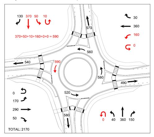
Figure 9-1. Circulating Volume Calculation
