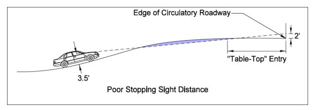
Figure 3-23. Vertical Considerations of Approach Stopping Sight Distance
