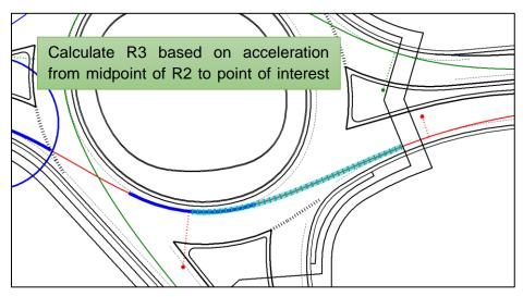
Figure D-4. Calculating R3
