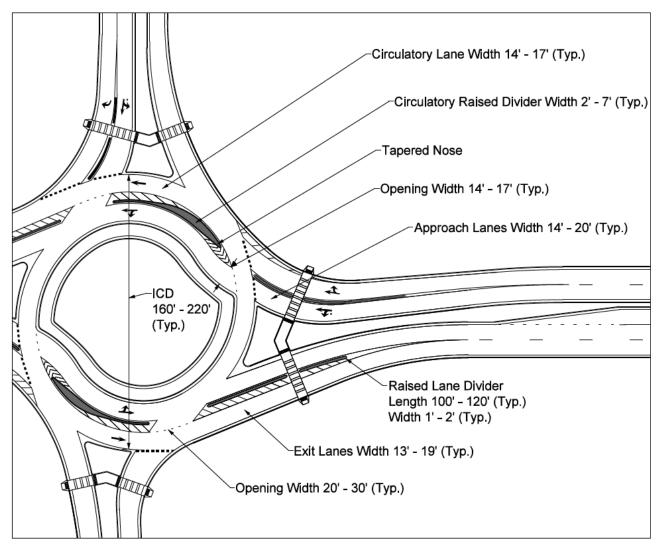
Figure 3-34. Case 3 Multilane Roundabout Opening Width and Path
