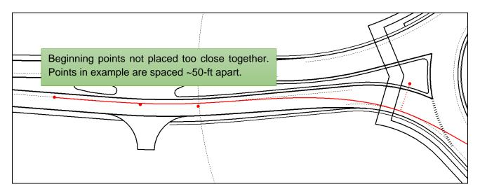
Figure D-1. Control Points on Approach
