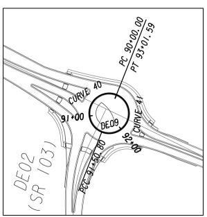
Figure F-3. Station of Circulatory Alignment
