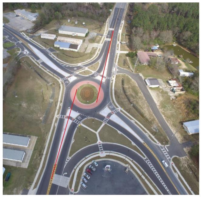
Figure A-3. Offset Left Design Example
