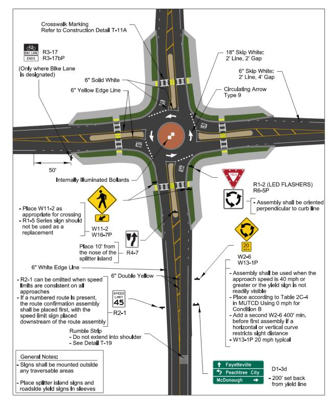
Figure 5-1. Mini-Roundabout Signing and Marking
