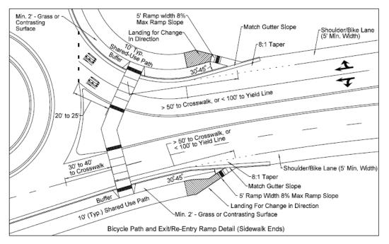
Figure 4-3. Bicycle Path Exit and Entry without Extended Sidewalk
