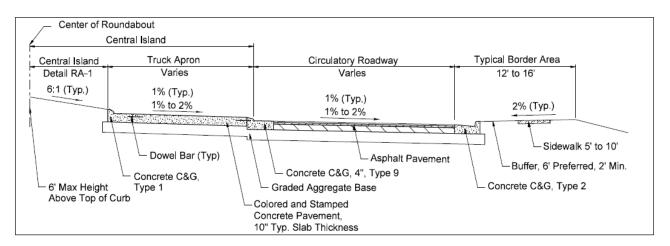
Figure 3-38B. Roundabout Detailed Section
