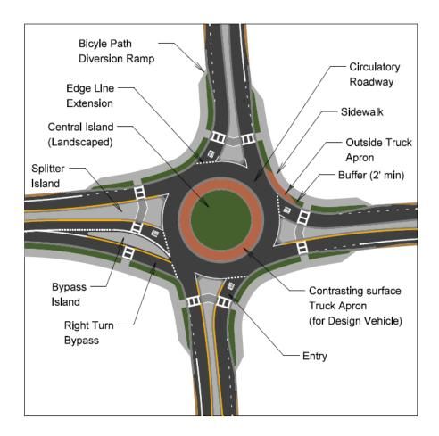
Figure 1-1. Key Roundabout Features
