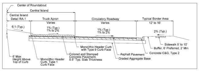
Figure 3-38A. Roundabout Detailed Section with Monolithic Truck Apron
