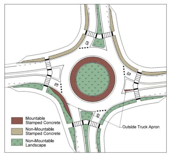
Figure 8-6. Truck Apron Coloring & Patterning
