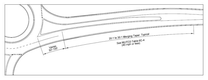
Figure 3-9b. High-Speed Multilane Exit Design
