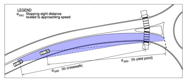
Figure 3-18. Approach Stopping Sight Distance (SSD)
