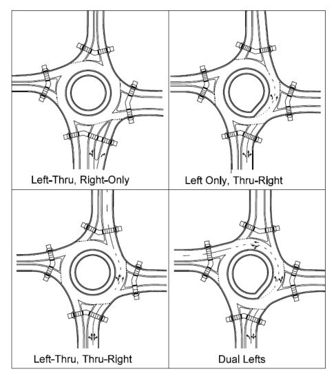
Figure 2-1. Lane Configuration Options for Two-lane Entry
