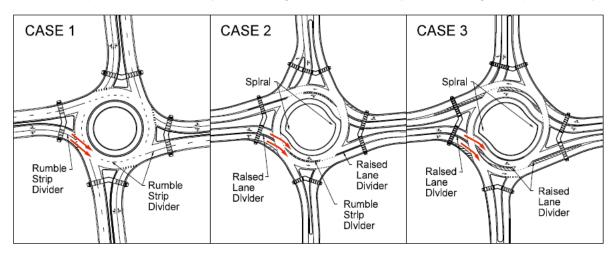
Figure 1-2. Multilane Roundabout Key Features
