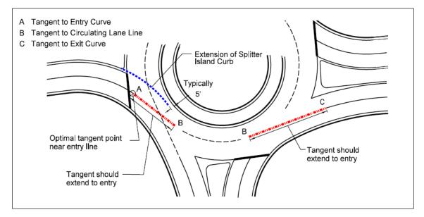
Figure 3-31. Method for Checking Path Overlap (Case 1)
