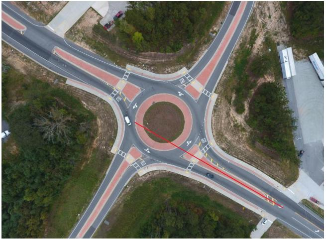
Figure A-2. Offset Left Design Example
