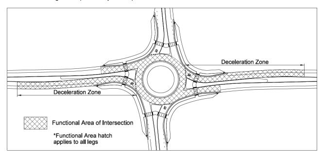
Figure 3-2. Roundabout Functional Area
