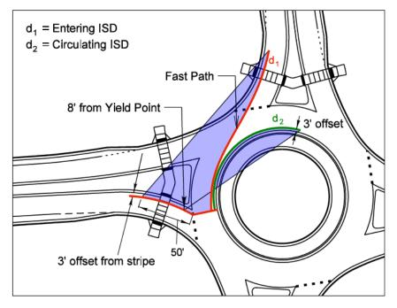
Figure D-9. Entering and Circulating ISD
