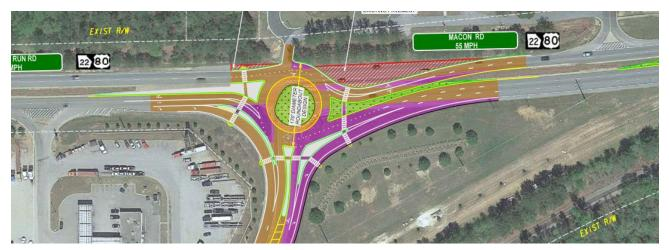
Figure A-5. Refined Roundabout Design
