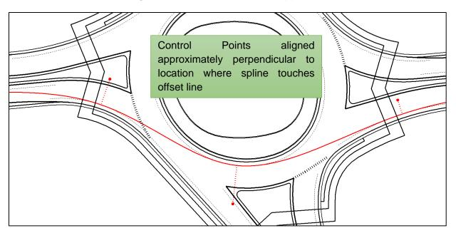
Figure D-2. Control Points Entry, Circulating, Exiting
