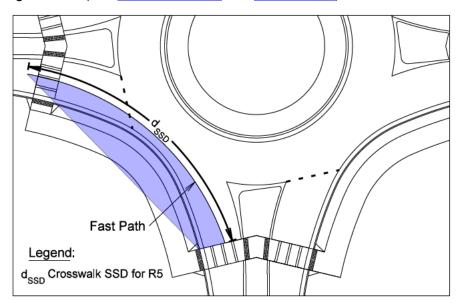
Figure D-7. SSD to Crosswalk on Exit
