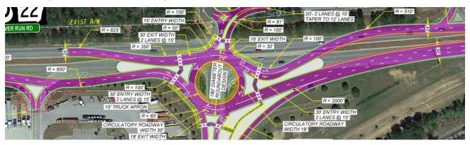
Figure A-4. Original Roundabout Design
