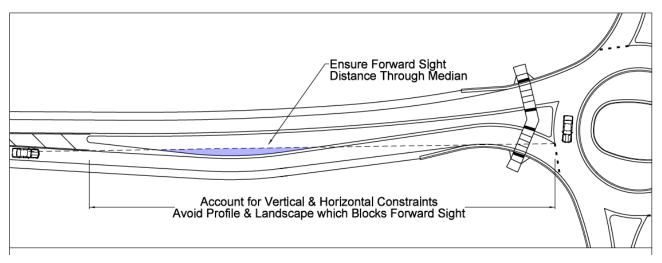
Figure 3-19. Approach SSD (with Reverse Curves)
