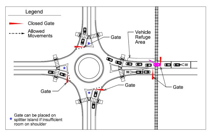
Figure 6-3B. Pre-empt hold stage with gated closures at approach entries and railroad crossing
