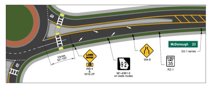
Figure 5-6. Lane Drop Multilane Roundabout Signing and Marking
