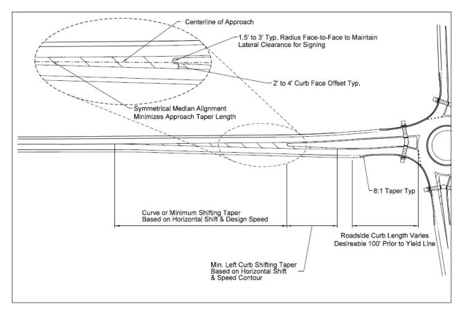
Figure 3-9a. High-Speed Approach Design
