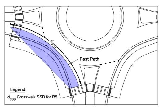
Figure 3-21. Stopping Sight Distance to the Downstream Crosswalk
