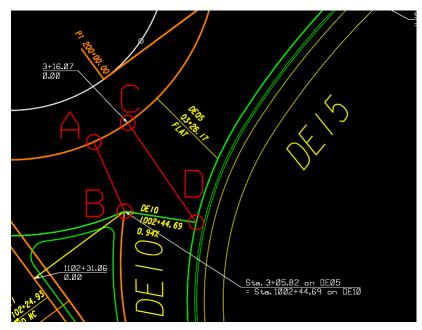
Figure F-6. Points of Station Equivalents
