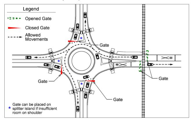
Figure 6-3A. Track clearance stage with gated closures at roundabout approach entries
