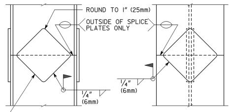
$^{\prime}$ 6" (I50mm) X 6" (I50mm) X  $^{\prime}$ 16" (I1mm) SPLICE PL'S. FOR HP IO (HP 250) 7" (I75mm) X 7" (I75mm) X  $^{\prime}$ 16" (I1mm) SPLICE PL'S. FOR HP I2 (HP 3IO) 8 $^{\prime}$ 2" (215mm) X 8 $^{\prime}$ 2" (215mm) X  $^{\prime}$ 2" (13mm) SPLICE PL'S. FOR HP I4 (HP 360)
