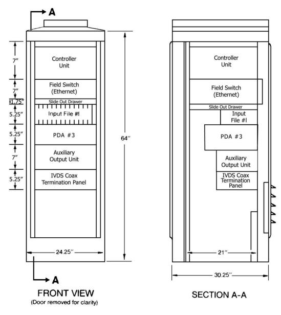
Figure 925-1 Typical 334 Cabinet Configuration
