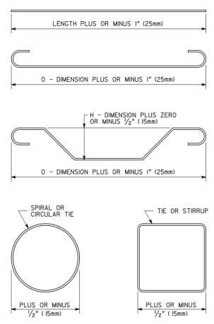
Figure 1 – Fabrication Tolerances
