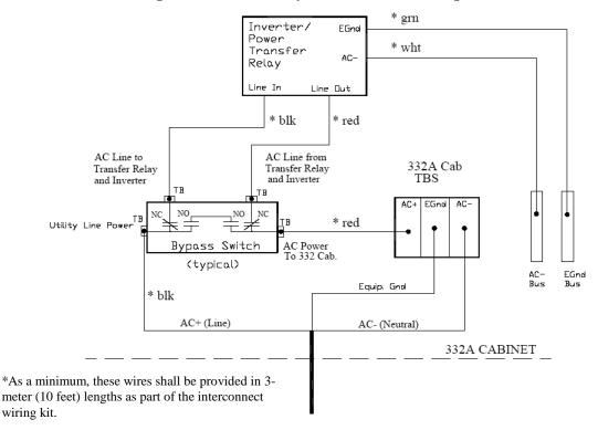
Figure 925- 7 BBS Utility Power Connection Diagram
