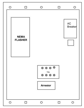
Note: Front view of cabinet Door Assembly not shown No scale
