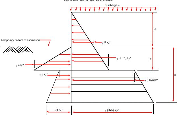
Load case 1 Soldier piles and lagging cantilevered during excavation for top row of anchors
