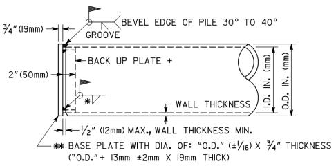
+BACK UP PLATE: TO BE CUT FROM PILE AND BENT TO FIT "I.D." TIGHTLY ALL AROUND. WELD BACK UP PLATE TO BASE PLATE.
