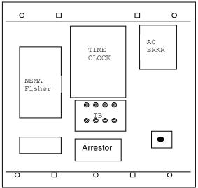
Use brackets that extend across the full width of the cabinet back on the top and bottom.
