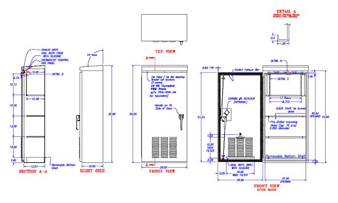
Figure 925-11 EIA Rail for Mounting Inverter or PTR inside External BBS Cabinet
