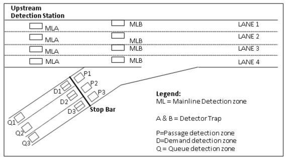
Figure 1: Typical Ramp Meter Layout
