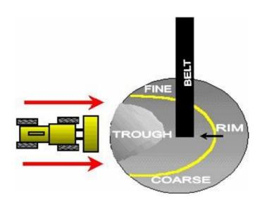
TO SHIP FROM THE PRODUCTION CONE THE LOADOUT MUST BE EQUAL TO PRODUCTION
