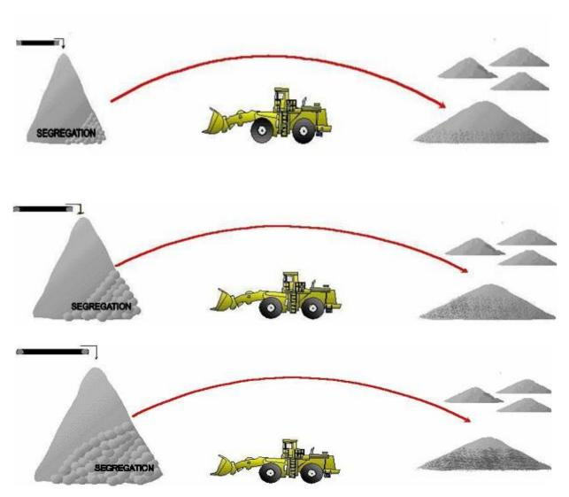
THE CONE CAN BECOME SO SEGREGATED THAT IT SIMPLY CANNOT BE RECLAIMED WITHIN SPECIFICATIONS. THIS IS PARTICULARLY TRUE WITH CLEAN STONE BECAUSE YOU CAN'T RAMP ON THE MATERIAL TO MIX LAYERS. IF YOU STOCKPILE FIVE LOADS THAT FAIL (TOO COARSE), YOU WILL SHIP FIVE LOADS THAT FAIL (TOO COARSE).
