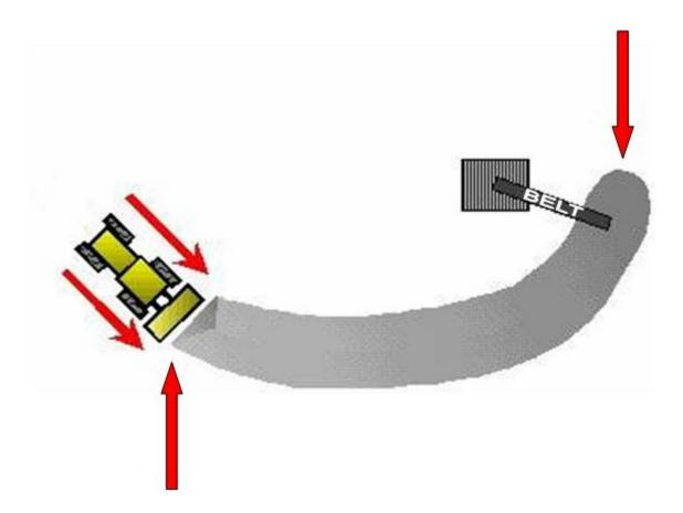
**DO** LOAD OUT OR RESTOCK FROM HERE, THE INACTIVE END
