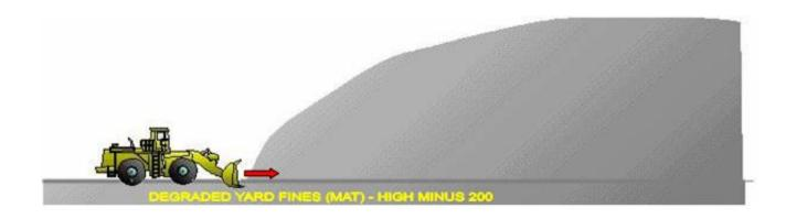
DO KEEP THE BUCKET UP AND MAKE SURE THE BUCKET IS CLEANED OUT WHEN SWAPPING FROM ONE SIZE TO ANOTHER.
