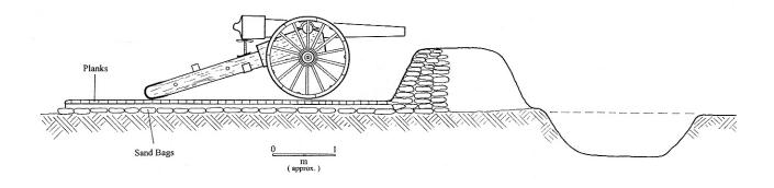
Figure 16. Idealized Cross Section of Parapet with a 30-Pounder Parrott Rifle.
