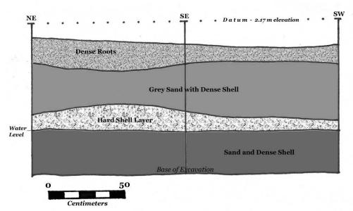
Figure 44. Profile of the East and South Walls of Test Pit #3.
