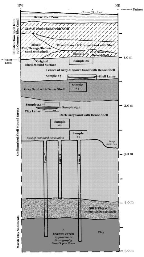
Figure 29. Profile of North Wall of Test Pit #1 showing Spoil and Shell Mound Strata, along with Core (A, B, C) and Bulk Sample (1, 2, 3, 4, 5, 6, 7) Locations.
