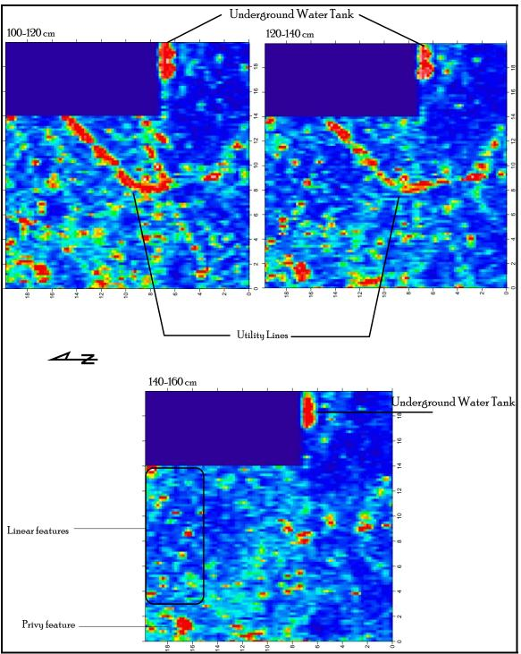
Figure 9. Super 3D composite radar image of Grids 1 and 2.
