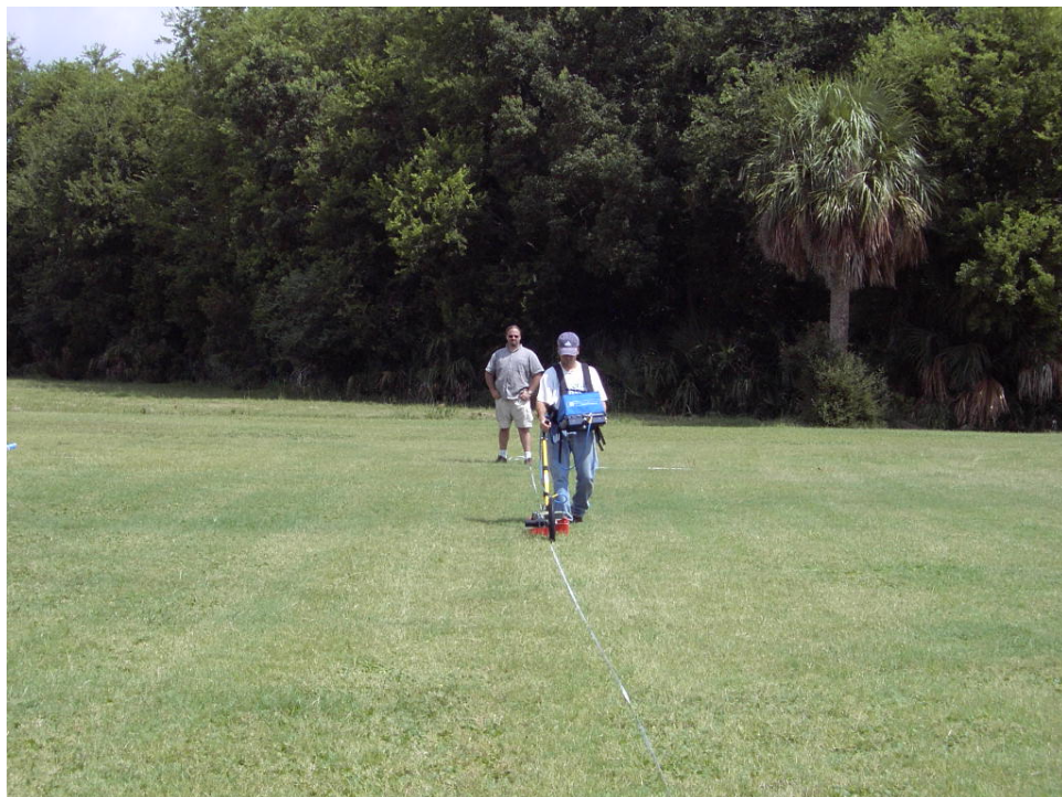
Figure 3. Collecting GPR data with a 400mhz antenna.
