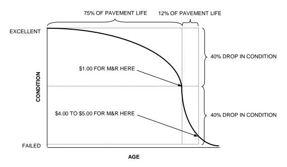
Figure 1. Pavement Condition versus Cost of Repair.
