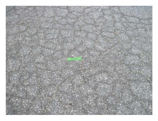
A01AY-10. Alligator Cracking and Weathering (Sample Unit #09).
