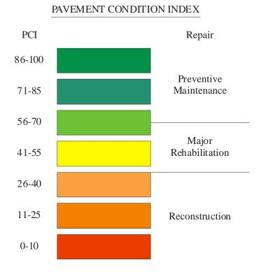
Figure 5. PCI versus repair type.
