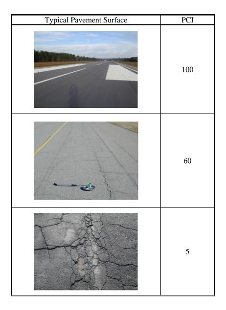
Figure 4. Visual representation of PCI scale.
