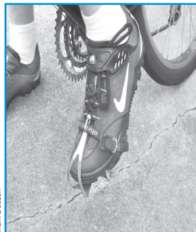
Toe clips help keep your foot secured to the pedal and provide more leverage
