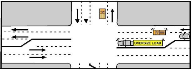
Fig. 16: Right turn at intersection - Lead escort vehicle proceeds thorough intersection to warn motorists of wide turns.
