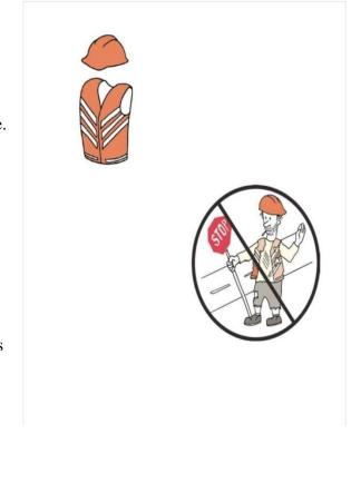
The flagger faces traffic and extends the "STOP" paddle in a stationary position extended horizontally away from the body. The free arm is extended at shoulder level with palm facing approaching traffic.
