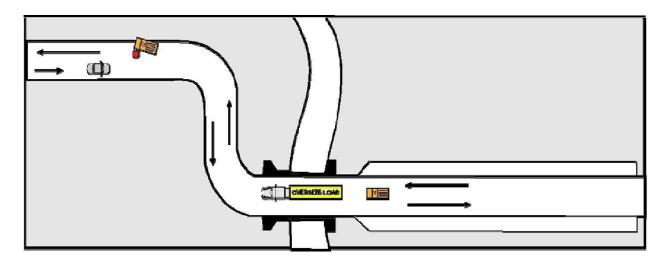
Fig. 9: Lead escort driver gives radio signal that they have traffic stopped and it is okay for permitted load to cross bridge.
