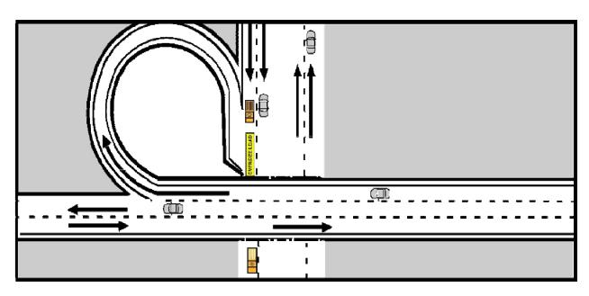
Fig. 15: Rear escort vehicle talks the permitted load driver through the traffic merger.
