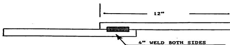
Lap Splice for Welding Re-Bar
