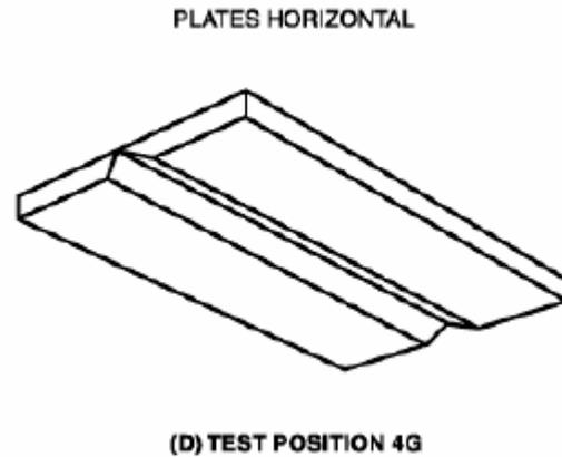
\* The backing shall be in intimate contact with the base metal.
