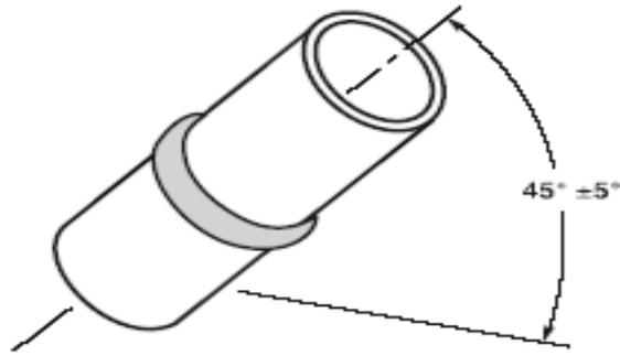
PIPE INCLINATION FIXED ( $45^{\circ} \pm 5^{\circ}$ ) AND NOT ROTATED DURING WELDING.
