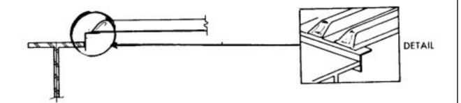
The steel forms are designed to sit flush on the steel angles, tightly enough to prevent grout from the poured concrete from seeping through to the girder below. There is no need for fiber bearing material between the steel angle and the forms.
