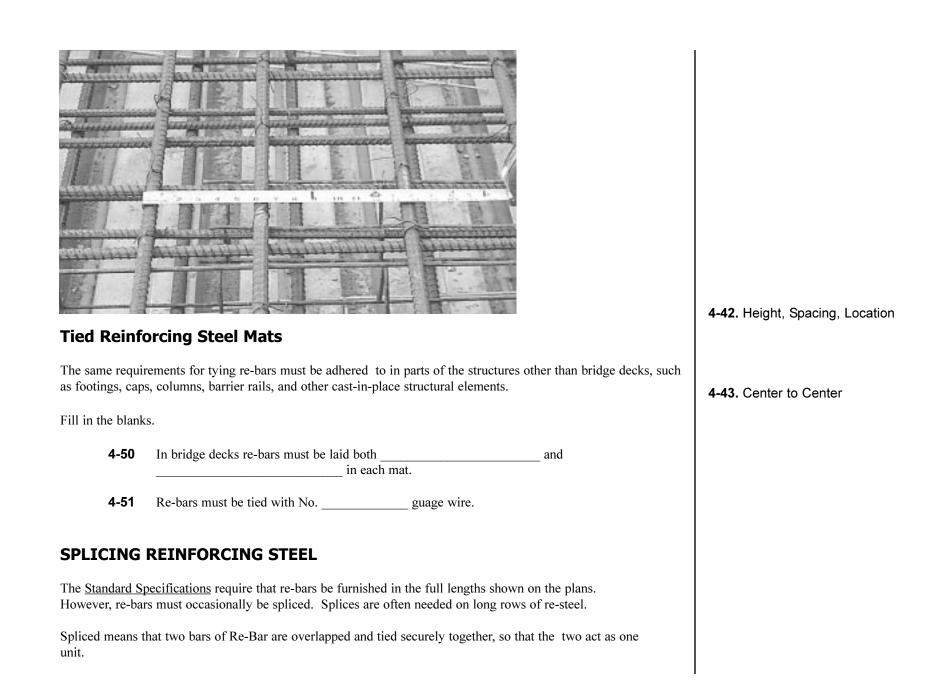
The plans will establish requirements for the amount of overlap to be used for different types of re-bars.
