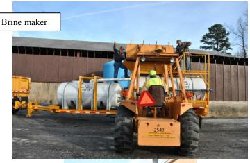
New liquid saddlebag distribution tanks controlled by dump truck driver. Truck can spread salt and stone, brine or all when needed.
