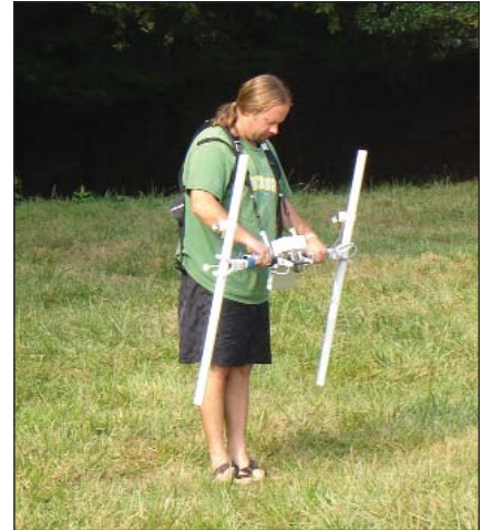
Archaeologist Jim Pomfret conducts a Gradiometer survey of a prehistoric Native American archaeological site in Bartow County, Georgia.
