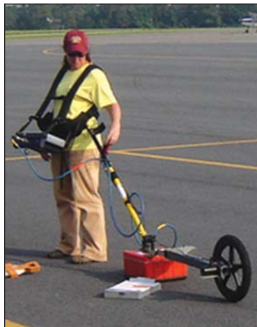
Archaeologist Sara Gale conducts a Ground-Penetrating Radar (GPR) survey at Saint Simons Island Airport in an attempt to locate subsurface voids.
