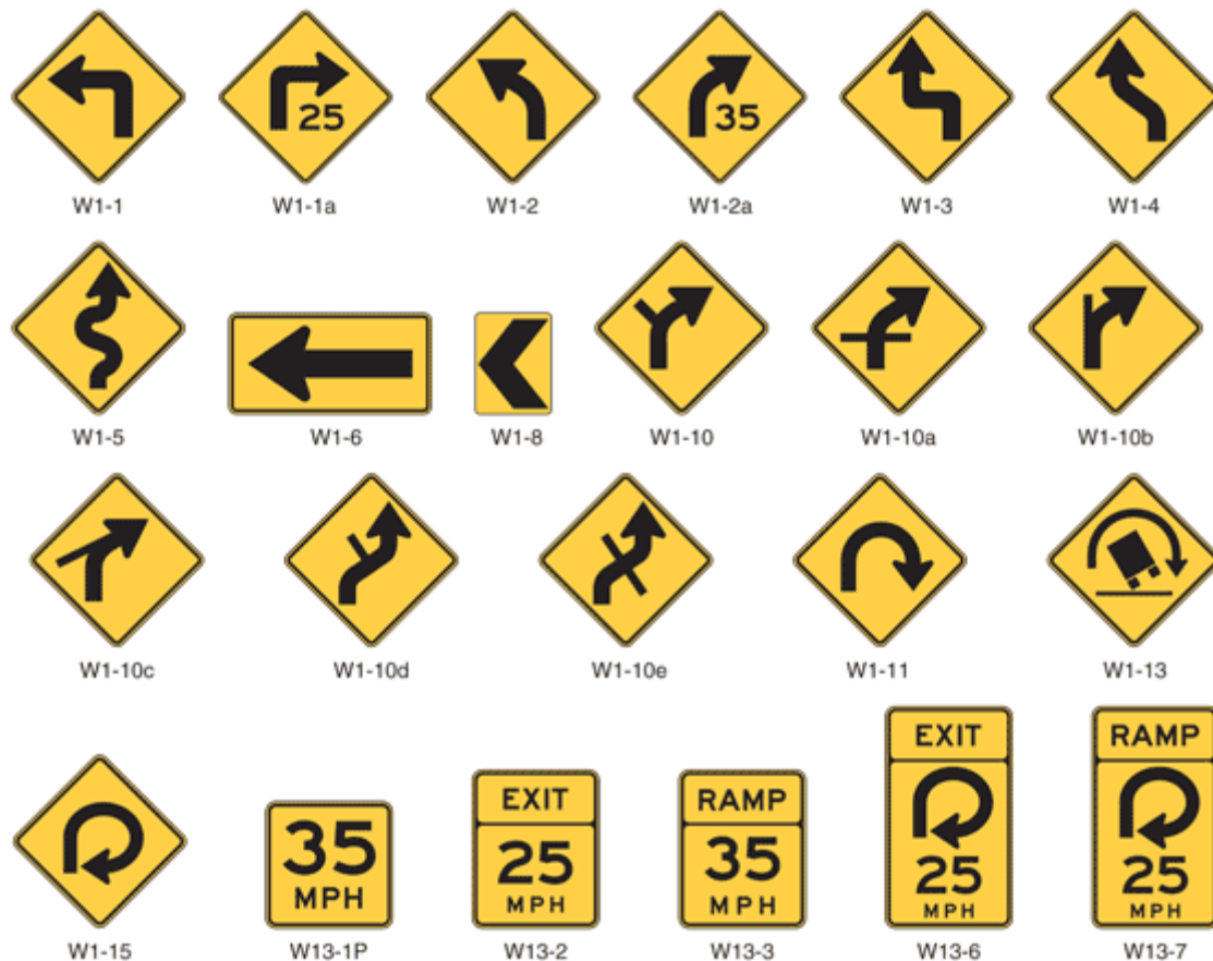
Figure 2C-1. Horizontal Alignment Signs and Plaques
