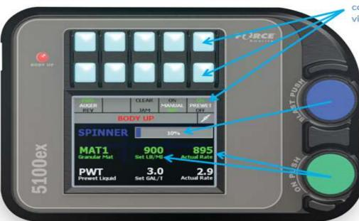
The 5100EX screen is a touch screen used for selecting Menu items, making selections on sub menus and adjusting values on sub menus.
