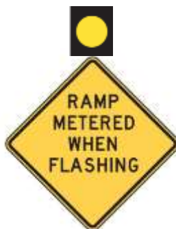
Figure 4-6: Ramp Metered When Flashing Sign (W3-8) with Flashing Beacon
