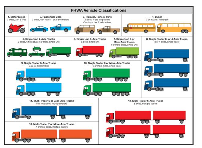
Figure 6.1. FHWA Truck Vehicle Classification Scheme
