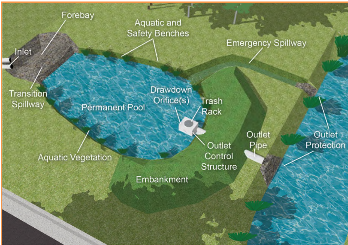
Figure 5.7-2 Typical Wet Detention Pond Configuration and Components
