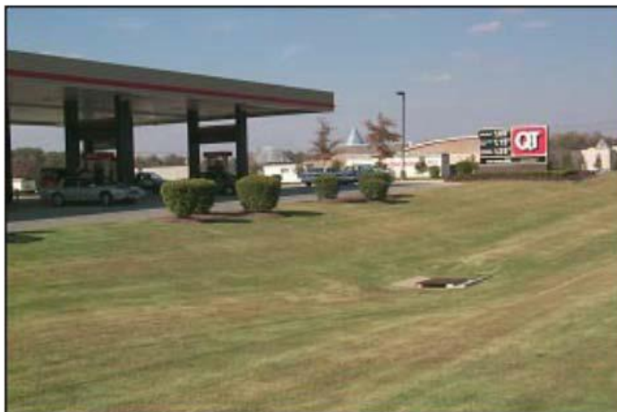
Figure 3.3 - Typical post-construction BMP - grass filter strip (3-5)
