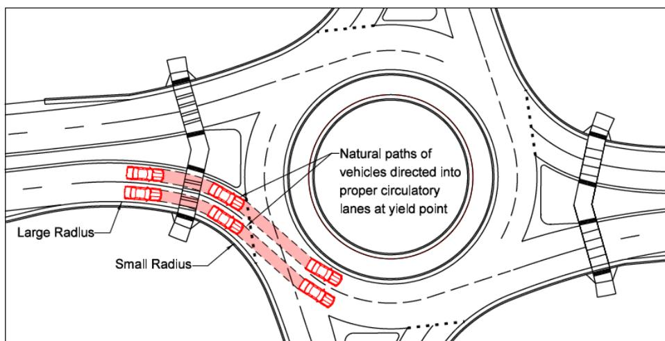
**Figure 3-30. Multilane Entry Design to Minimize Path Overlap**
