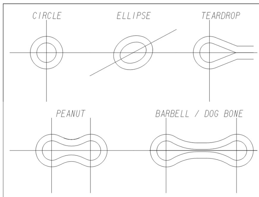
Figure 3-7. Roundabout Shapes
