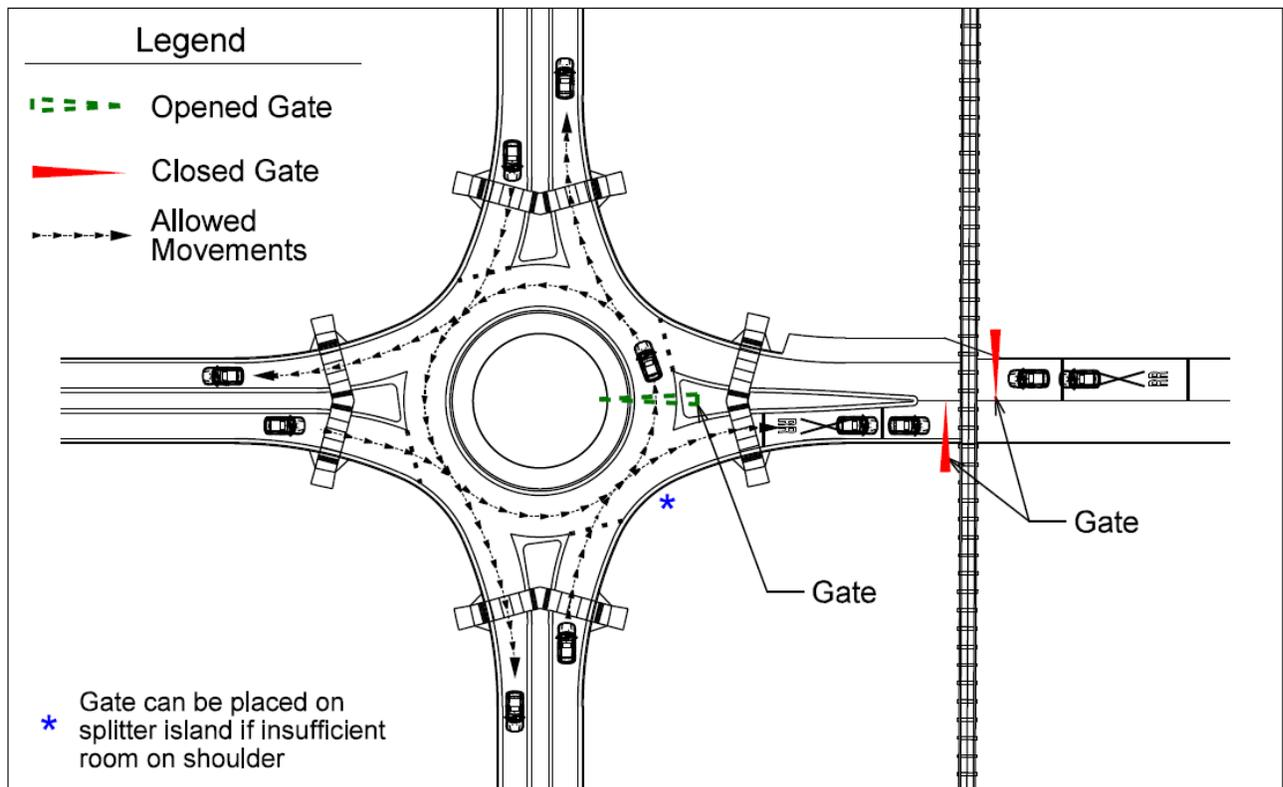
**Figure 6-2C. Track hold stage with gated closure at railroad crossing only**
