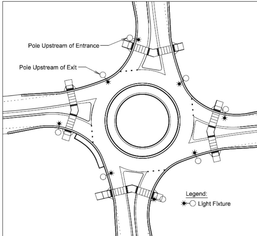
Figure 7-1. Perimeter Pole Placement
