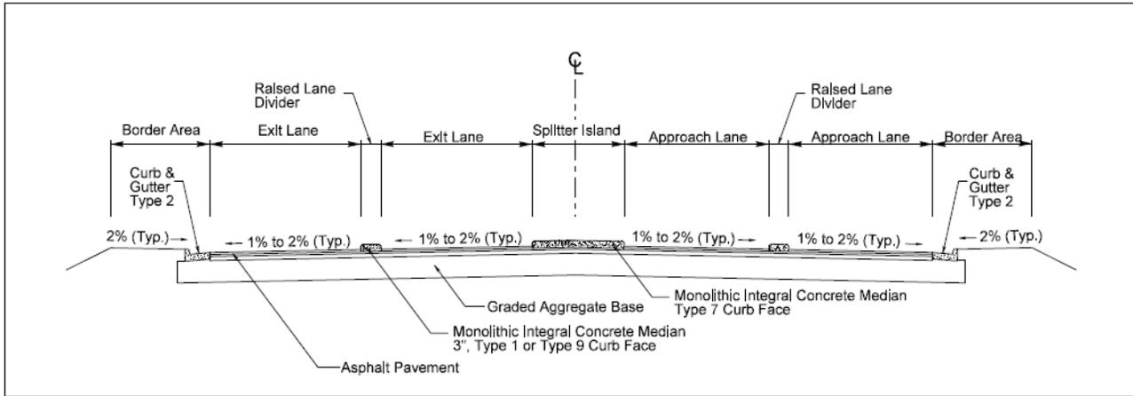
**Figure 3-43. Case 3 Multilane Roundabout Approach/Departure Typical Section**
