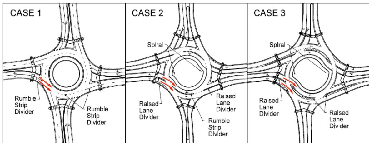
**Figure 1-2. Multilane Roundabout Key Features**
