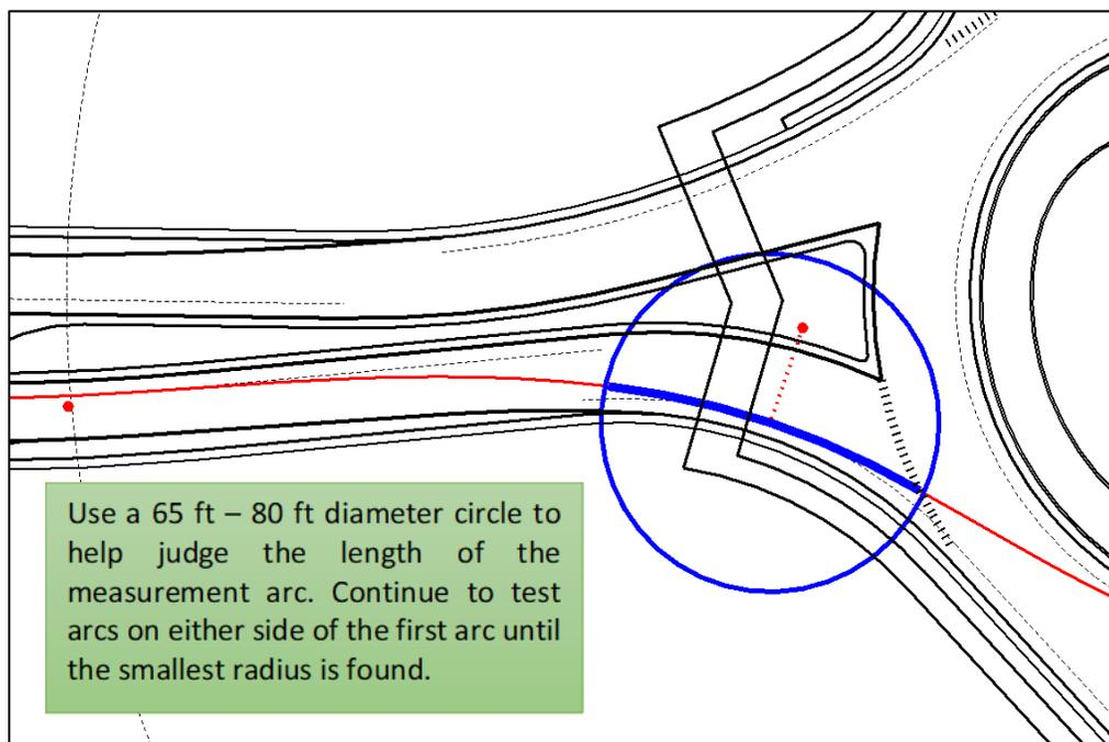
**Figure D-3. Measuring Critical Spline Radius**
