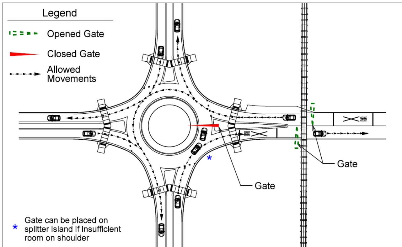
Figure 6-2A. Track clearance stage with gated closure for circulating flow
