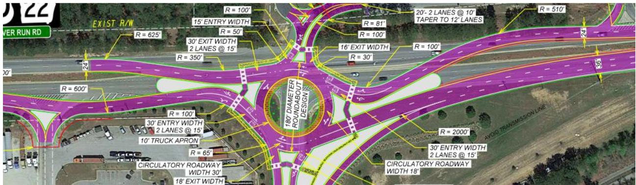
Figure A-4. Original Roundabout Design
