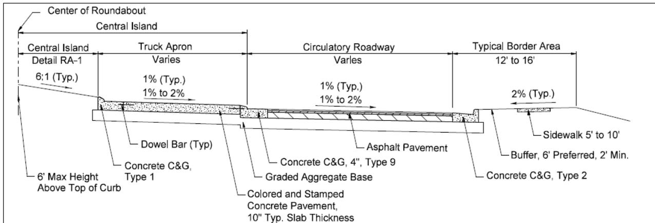
**Figure 3-38B. Roundabout Detailed Section**
