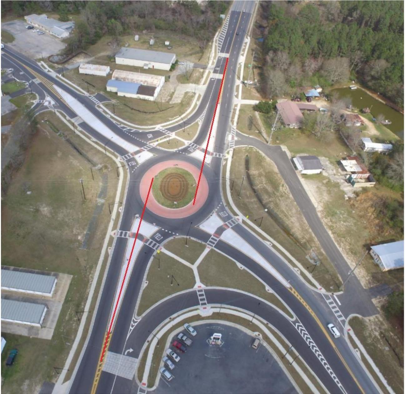
Figure A-3. Offset Left Design Example
