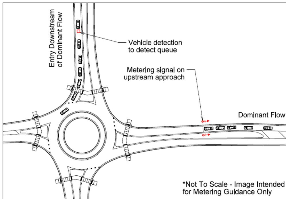
**Figure 5-8. Roundabout with Signalized-Meter Approach**
