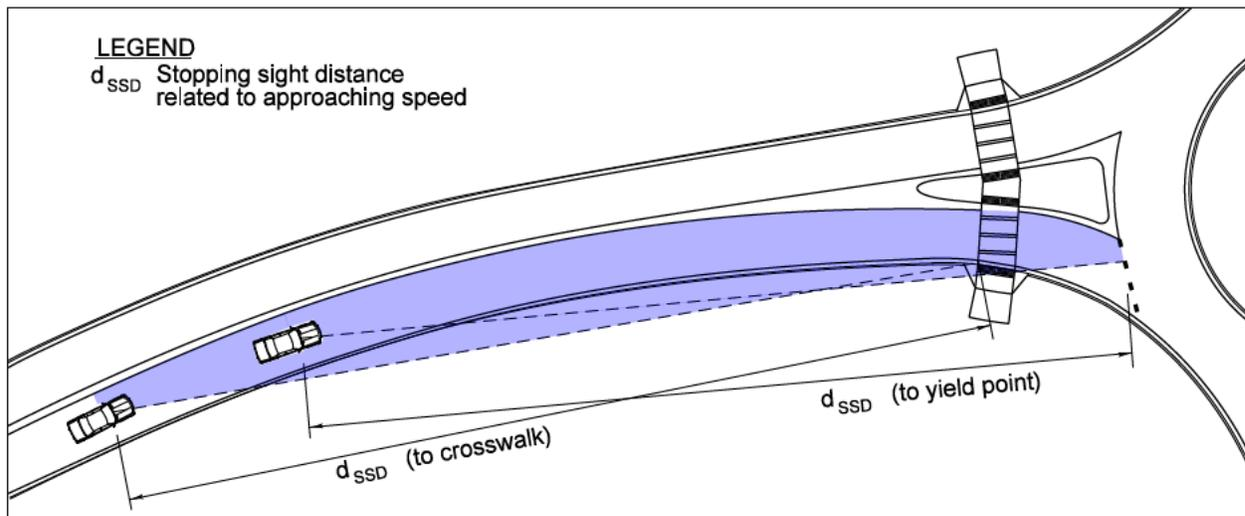
Figure 3-18. Approach Stopping Sight Distance (SSD)
