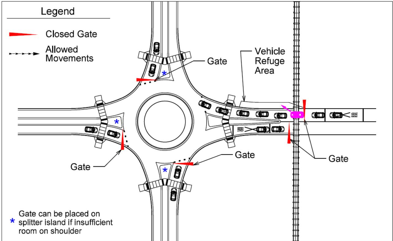
**Figure 6-3B. Pre-empt hold stage with gated closures at approach entries and railroad crossing**
