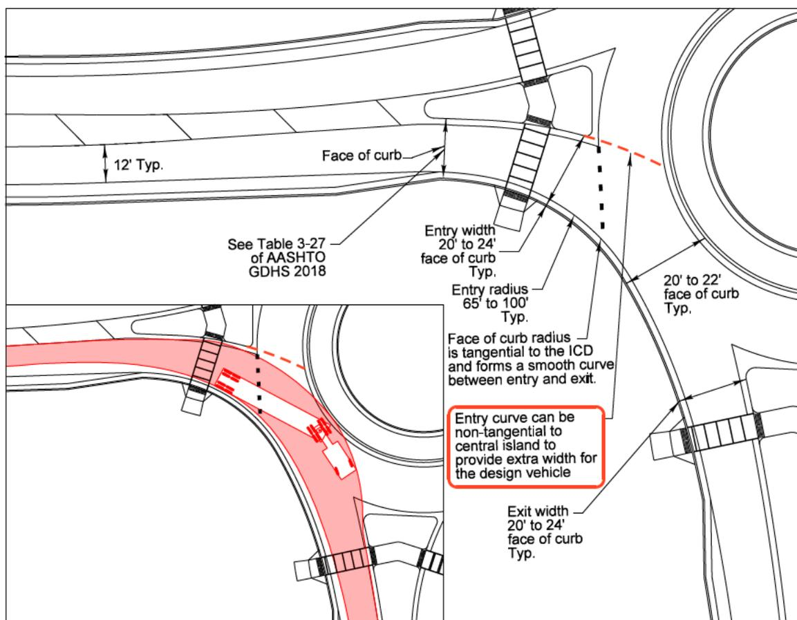
**Figure 3-11. Example of Typical Entry to Exit Curves**
