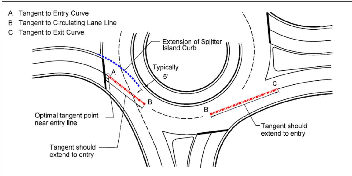
**Figure 3-31. Method for Checking Path Overlap (Case 1)**
