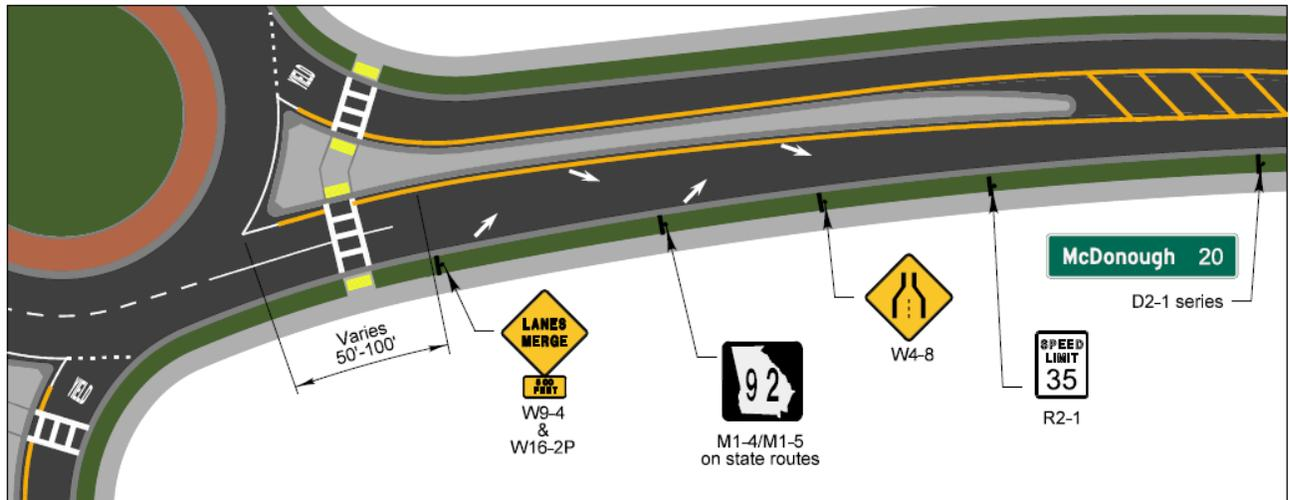
**Figure 5-6. Lane Drop Multilane Roundabout Signing and Marking**
