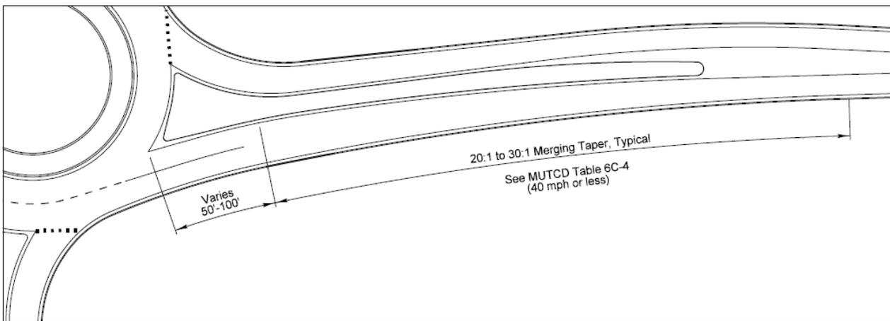
**Figure 3-9b. High-Speed Multilane Exit Design**
