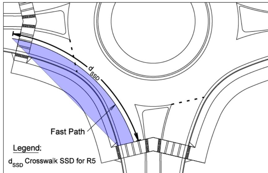
Figure D-7. SSD to Crosswalk on Exit
