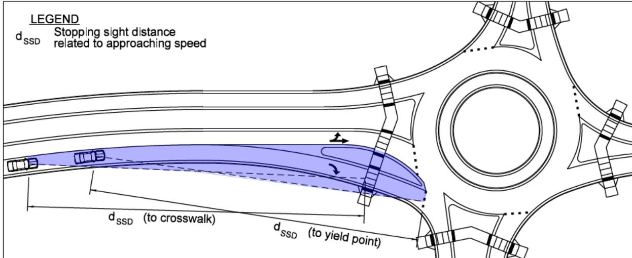
Figure 3-20. Approach SSD (with Bypass Lane)
