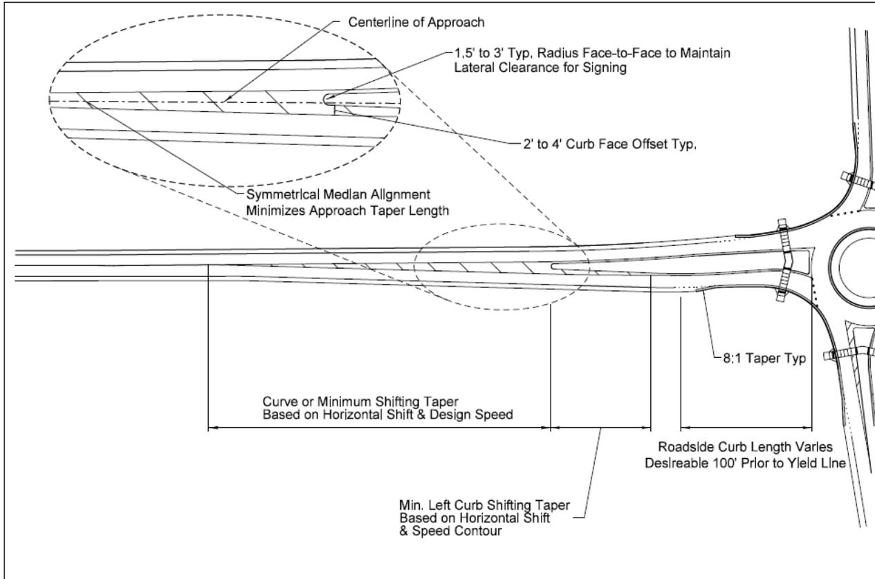
**Figure 3-9a. High-Speed Approach Design**
