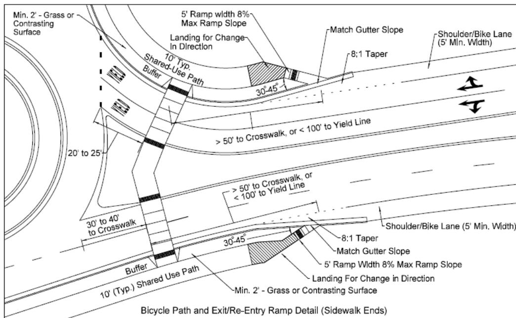
Figure 4-3. Bicycle Path Exit and Entry without Extended Sidewalk
