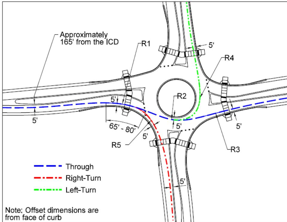
Figure 3-12. Determination of Entry Path Curvature – Mini-Roundabouts
