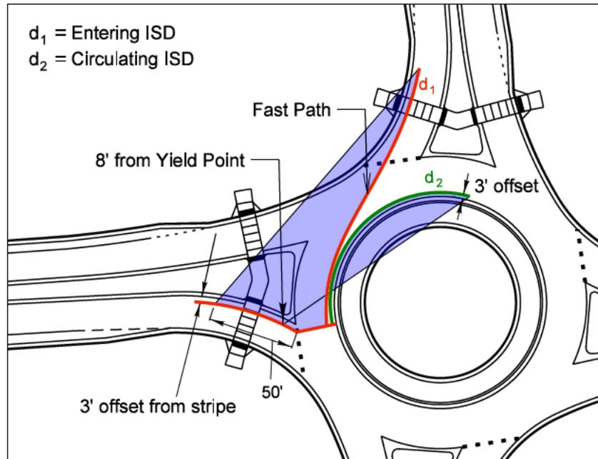
Figure D-9. Entering and Circulating ISD
