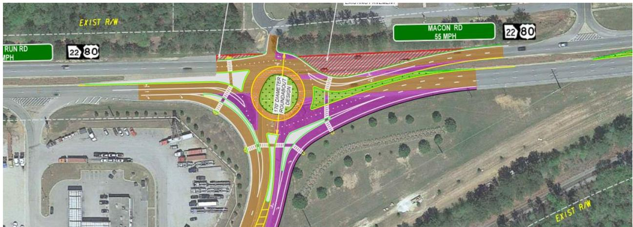
Figure A-5. Refined Roundabout Design
