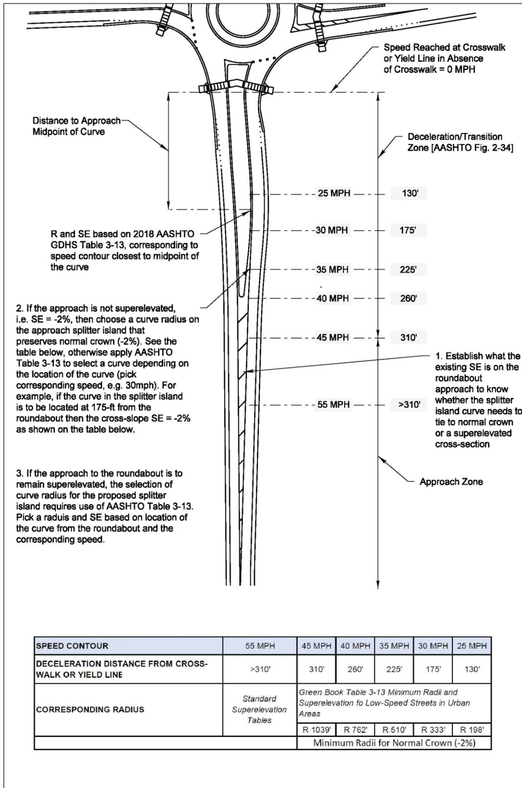
Figure 3-10. Superelevation on Approach
