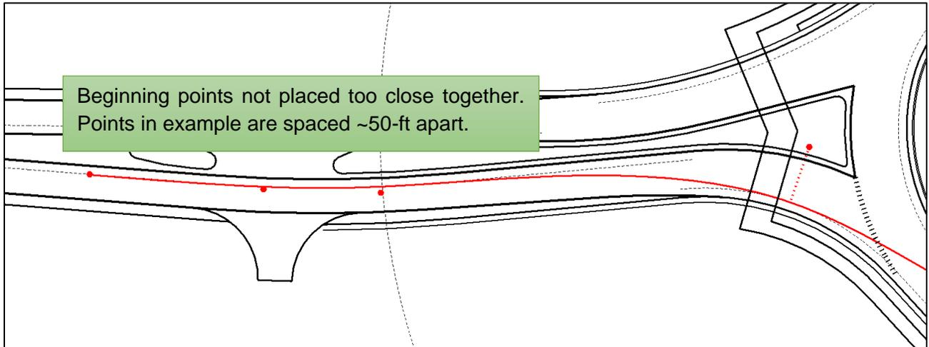
**Figure D-1. Control Points on Approach**
