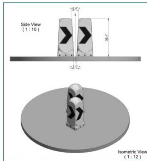
**Figure 3-46. Additional Detail of Bollard Configuration**
