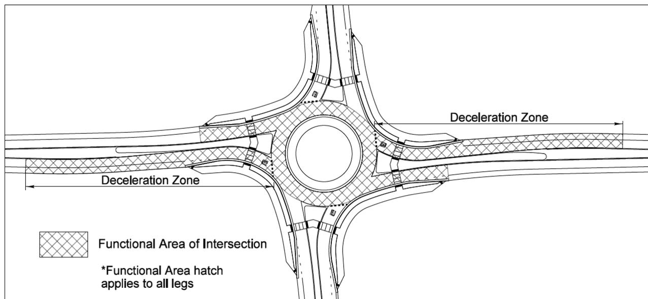
**Figure 3-2. Roundabout Functional Area**
