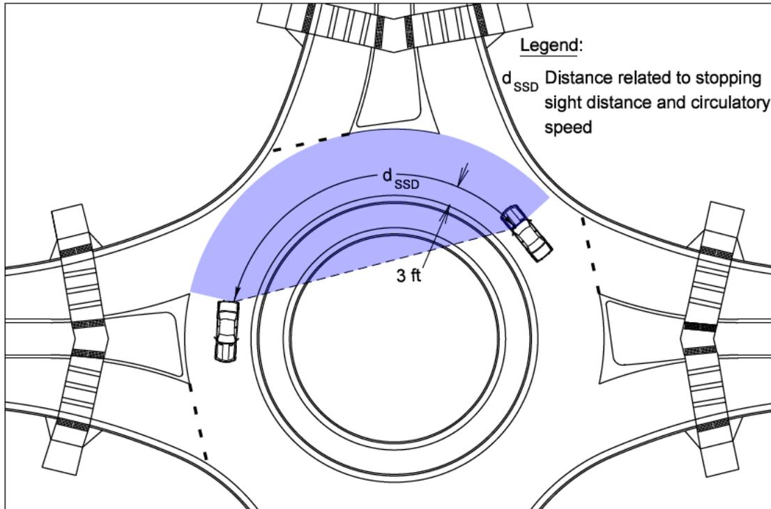
**Figure 3-22. Stopping Sight Distance around the Circulatory Roadway**
