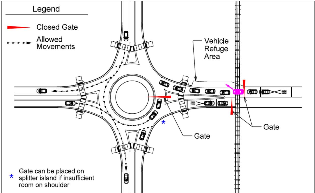
**Figure 6-2B. Track clearance stage with gated closure for circulating flow and at track crossing**
