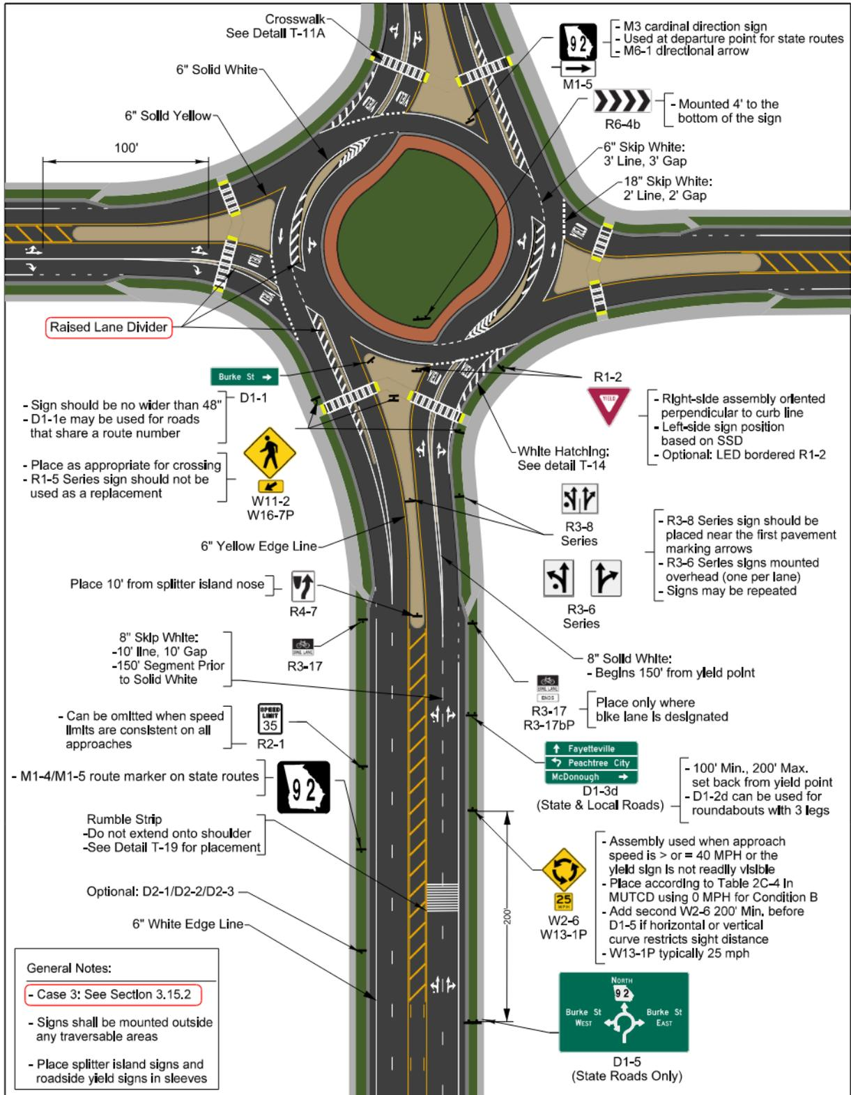
Figure 5-5. Case 3 Multilane Roundabout (1x2) Signing and Marking
