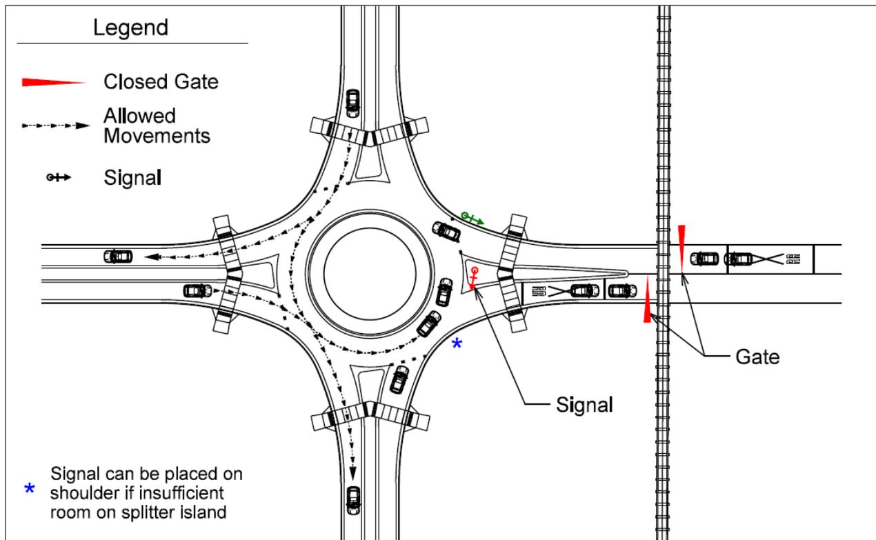
Figure 6-5. Signal at roundabout with gate at railroad crossing
