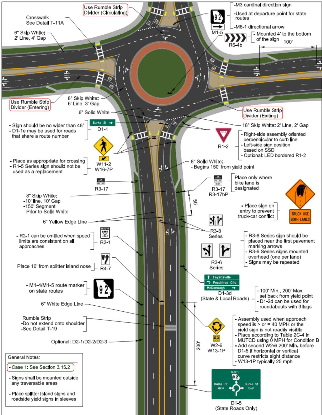
Figure 5-3. Case 1 Multilane Roundabout Signing and Marking
