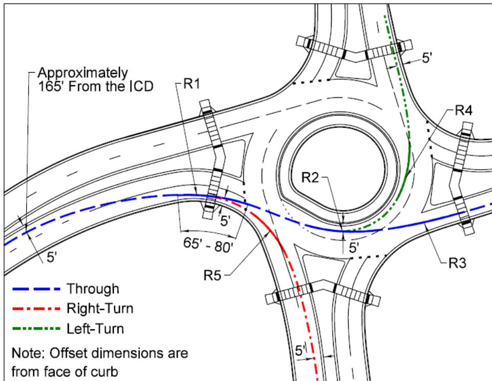
Figure 3-15. Determination of Entry Path Curvature – Multilane Roundabouts Case 1
