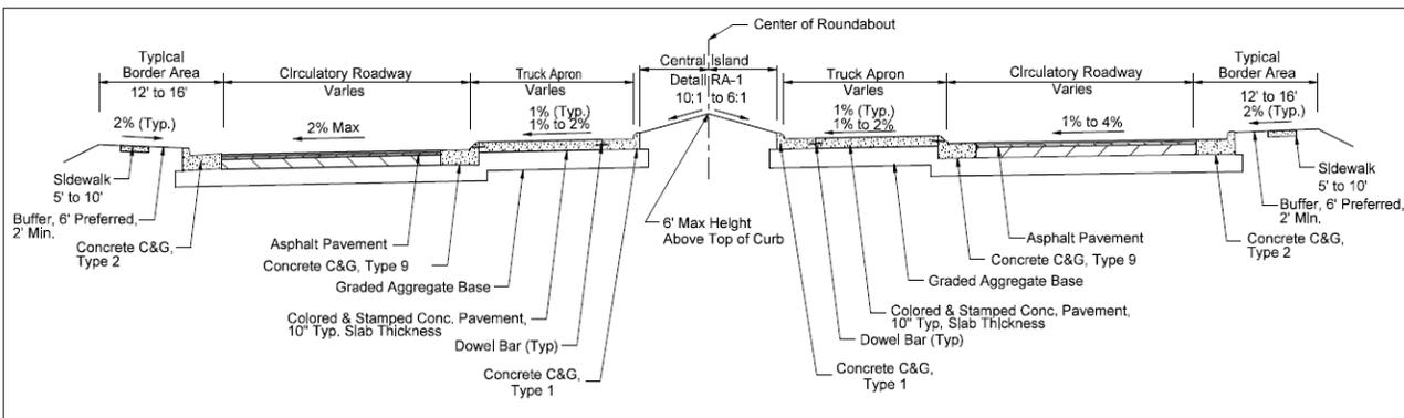
Figure 3-39B. Roundabout with Tipped Circle Section (Truck Apron Sloped In)
