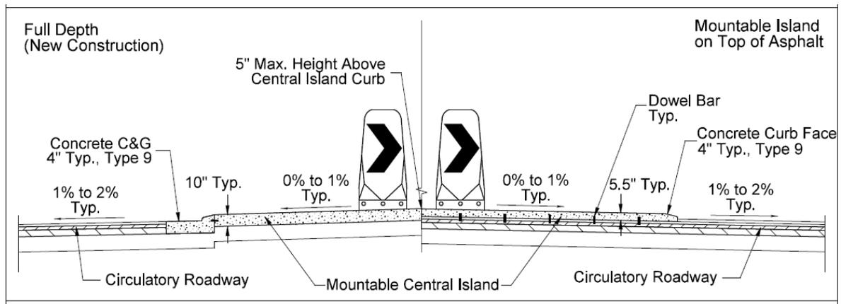
**Figure 3-45. Mountable Apron at Mini-Roundabouts, shown with Bollards**
