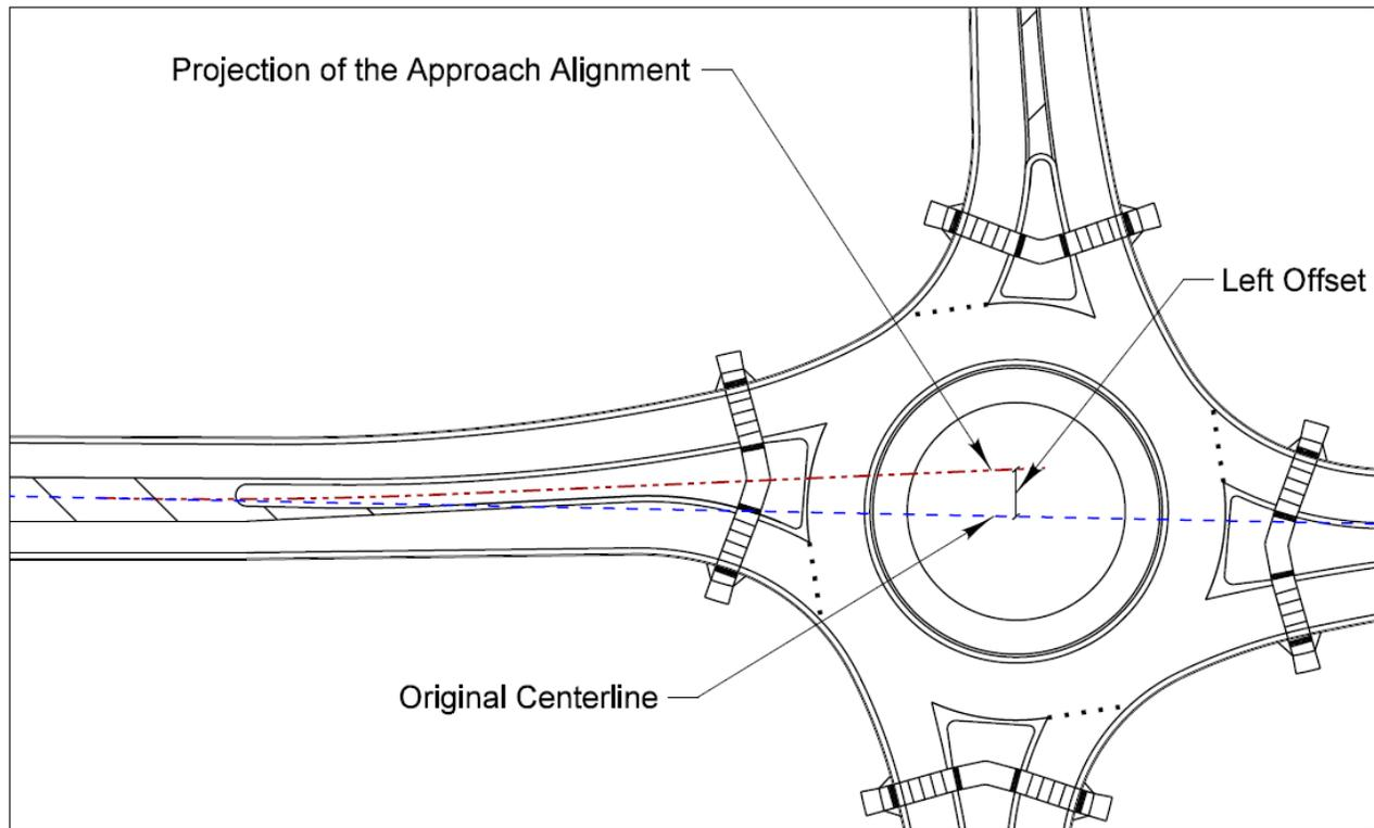
**Figure 3-8. Left Offset Design for Entry Deflection**
