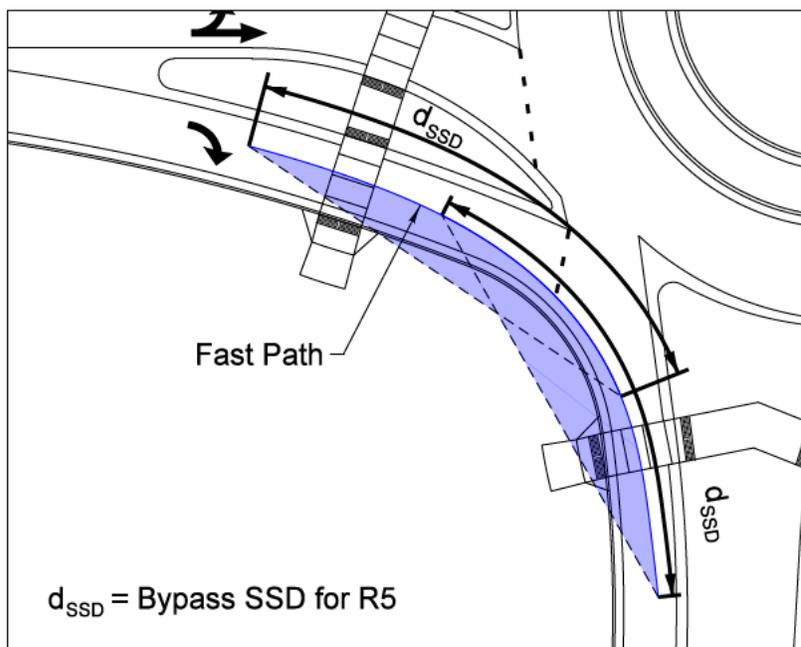
Figure D-6. Approach SSD for Free-Flow Right Turn Bypasses
