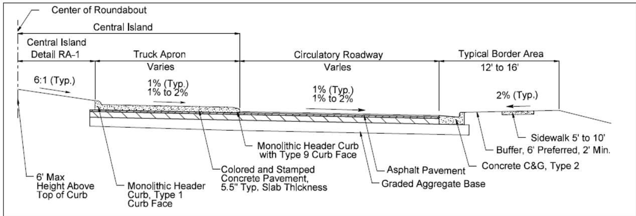
**Figure 3-38A. Roundabout Detailed Section with Monolithic Truck Apron**
