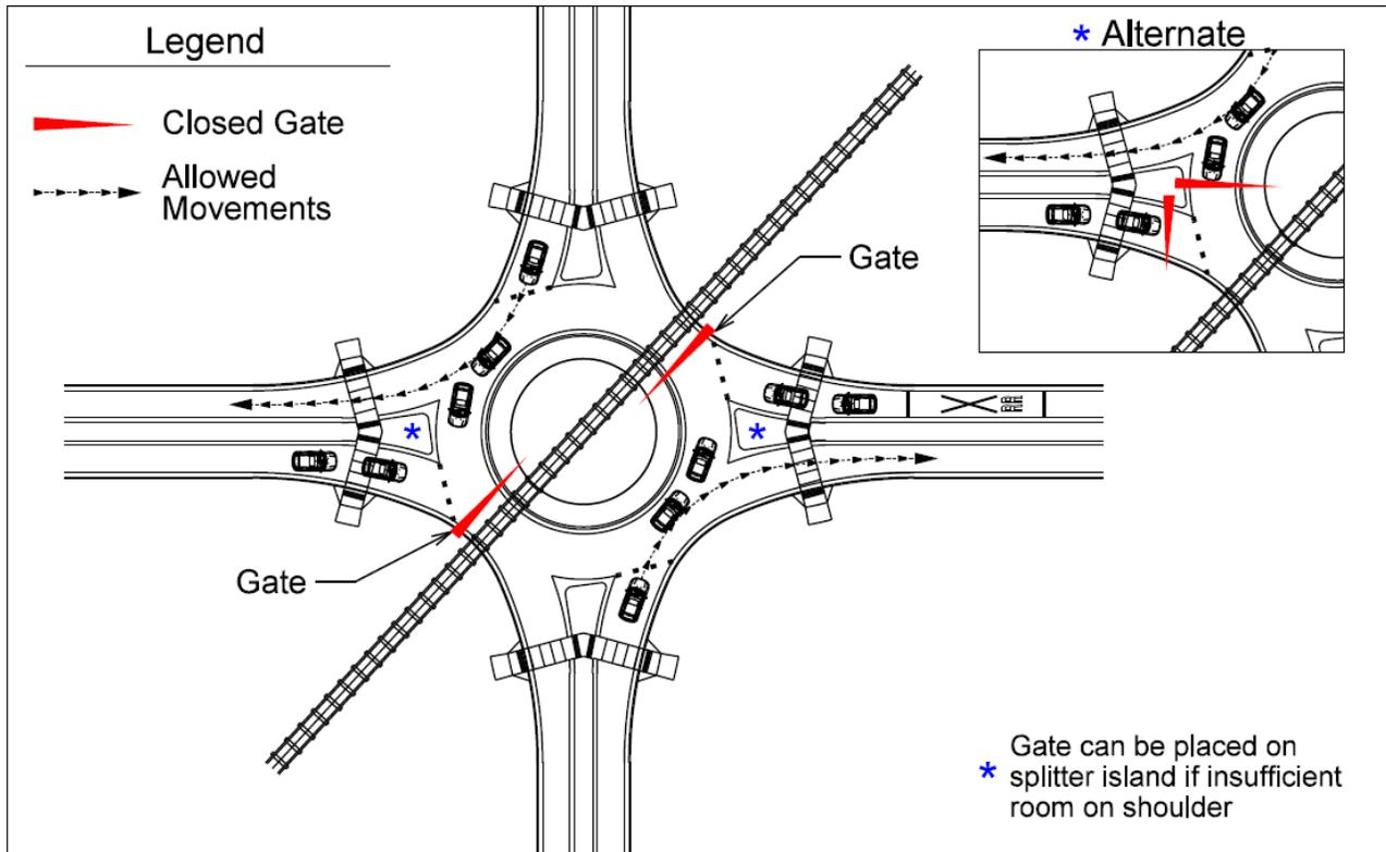
Figure 6-4. Railroad through the roundabout
