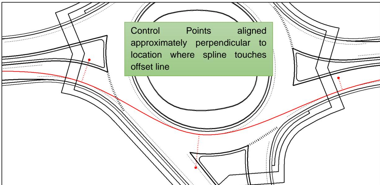
**Figure D-2. Control Points Entry, Circulating, Exiting**
