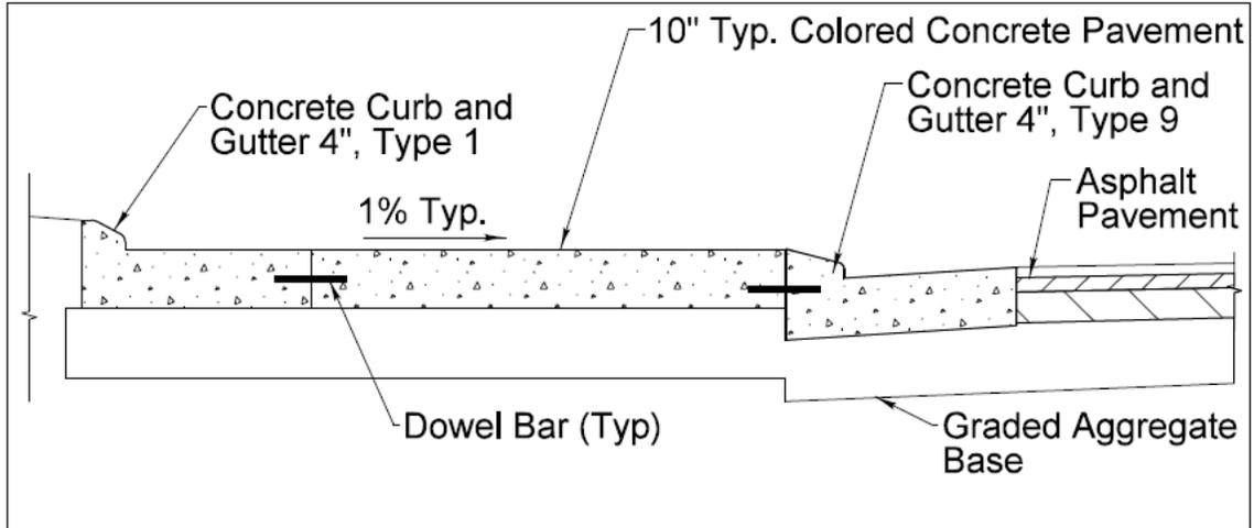
Figure 3-40B. Outside Truck Apron Typical Section
