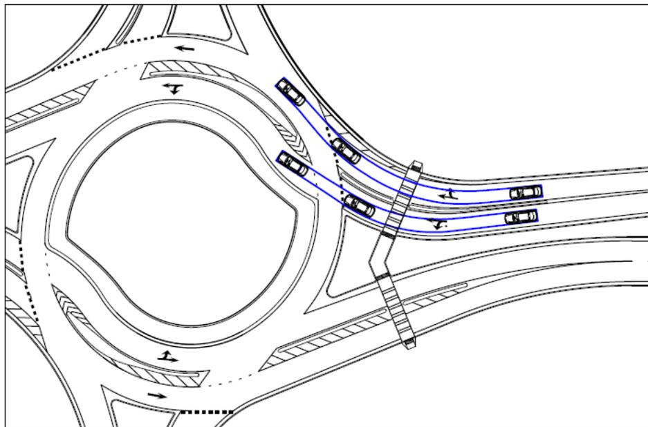
**Figure 3-33. Case 3 Multilane Roundabout Entry Path Alignment**
