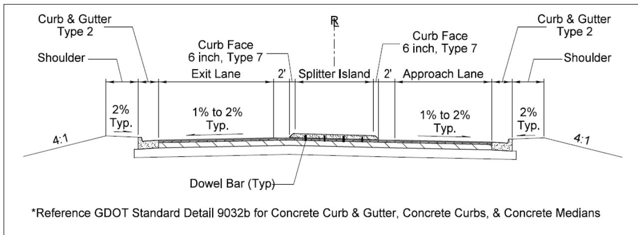
**Figure 3-37A. Roundabout Approach Typical Section with Monolithic Splitter Island**
