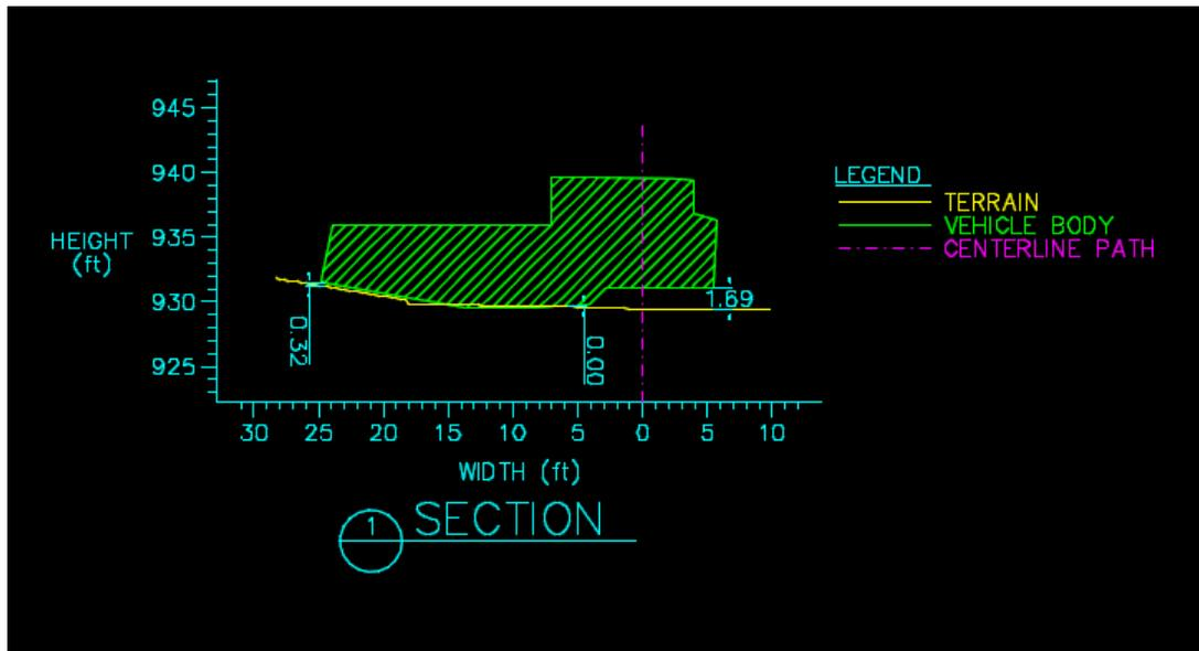
Figure D-12. Vertical Check Punch Through Example
