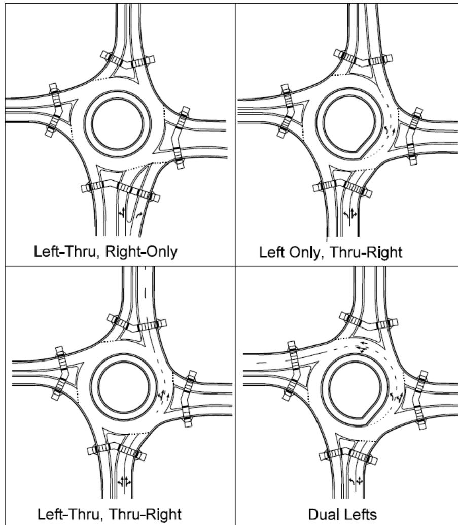
**Figure 2-1. Lane Configuration Options for Two-lane Entry**
