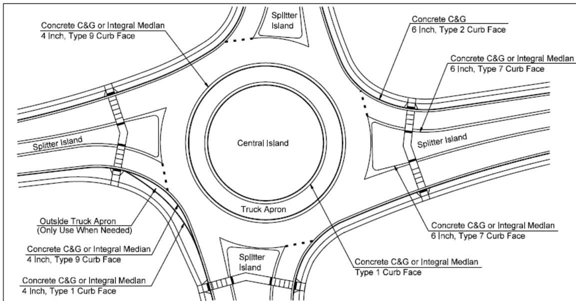
Figure 3-36. Curb Types Within the Roundabout
