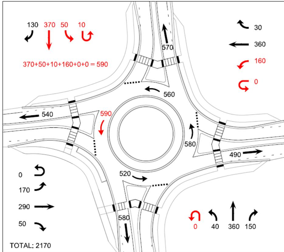
Figure 9-1. Circulating Volume Calculation
