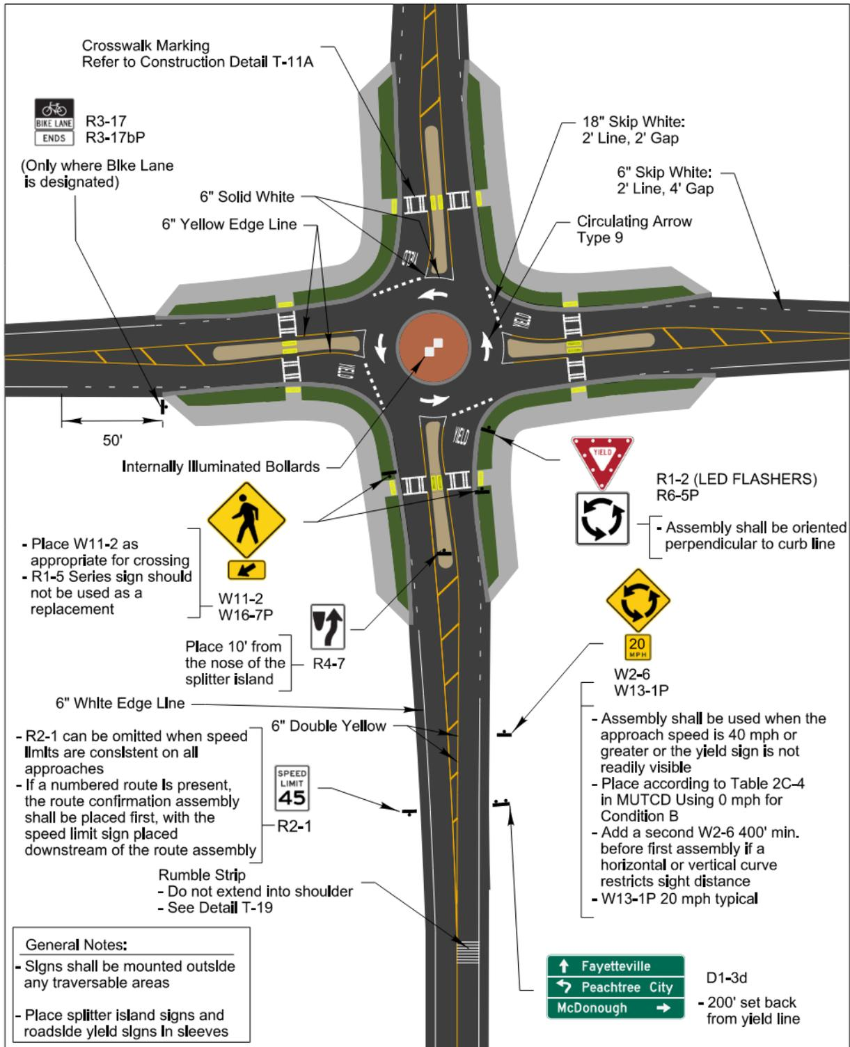
Figure 5-1. Mini-Roundabout Signing and Marking
