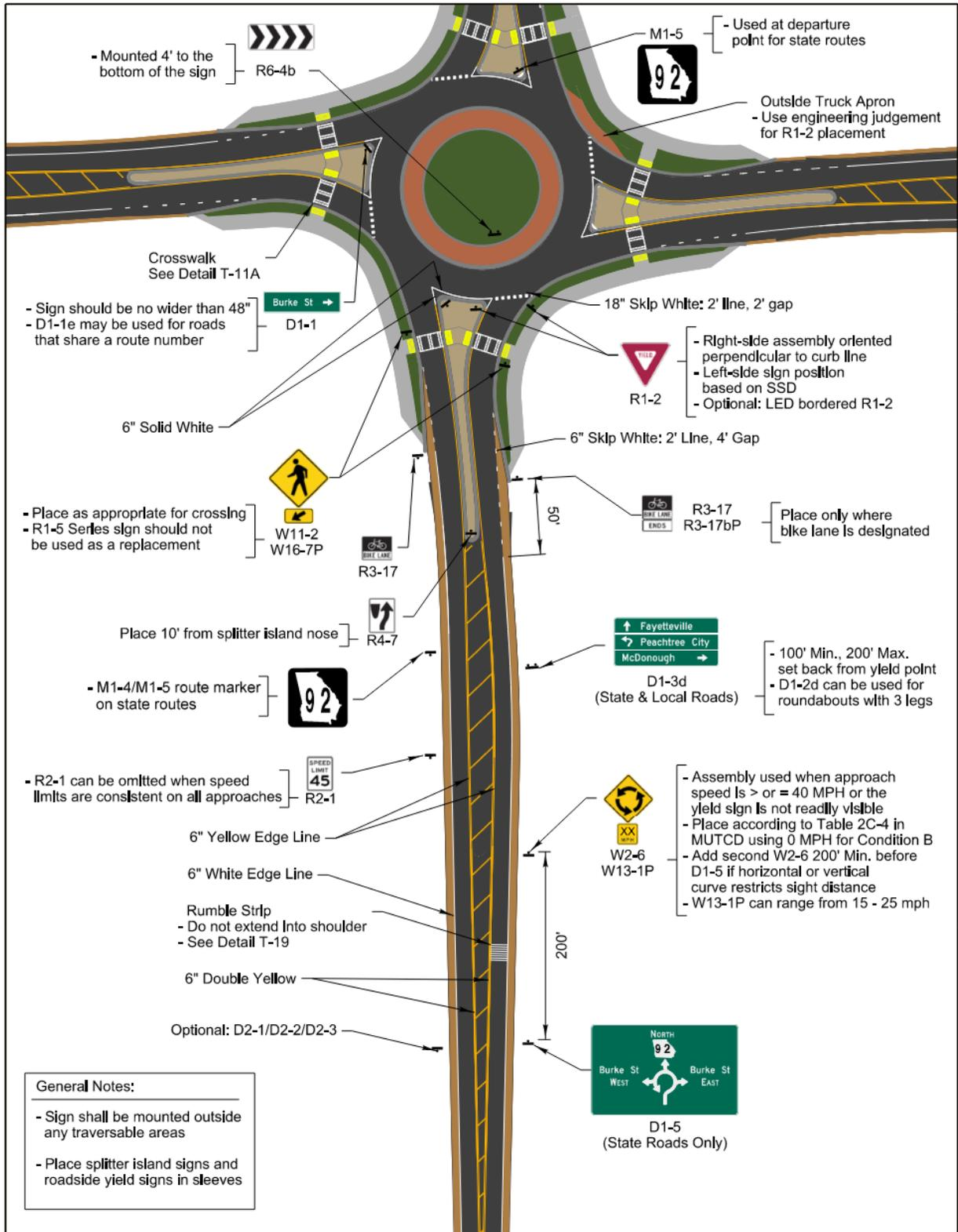
Figure 5-2. Single Lane Roundabout Signing and Marking
