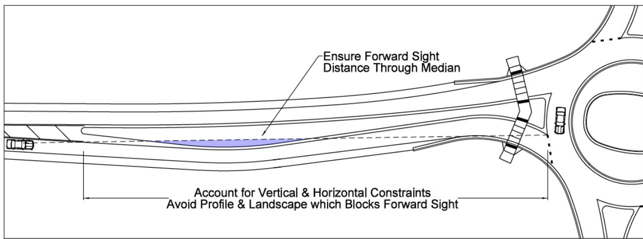
Figure 3-19. Approach SSD (with Reverse Curves)
