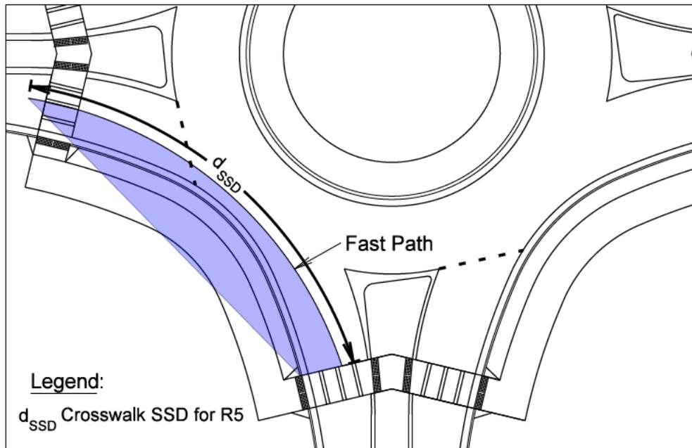
Figure 3-21. Stopping Sight Distance to the Downstream Crosswalk
