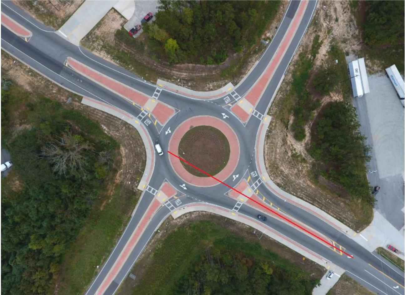
Figure A-2. Offset Left Design Example
