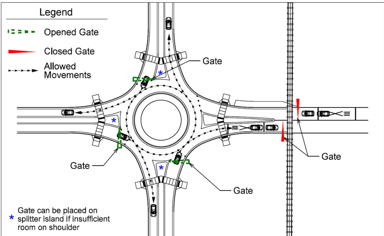
**Figure 6-3C. Track hold stage with gated closures at railroad crossing only**
