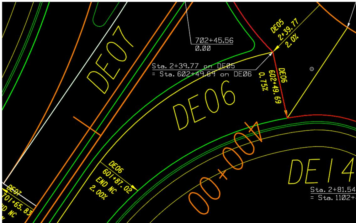
**Figure F-7. Cross Slope Transition at Entry or Exit Tie-in**
