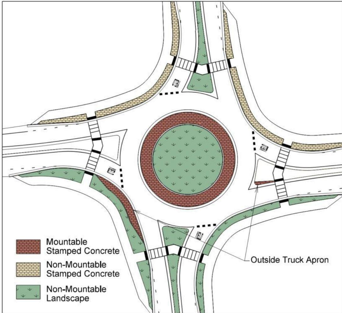
**Figure 8-6. Truck Apron Coloring & Patterning**
