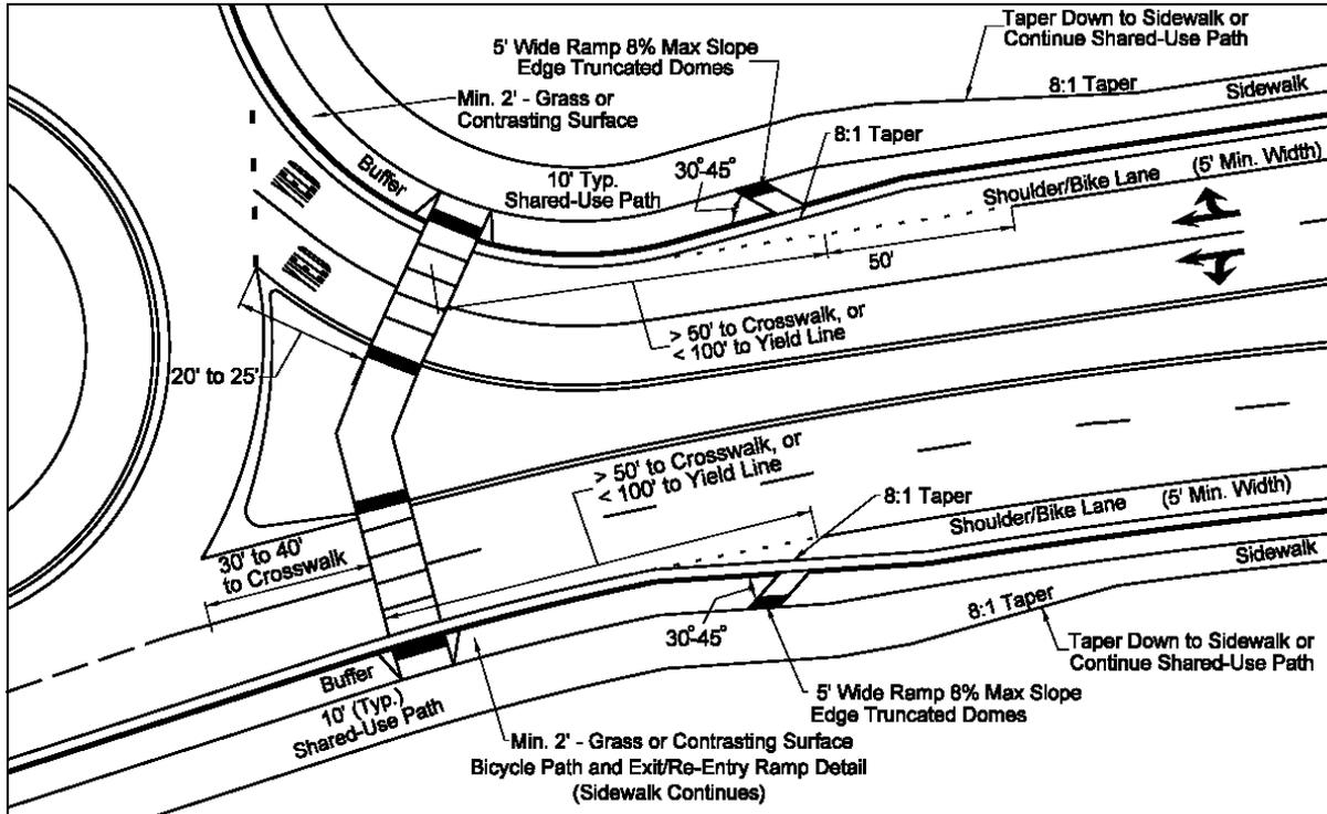
Figure 4-4. Bicycle Path Exit and Entry with Extended Sidewalk
