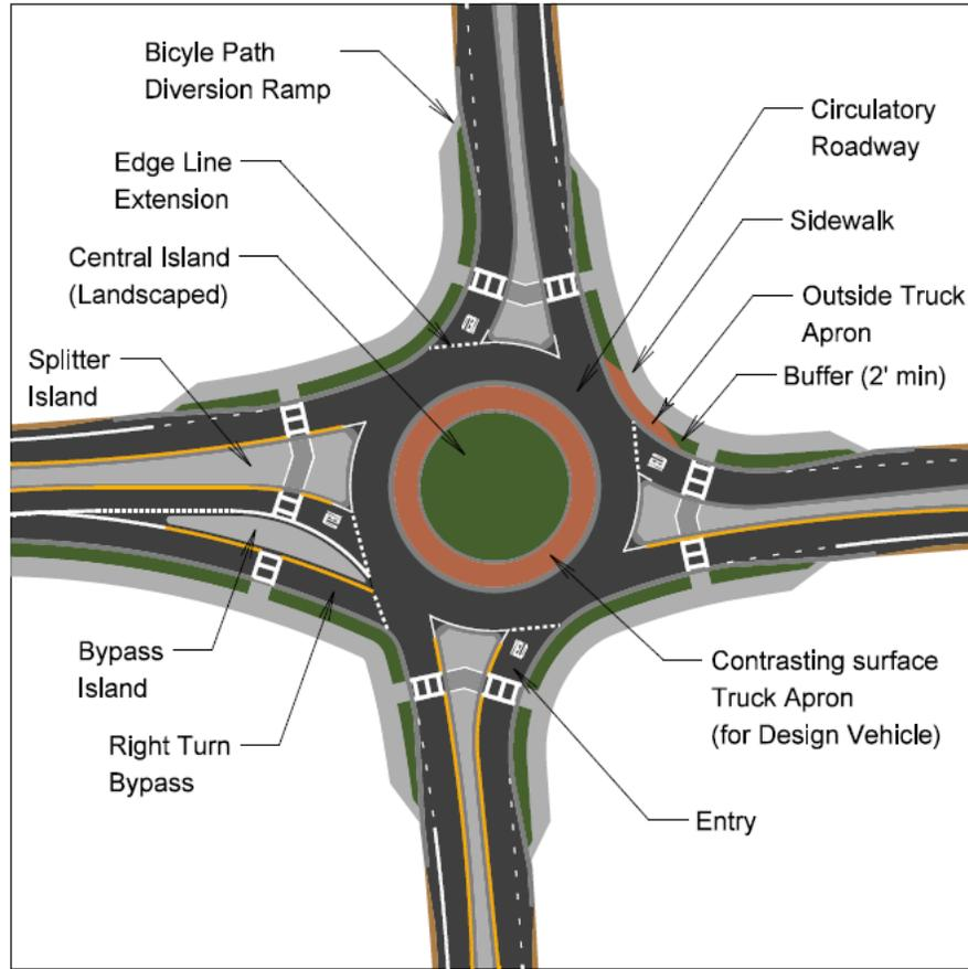
**Figure 1-1. Key Roundabout Features**
