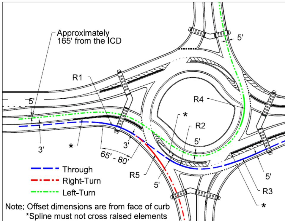
Figure 3-17. Determination of Entry Path Curvature – Multilane Roundabouts Case 3
