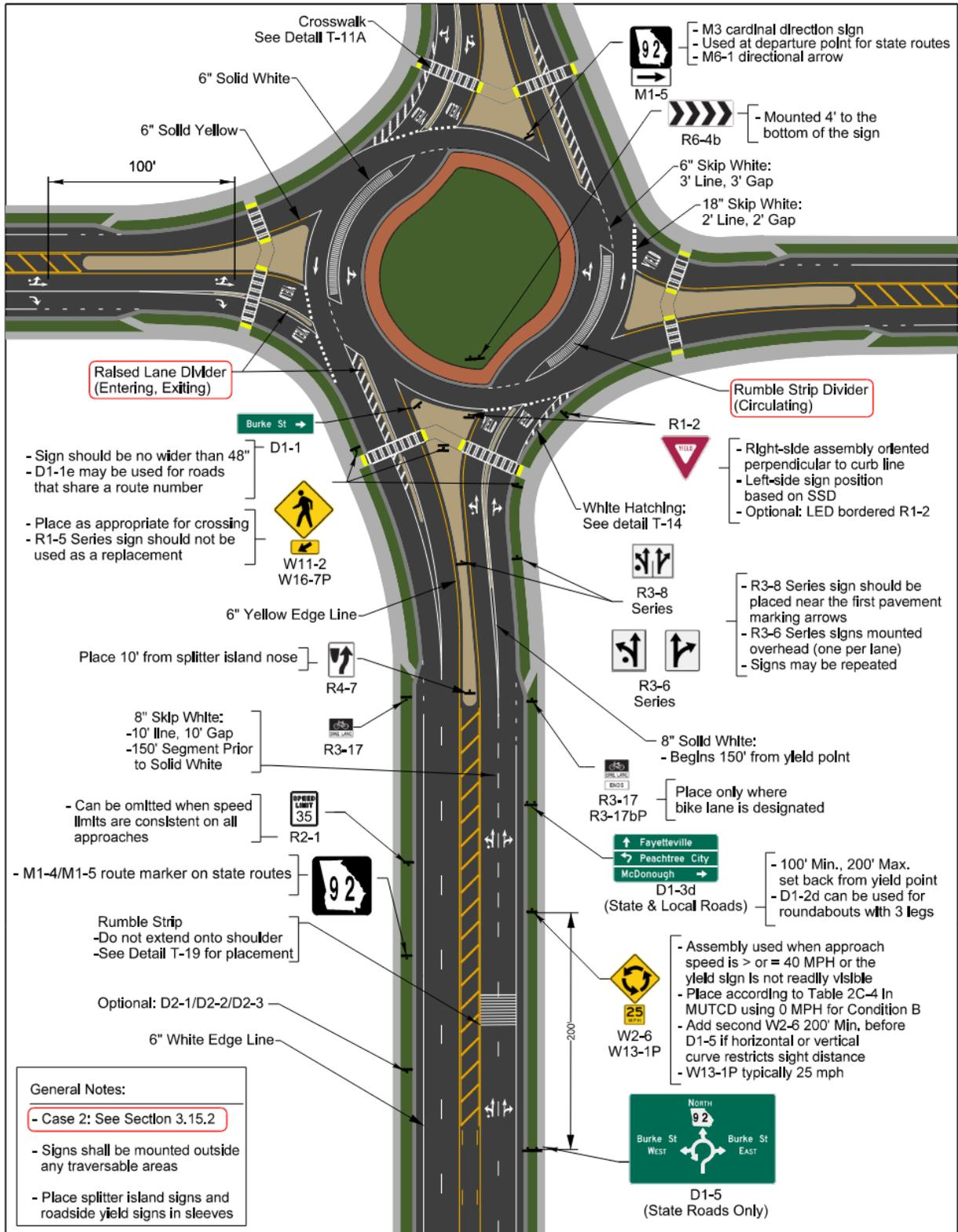
Figure 5-4. Case 2 Multilane Roundabout Signing and Marking
