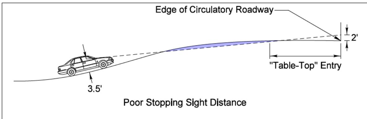
**Figure 3-23. Vertical Considerations of Approach Stopping Sight Distance**
