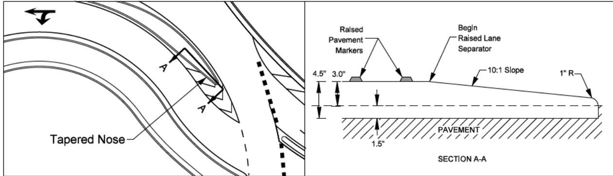
Figure 3-41. Tapered Nose Detail (Frog)
