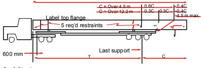
$\begin{array}{l} \text{C} = 0.2 \text{L} \text{ min.} \\ \text{C} = 0.3 \text{L} \text{ max.} \end{array}$
