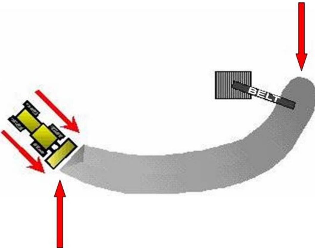
**DO** LOAD OUT OR RESTOCK FROM HERE, THE INACTIVE END
