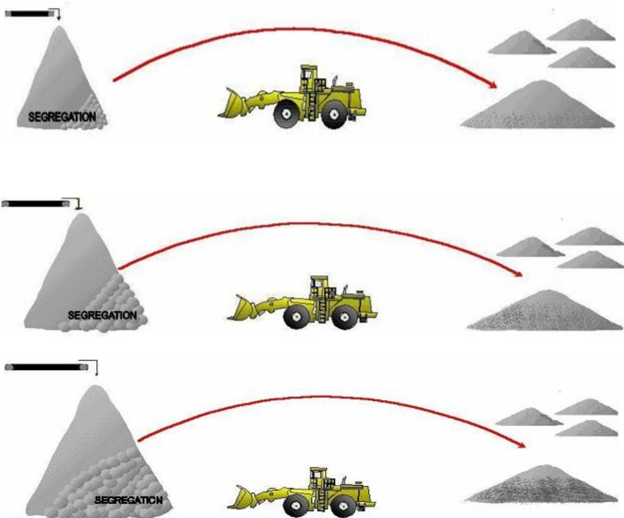
**THE CONE CAN BECOME SO SEGREGATED THAT IT SIMPLY CANNOT BE RECLAIMED WITHIN SPECIFICATIONS. THIS IS PARTICULARLY TRUE WITH CLEAN STONE BECAUSE YOU CAN'T RAMP ON THE MATERIAL TO MIX LAYERS. IF YOU STOCKPILE FIVE LOADS THAT FAIL (TOO COARSE), YOU WILL SHIP FIVE LOADS THAT FAIL (TOO COARSE).**
