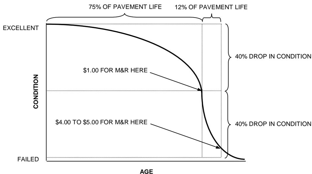
Figure 1. Pavement Condition versus Cost of Repair.
