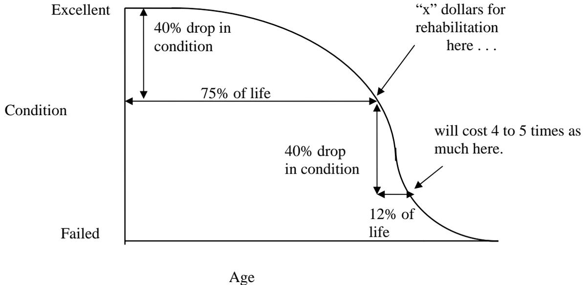
Figure 1. Pavement condition versus cost of repair.
