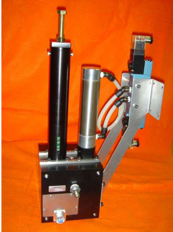
Figure 3. Single Sealant Applicator
