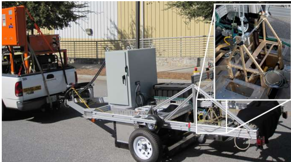
Figure 2. Prototype Crack Sealing Hardware with Detail of Applicators
