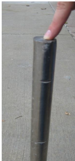
Figure 4.2.1.2 – Dowel bar for bearing systems
