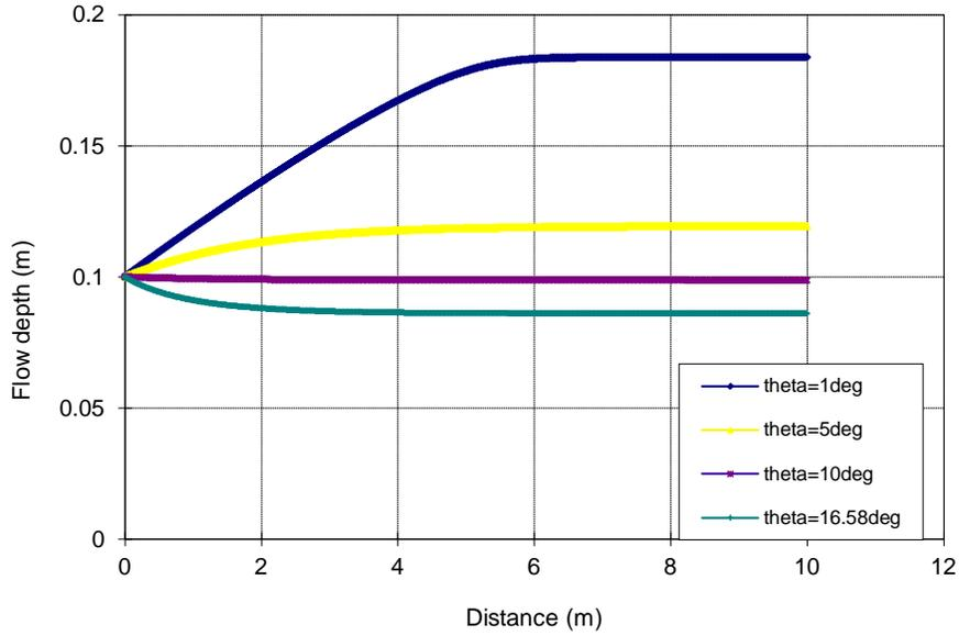
**Figure 6. The influence of slope gradient on flow depth.**
