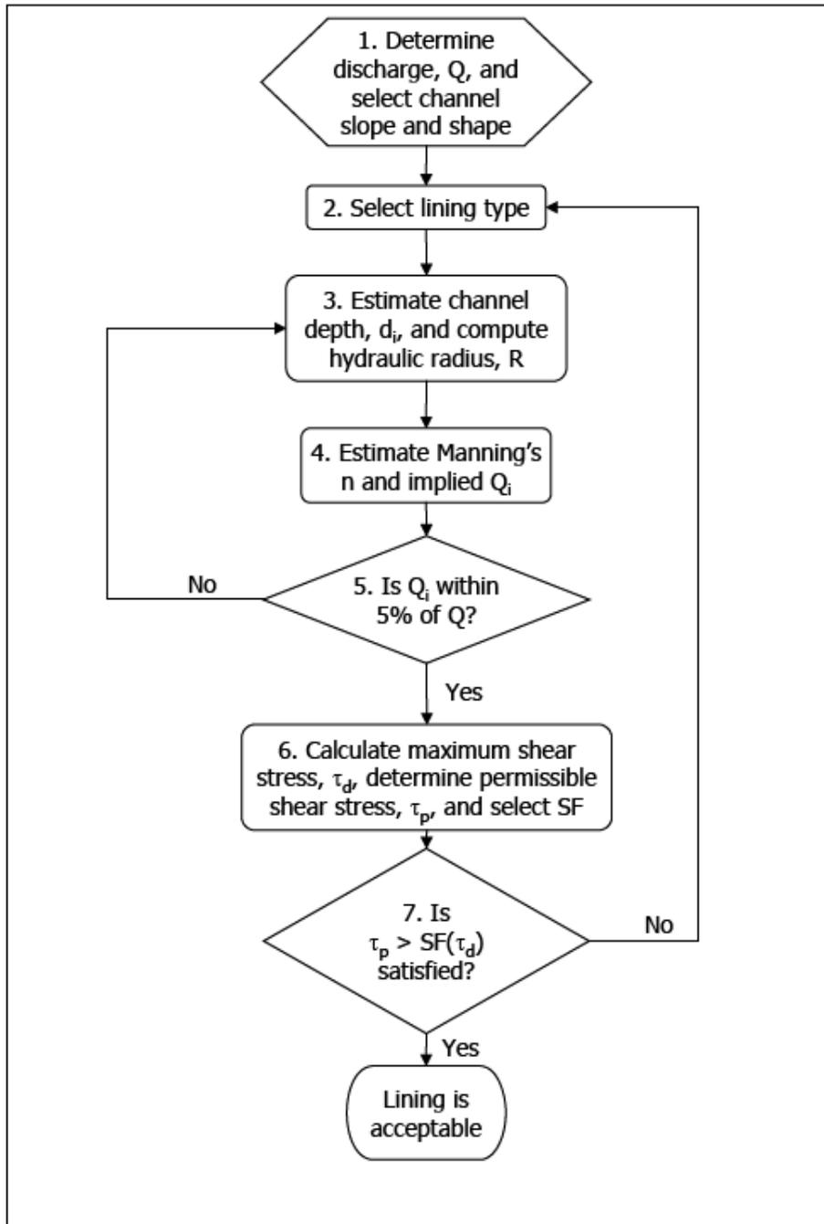
Figure 3.1. Flexible Channel Lining Design Flow Chart
