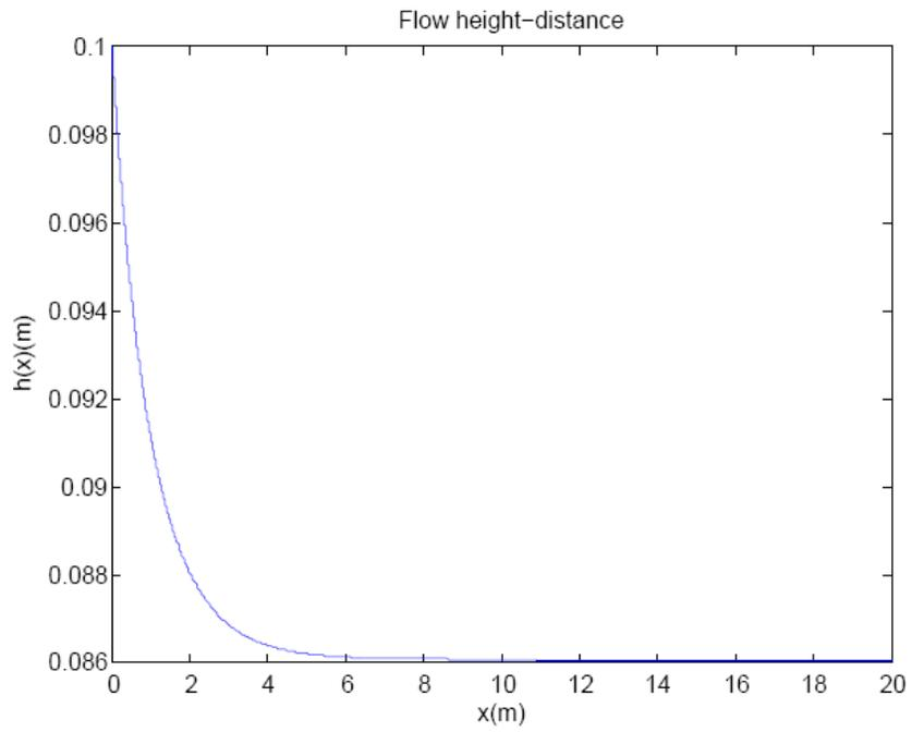
**Figure 4. Flow depth-distance (along the slope).**
