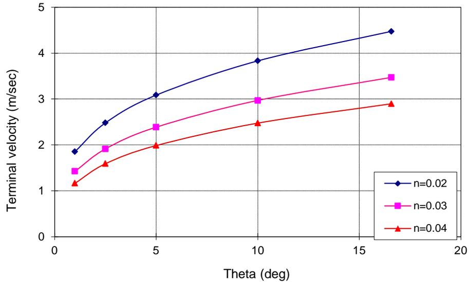
**Figure 9. Terminal velocity as a function of slope and roughness.**
