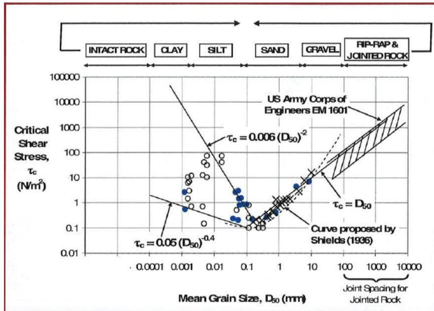
**Figure 12. Critical shear stress as a function of mean grain size (Briaud, 2008).**
