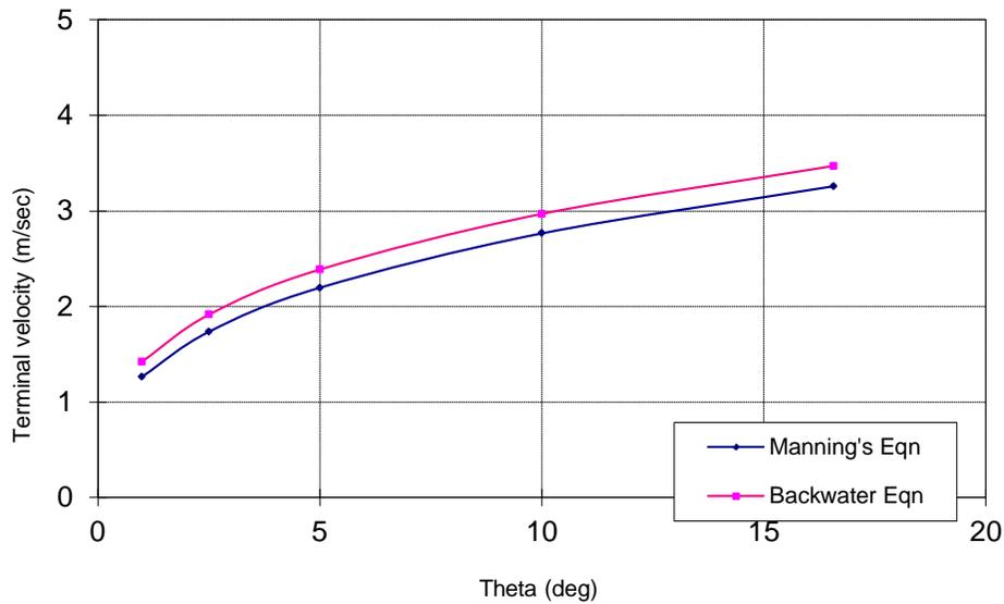
**Figure 8. Comparison between Manning's equation and the backwater equation.**
