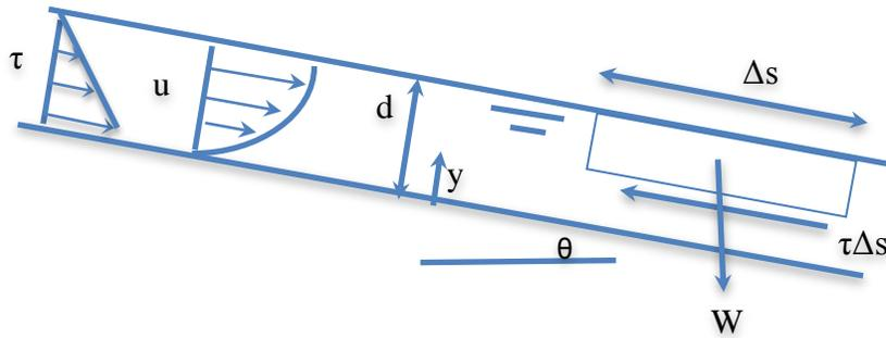
**Figure 1. Velocity gradient in open, laminar channel flow (cross-sectional view).**
