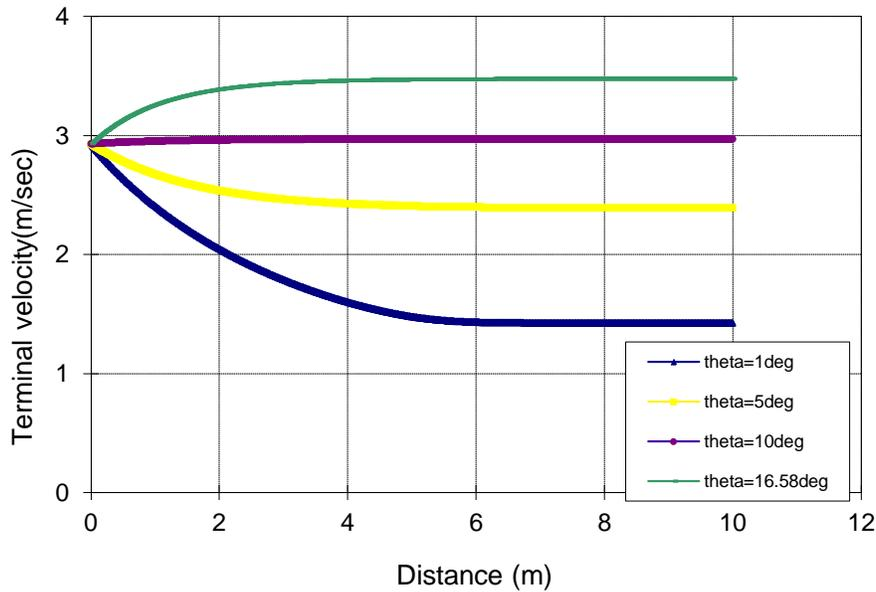
**Figure 7. The influence of slope gradient on terminal velocity.**
