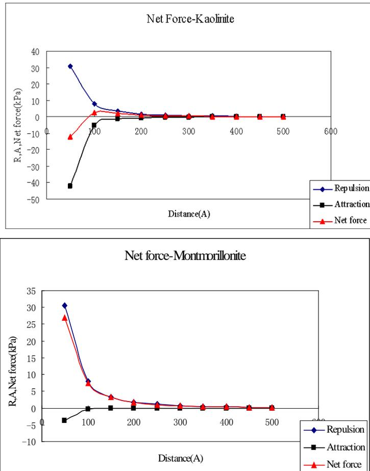
**Figure 13. Net force as a function of clay particle separation.**
