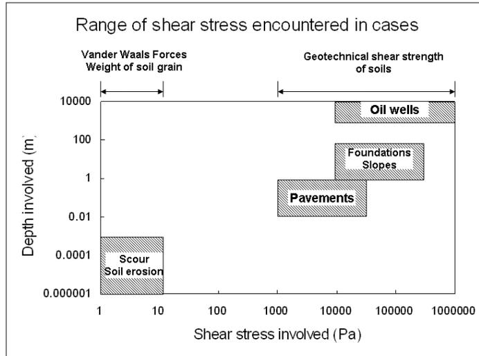
**Figure 3. Magnitude of shear stress in erosion problems (Briaud, 2008).**
